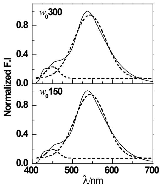
**Figure S1.** Deconvolution of emission spectra (bold line) of C153 in lower aqueous layer of ternary solutions ( $w_0 = 300$  and 150) into two gaussian (dashed line) functions. The emission spectra are recorded at  $\lambda_{\text{ex}} = 402$  nm.
