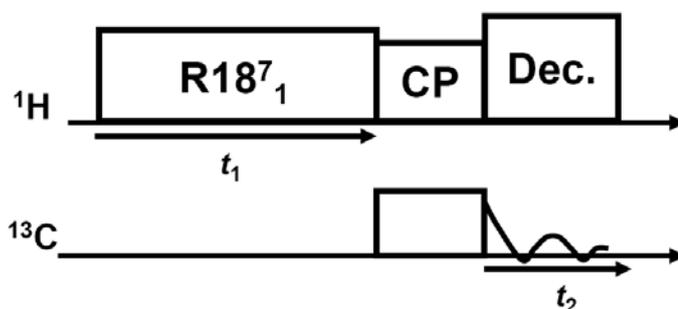
Fig. S1a. Proton Detected (encoded) Local Field spectroscopy with R-type recoupling (R-PDLF).<sup>1</sup> Proton magnetization evolves during the time period  $t_1$  under the effect of the heteronuclear recoupling sequence  $R18^7$ .<sup>2</sup> This magnetization, modulated by the  $^1\text{H}$ - $^{13}\text{C}$  dipolar interaction, is transferred via cross polarization (CP) to the  $^{13}\text{C}$  spins for detection during  $t_2$  in the presence of the heteronuclear proton decoupling.
