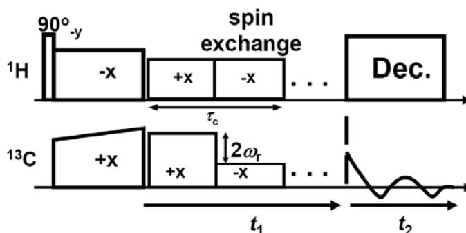
Fig. S1b. Amplitude- and Phase-Modulated Cross-Polarization (APM-CP).<sup>3,4</sup> After the CP signal enhancement, the dipolar evolution period is initiated by inverting the phase of the  $^1\text{H}$  spin-lock field. The CP fields during  $t_1$  period are phase- and amplitude-modulated to achieve the  $^1\text{H}$ - $^{13}\text{C}$  heteronuclear dipolar recoupling. Finally, the  $^{13}\text{C}$  signal is detected in the presence of the heteronuclear  $^1\text{H}$  decoupling.
