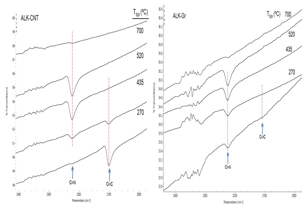
**Figure S7.** FTIR spectra corresponding to amplified region of the spectra in Fig 3 for ALK-G and ALK-MWNT as a function of thermal treatment under nitrogen in the thermobalance.
