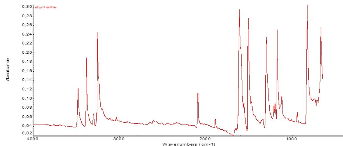
**Figure S6.** FTIR spectrum of 4-ethynylaniline.
