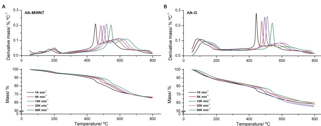
**Figure S5.** TG and dTG traces for the MWNT and Graphene alkyne derivatives tested at 1, 5, 10, 20 and 50 K min<sup>-1</sup> under a N<sub>2</sub> atmosphere
