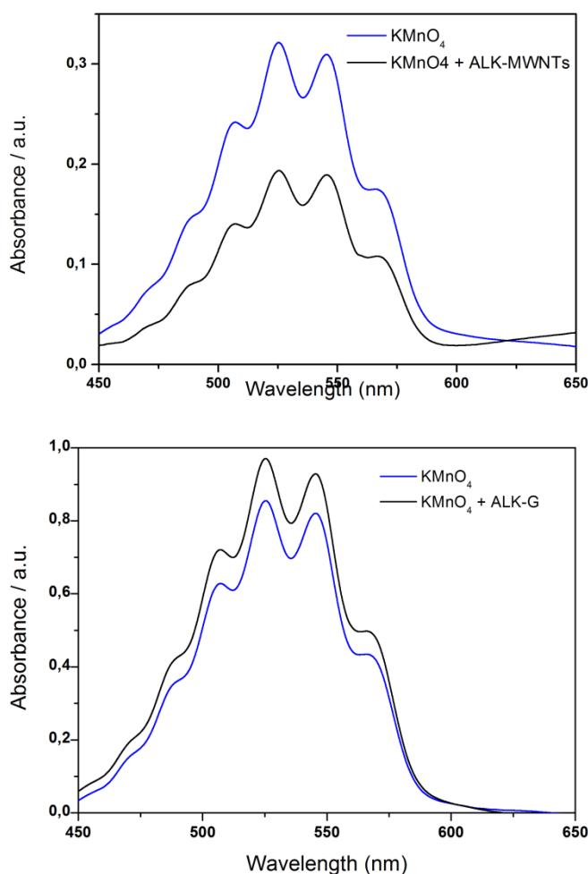
**Figure S3.** UV absorption spectra of  $\text{KMnO}_4$  before and after mixing with ALK-MWNT (top) and ALK-G (bottom).
