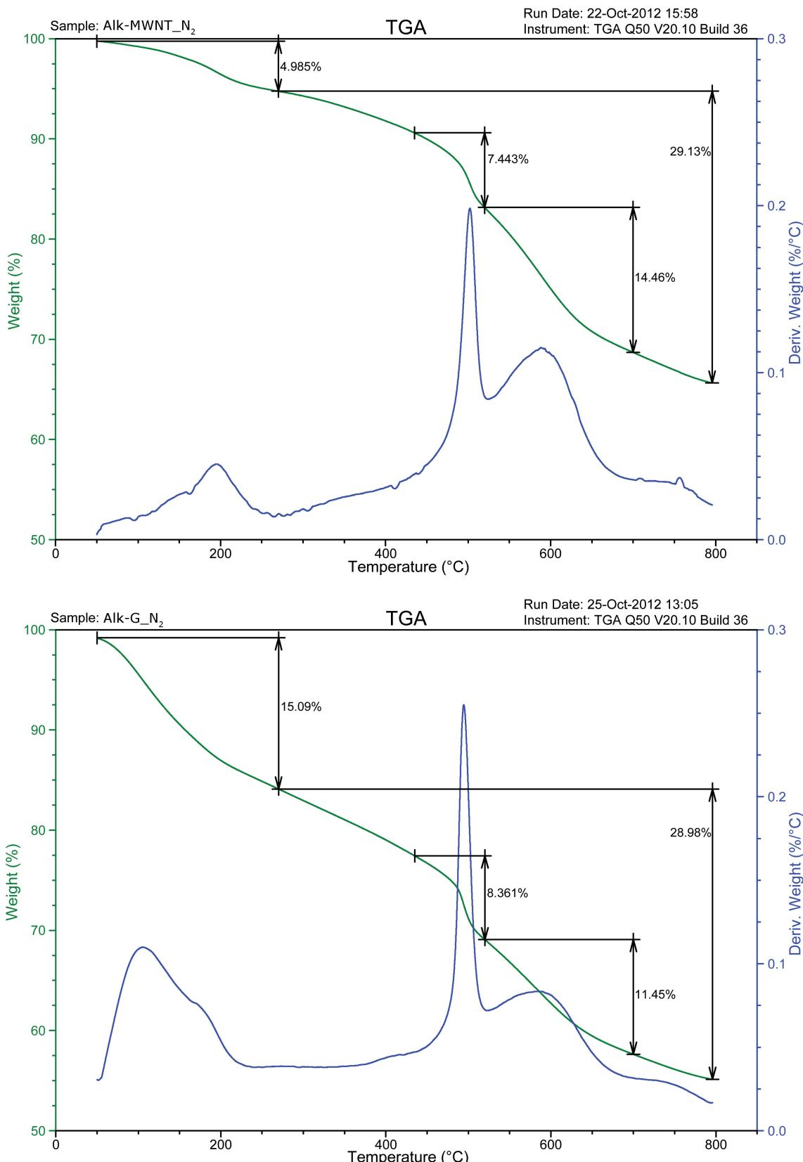
**Figure S2.** TGA and dTGA traces for the MWNTs and Graphene alkyne derivatives tested at 10 °C
