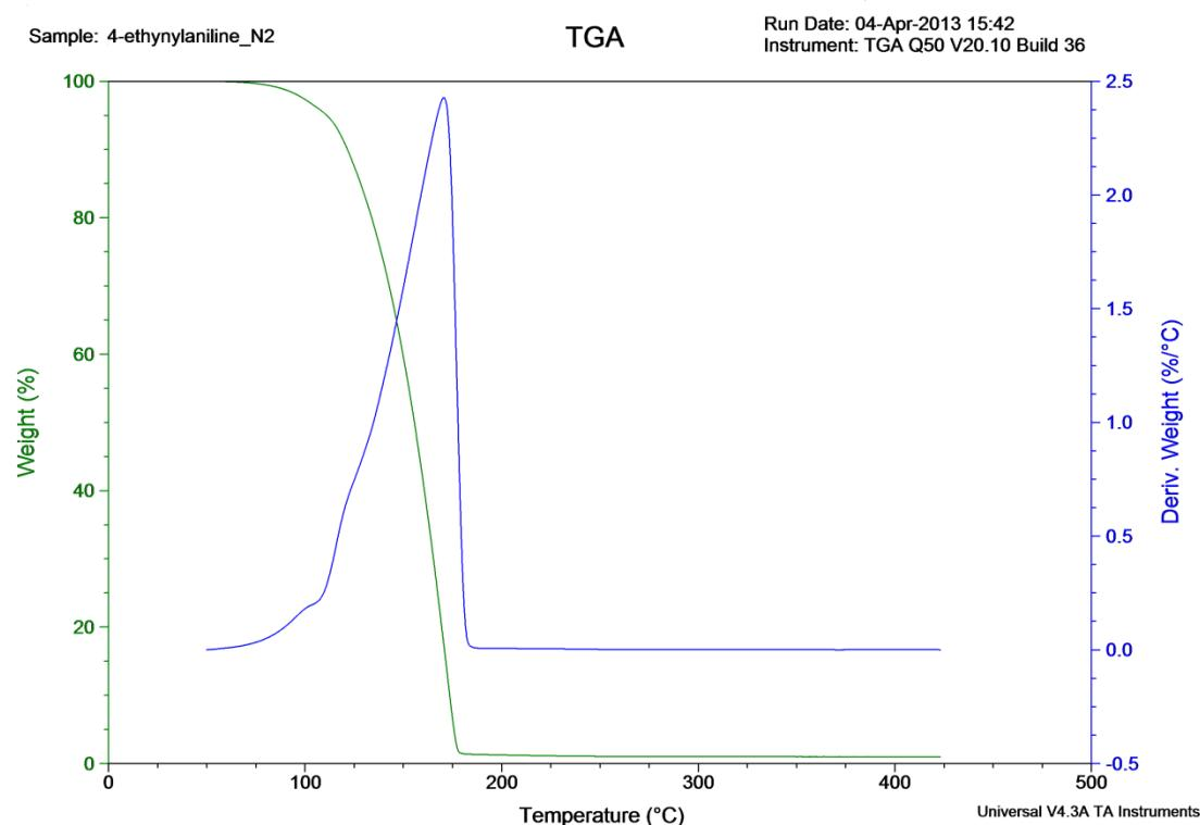
**Figure S4.** TGA and dTGA traces for 4-ethynylaniline tested at  $10\text{ }^{\circ}\text{C min}^{-1}$ ,  $\text{N}_2$
