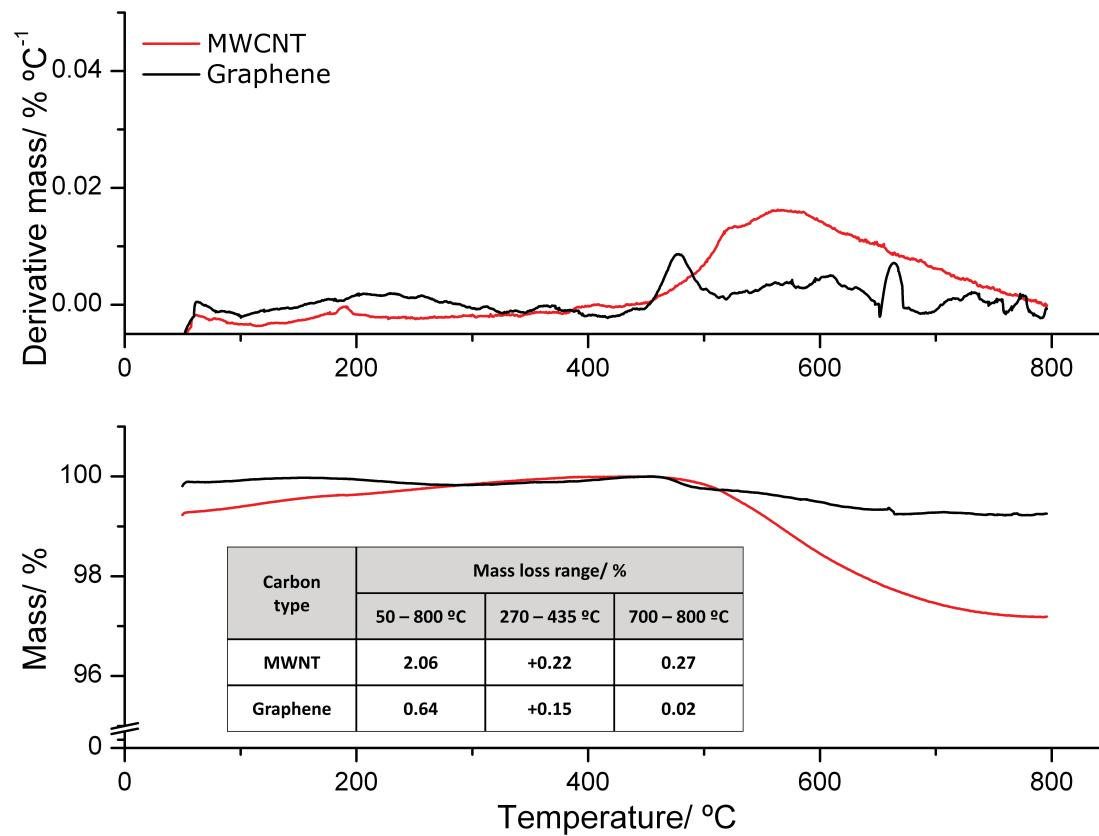
**Figure S1.** TGA traces of the unmodified MWNTs and Graphene samples tested at  $10\text{ }^{\circ}\text{C min}^{-1}$ ,  $\text{N}_2$ .
