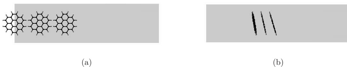
FIG. 5: (a) Starting configuration with 3 molecules aligned parallel to the tube axis in a tube with D = 1.5 \text{ nm} and (b) a snapshot of a configuration resulting from equilibrating the configuration shown in a) for T = 300 \text{ K} .
