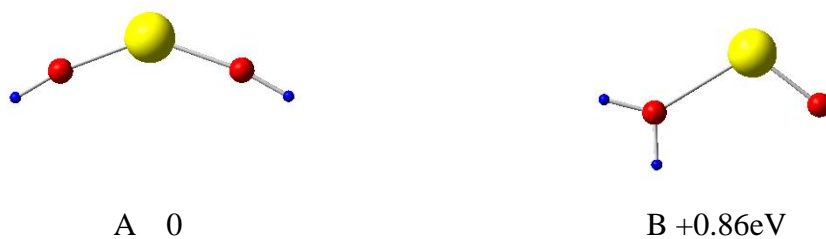
Figure S1 Optimized geometries of the typical low-lying isomers of \text{TiO}(\text{H}_2\text{O})^+ cluster obtained at B3LPY/6-311G+(d, p) level. The relative energy to the most stable isomer is shown. The yellow, red and blue spheres stand for Ti, O and H atoms, respectively.
