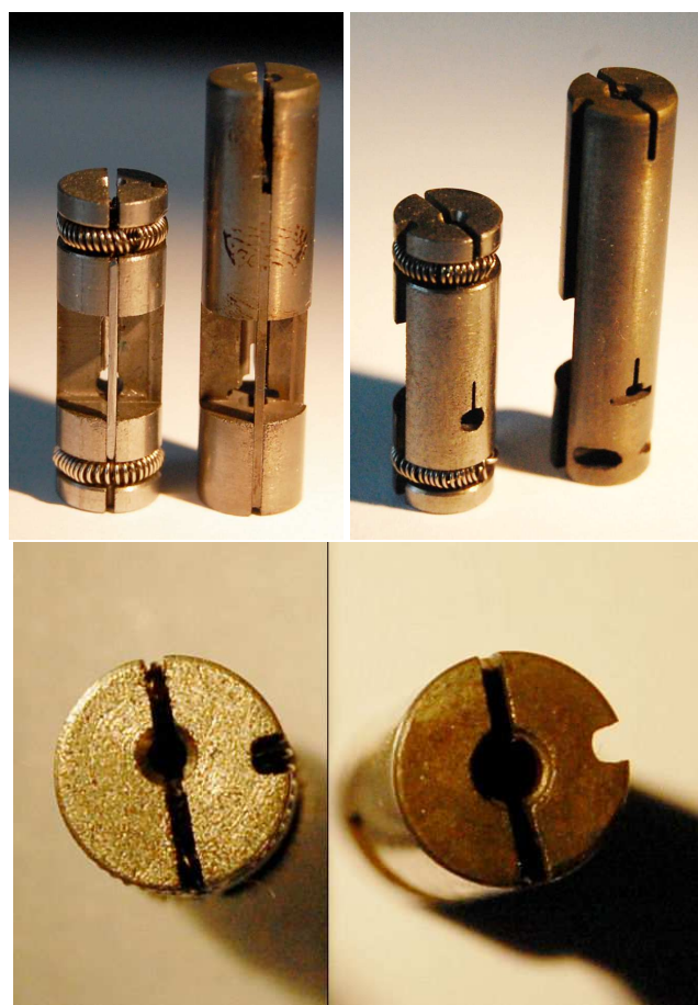
Sup. Fig. 1 Comparison of the MK3BRIM and MK2BRIM. Views from the beam stop blade side (upper left panel), beam entrance slits side (upper right panel), and top (lower panel). The top view shows the sample tube holes, side slot that allows easy flow of the pressure transmitting fluid past the BRIM, and a slot across the top that enables rotation of the BRIM in the pressure vessel bore during initial manual alignment.
