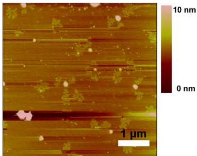
**Fig. S1.** AFM image of our graphene fluoride nanosheets scanned in a large visual field.
