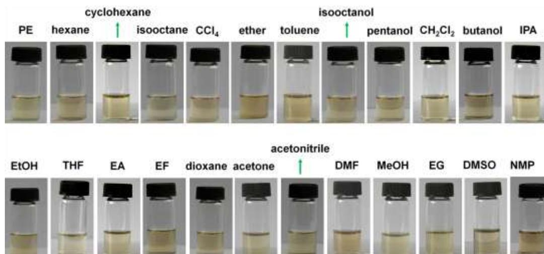
**Fig. S3.** Digital pictures of the fluorographene nanosheets freshly dispersed in other 24 kinds of organic solvents. The dispersions are prepared *via* a volatilization–redispersion process.
