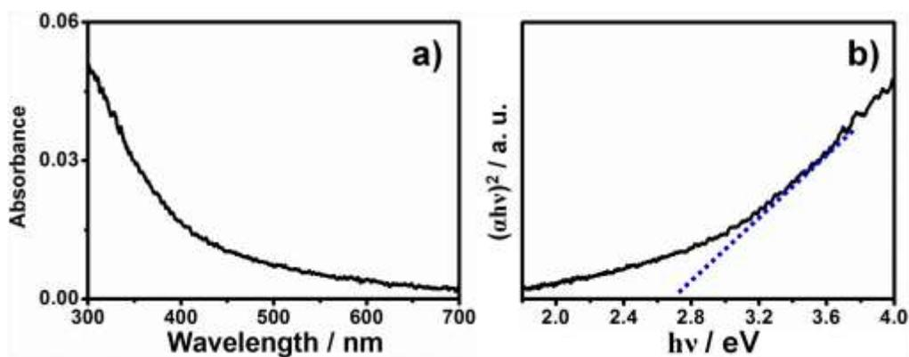
**Fig. S2.** DRS (a) and the corresponding plots of  $(\alpha h\nu)^2$  vs. photon energy (b) of our fluorinated graphene species.
