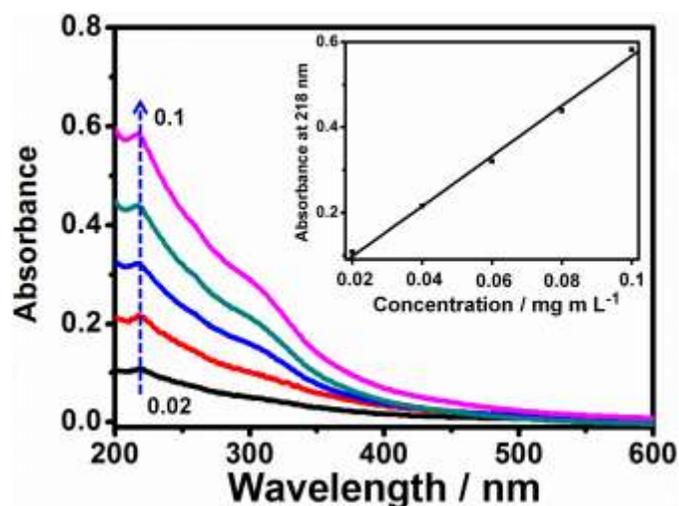
**Fig. S4.** UV-vis spectra of our fluorinated graphene of different concentration dispersed in hexane. Inset: absorbance at 218 nm versus concentration.
