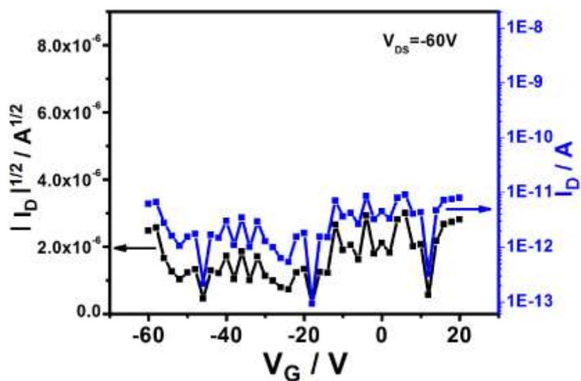
**Fig. S5.** Transfer characteristics of the OFETs using our fluorographene as the active semiconductor layer.
