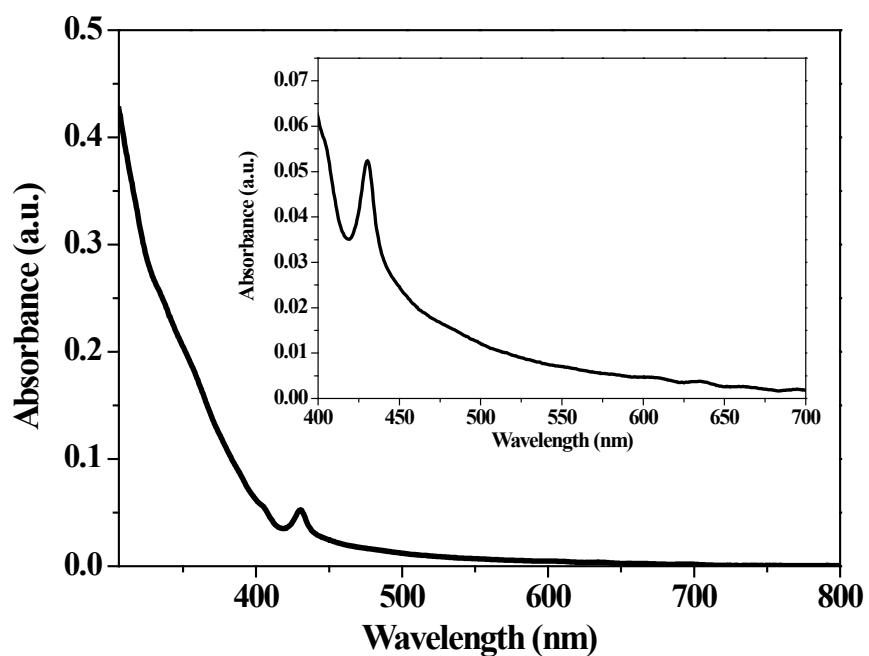
**Figure S5** Absorption spectrum for **1** in  $\text{CHCl}_3$  ( $10^{-5}$  mol/L). Inset: enlarged absorption spectrum in the visible region (400-700nm).
