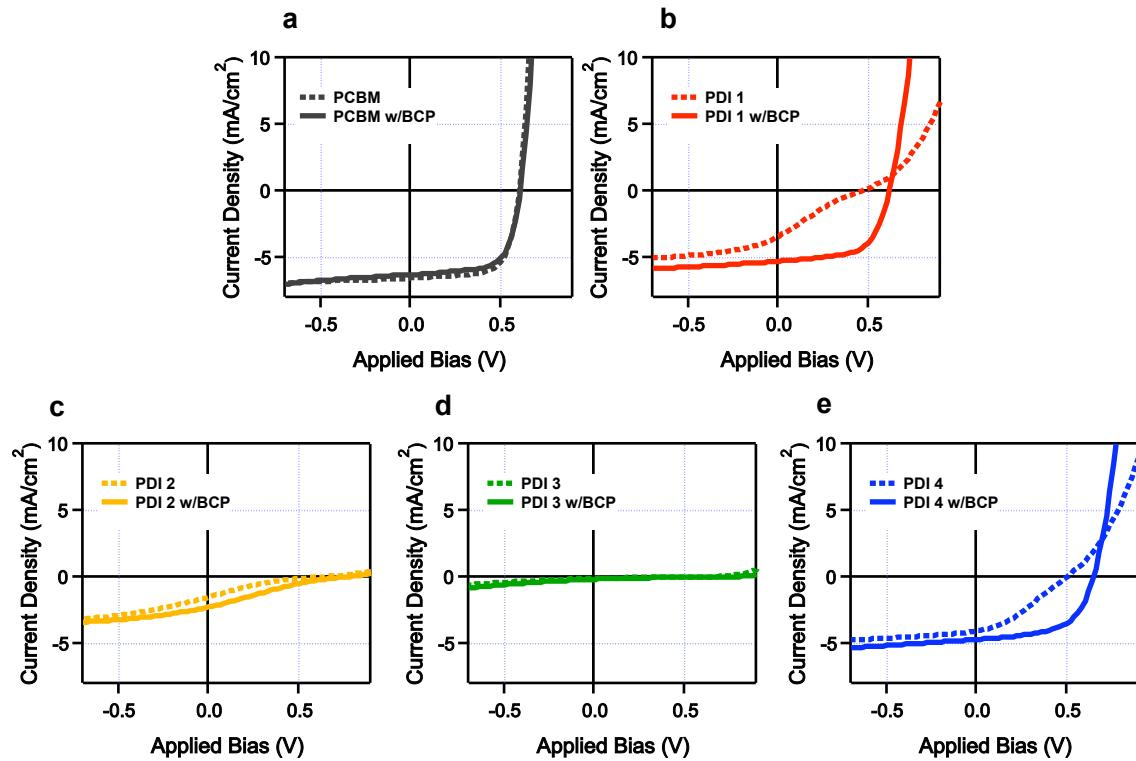
**Figure SI 3. Bilayer OPV device current-voltage ( $J$ - $V$ ) curves under AM1.5 G simulated illumination.** Devices with and without an interfacial bathocuproine (BCP) layer are shown. The device architecture used is ITO/PEDOT:PSS/BP/acceptor/with or without BCP/Al.
