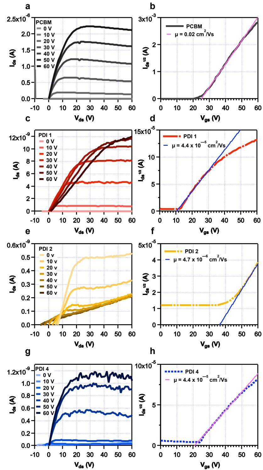
**Figure SI 4.** FET measurements of PDIs. Output characteristics (a, c, e, g) and transfer characteristics in the saturation regime (b, d, f, h) are shown.
