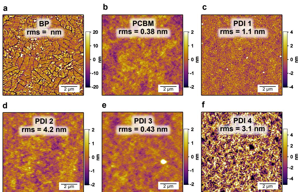
**Figure SI 5.** Tapping mode AFM height images of neat films of the materials used in this study on ITO/PEDOT:PSS substrates. Root mean square (RMS) values are shown below the material name. Images are  $10 \times 10 \mu\text{m}$ .
