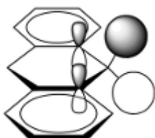
Figure S5 Schematic representation of the coupling between the s orbitals from the \text{CH}_2 group in AH and the p_z orbitals in the phenyl rings, that resembles the coupling of p_z orbitals in cross-conjugated structures.
