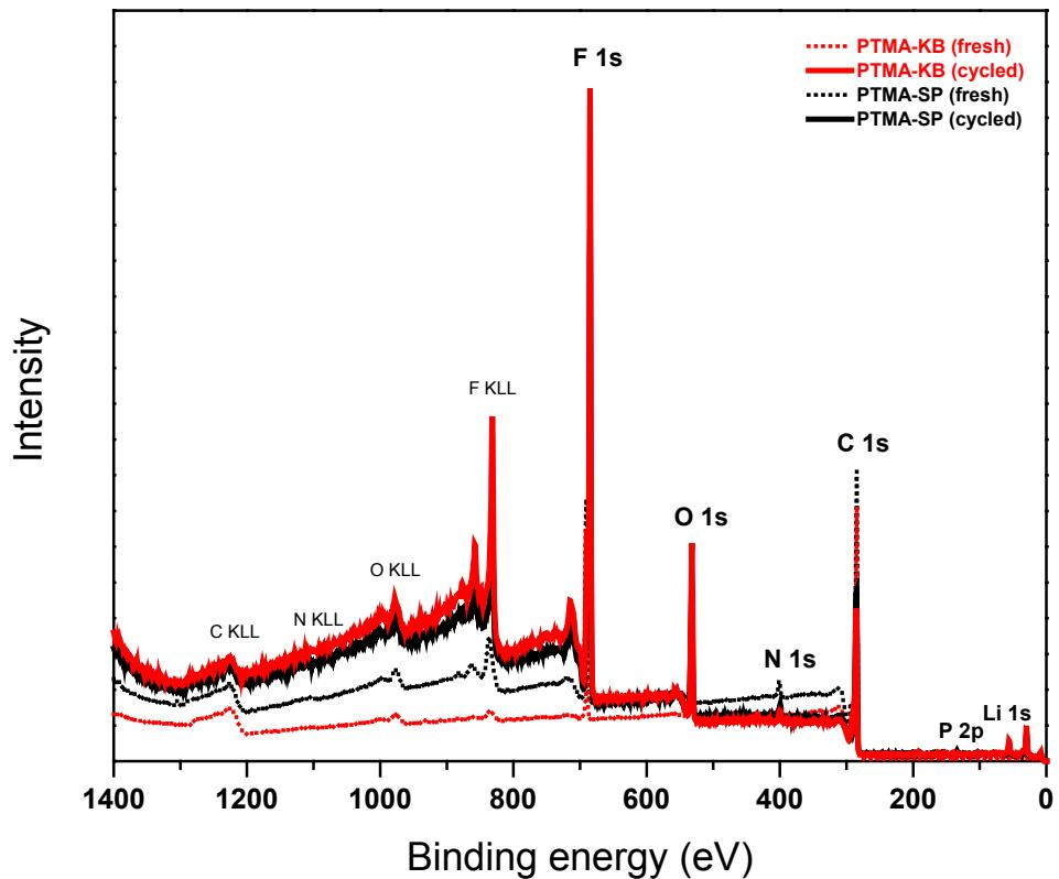
Fig. S1. XPS survey scans for PTMA electrodes before and after 100 cycles.
