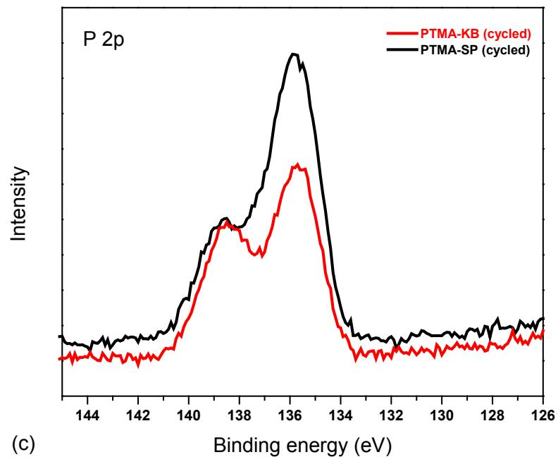
Fig. S2. High-resolution XPS spectra for the binding energy of (a) O 1s, (b) Li 1s, and (c) P 2p for PTMA electrodes before and after 100 cycles.
