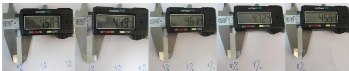
**Fig. S7** Thickness of ZnO QDs/epoxy nanocomposites with different ZnO<sub>KH560</sub> contents.
