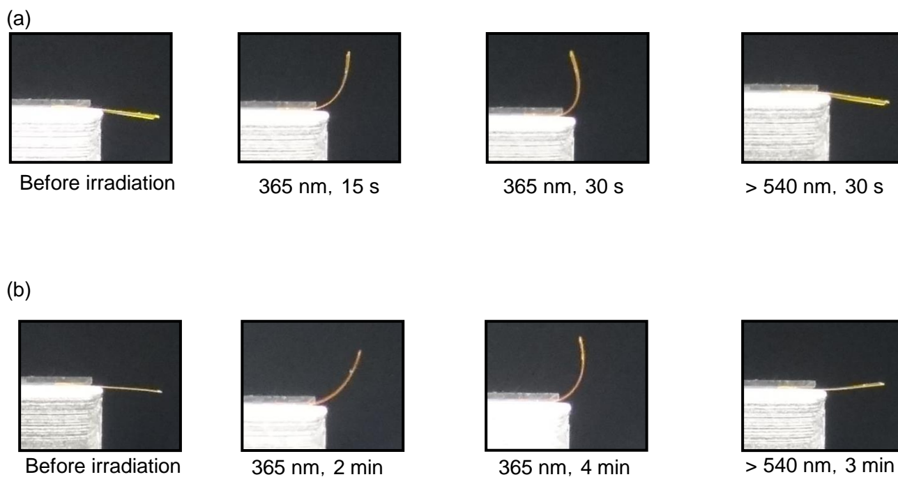
Fig.S1 Pictures of the film bending by irradiation of a UV light at the wavelength of 365 nm at (a) 65 °C, and (b) 30 °C, and the returning back to the original position by irradiation of a visible light (>540 nm). The film size was 10 mm×3 mm×16 μm. The light intensities of the UV and the visible lights were 10 and 40 mW/cm 2 .
