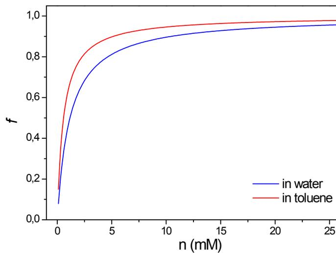
**Fig. S2** Peak-to-trough intensity power dependence of the low field EPR line (the derivative of Lorentzian line) for TEMPONE-D-<sup>15</sup>N in toluene at different concentrations. The solid lines represent fitting curves with (C. P. Poole, *Electron Spin Resonance*, John Wiley & Sons, New York, 1983):
