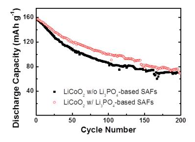
**Fig. S3** Cycling stability of LiCoO<sub>2</sub> specimens with and without Li<sub>3</sub>PO<sub>4</sub>-based SAFs that were cycled between 3 V and 4.5 V (*vs.* Li/Li<sup>+</sup>) at the charge/discharge rate of 1C at room temperature. The capacity fading is appreciably lower in the specimen with ~ 2.5 nm thick SAFs. It is possible that the SAFs disintegrated after ~140 cycles due to the strain accumulation resulted from cycling at the extended voltage range of 3 V to 4.5 V.
