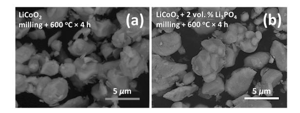
**Fig. S2** Representative SEM images of the **(a)**  $LiCoO_2$  and **(b)**  $LiCoO_2 + 2$  vol. %  $Li_3PO_4$  specimens that were milled and subsequently annealed at 600 °C for 4 h.
