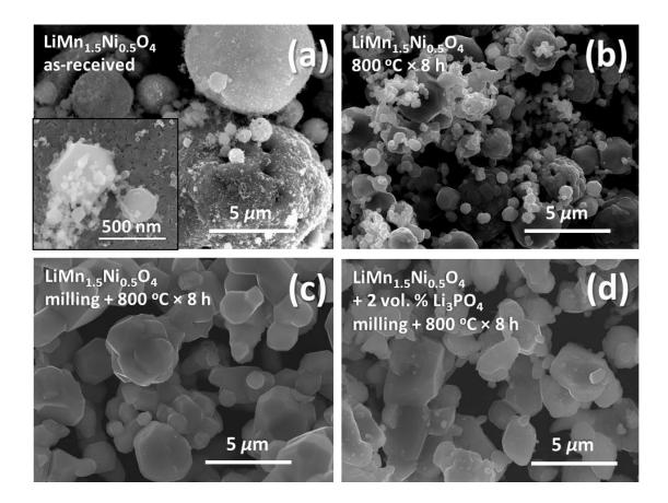
**Fig. S5** Representative SEM images of **(a)** the as-received  $LiMn_{1.5}Ni_{0.5}O_4$  specimen and **(b)** the reference  $LiMn_{1.5}Ni_{0.5}O_4$  specimen annealed at 800 °C (without ball milling), as well as the **(c)**  $LiMn_{1.5}Ni_{0.5}O_4$  and **(d)**  $LiMn_{1.5}Ni_{0.5}O_4 + 2$  vol. %  $Li_3PO_4$  specimens that were milled and subsequently annealed at 800 °C for 8 h.
