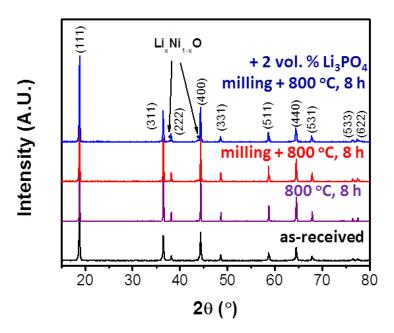
**Fig. S4** XRD patterns of various  $LiMn_{1.5}Ni_{0.5}O_4$  specimens. Minor amounts of a secondary crystalline phase of  $Li_xNi_{1-x}O$  were detected in the milled and annealed specimens.
