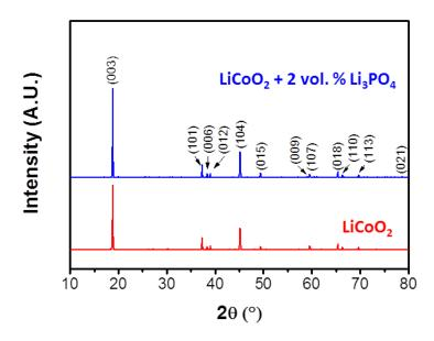
**Fig. S1** XRD patterns of the  $LiCoO_2$  and  $LiCoO_2 + 2$  vol. %  $Li_3PO_4$  specimens that were milled and subsequently annealed at 600 °C for 4 h.
