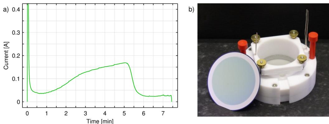
**Fig. S2** Current trace obtained from the on-chip aluminum oxidation (Figure S1d) of a structured wafer (a). The initial peak current, which is limited to 1.8 A, is not depicted completely. For the process a home-built Teflon holder is used (b). It is shown here with an unstructured anodized 4"-wafer.
