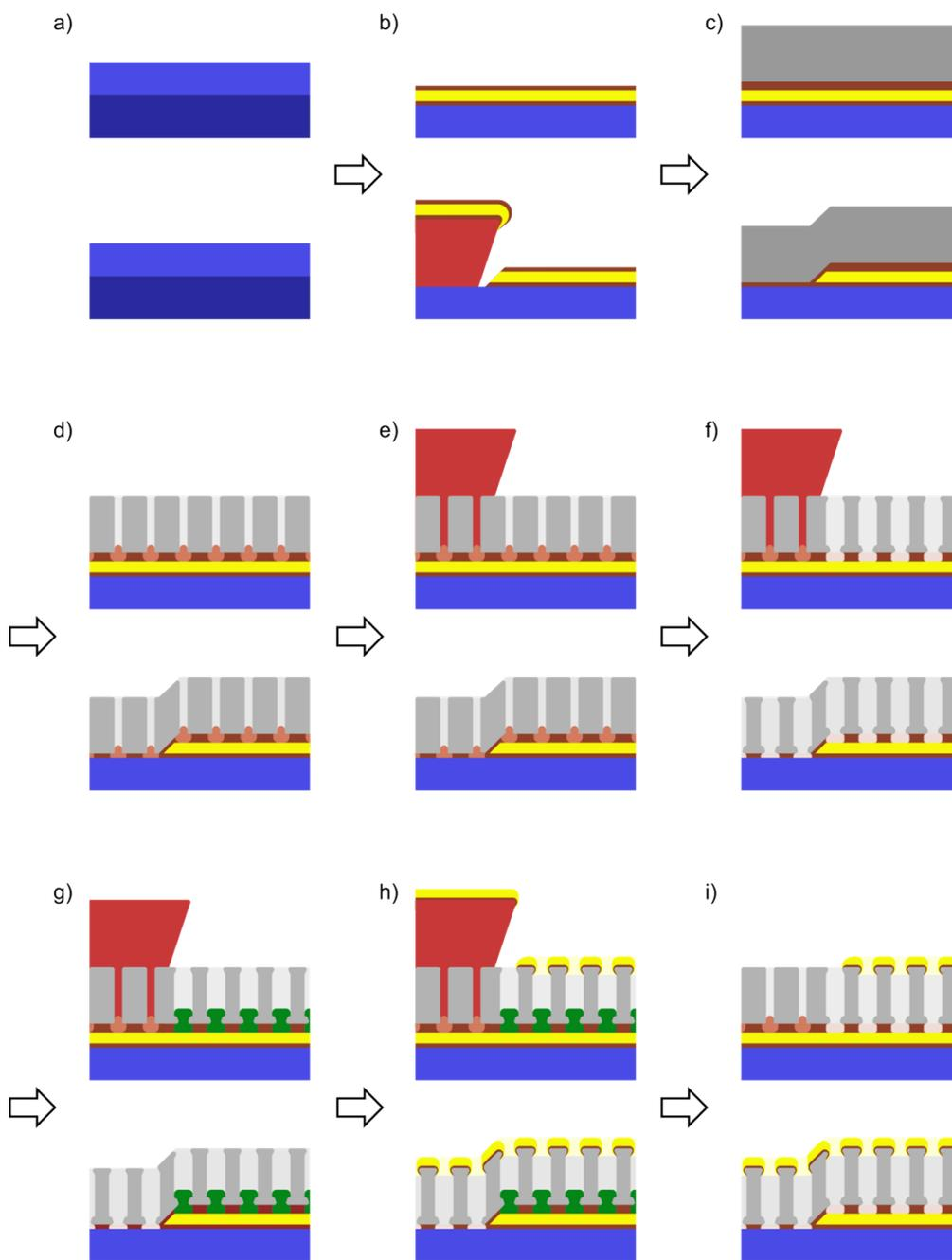
**Fig. S1** Fabrication steps of the nanoporous alumina sensor at the boundary areas of the crossing electrodes. Upper and lower sketches show the edge of the top and the edge of the bottom electrode, respectively.
