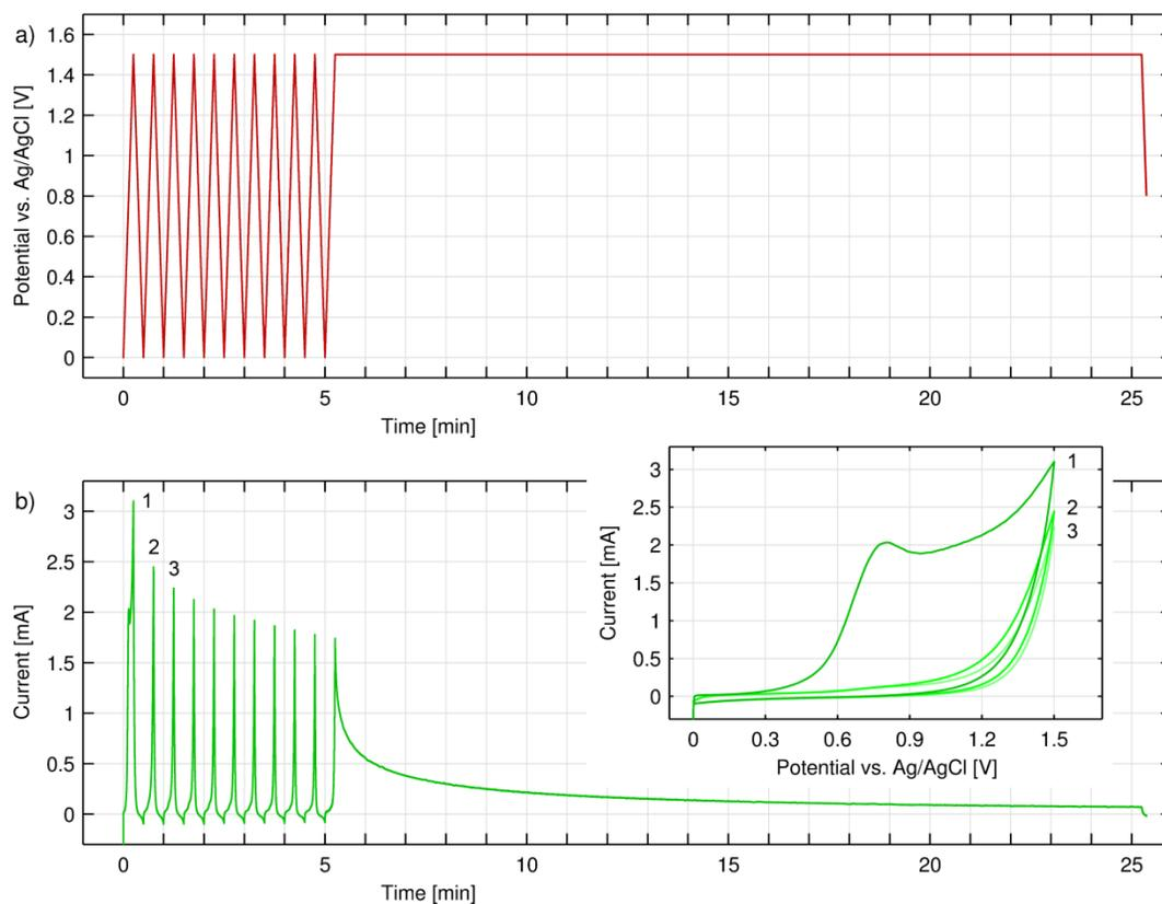
**Fig. S3** Potential (a) and current (b) trace of the pyrrole deposition step (Figure S1g). In the inlay the currents of first three sweeps (1-3) are plotted versus the applied potential.
