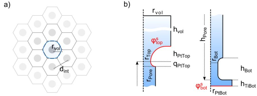
**Fig. S4** Approximation of the nanoporous sensor by single identical domains (a) as well as the assumed radial symmetric geometry of a single pore and the adjacent reservoir (b).
