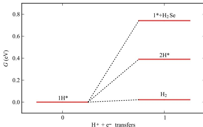
Figure S2: Free energy diagram for  $\text{H}_2$  evolution, H adsorption, and  $\text{H}_2\text{Se}$  evolution on the Mo-edge of  $\text{MoSe}_2$  with  $\theta_{\text{Se}} = 0.5$  ML and  $\theta_{\text{H}} = 0.25$  ML. Here,  $\text{H}^*$  denotes an adsorbed hydrogen, and  $*$  denotes a selenide vacancy.
