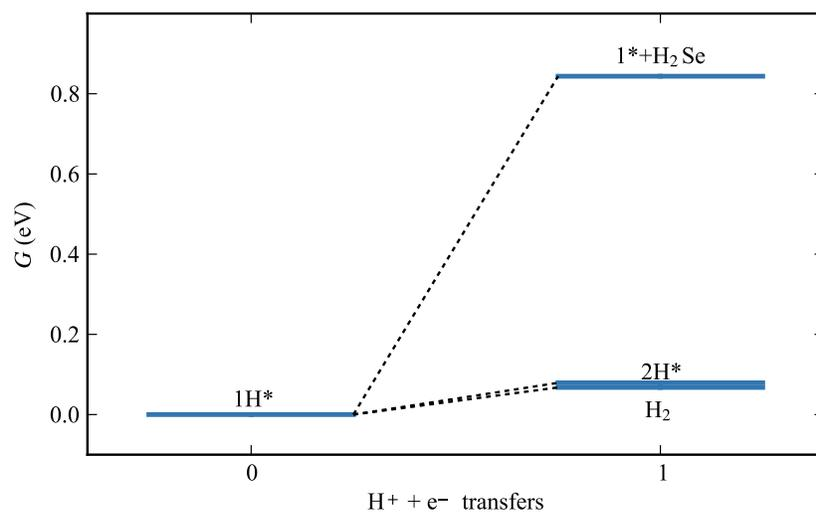
Figure S3: Free energy diagram for  $\text{H}_2$  evolution, H adsorption, and  $\text{H}_2\text{Se}$  evolution on the Mo-edge of  $\text{MoSe}_2$  with  $\theta_{\text{Se}} = 0.75$  ML and  $\theta_{\text{H}} = 0.25$  ML. Here,  $\text{H}^*$  denotes an adsorbed hydrogen, and  $*$  denotes a selenide vacancy.
