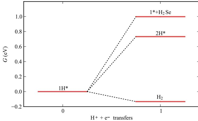
Figure S7: Free energy diagram for  $\text{H}_2$  evolution, H adsorption, and  $\text{H}_2\text{Se}$  evolution on the W-edge of  $\text{WSe}_2$  with  $\theta_{\text{Se}} = 0.5$  ML and  $\theta_{\text{H}} = 0.25$  ML. Here,  $\text{H}^*$  denotes an adsorbed hydrogen, and  $*$  denotes a selenide vacancy.
