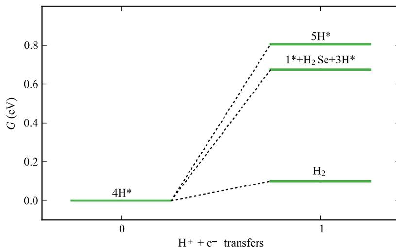
Figure S5: Free energy diagram for  $\text{H}_2$  evolution, H adsorption, and  $\text{H}_2\text{Se}$  evolution on the Se-edge of  $\text{MoSe}_2$  with  $\theta_{\text{Se}} = 1.0$  ML and  $\theta_{\text{H}} = 1.0$  ML. Here,  $\text{H}^*$  denotes an adsorbed hydrogen, and  $*$  denotes a selenide vacancy.
