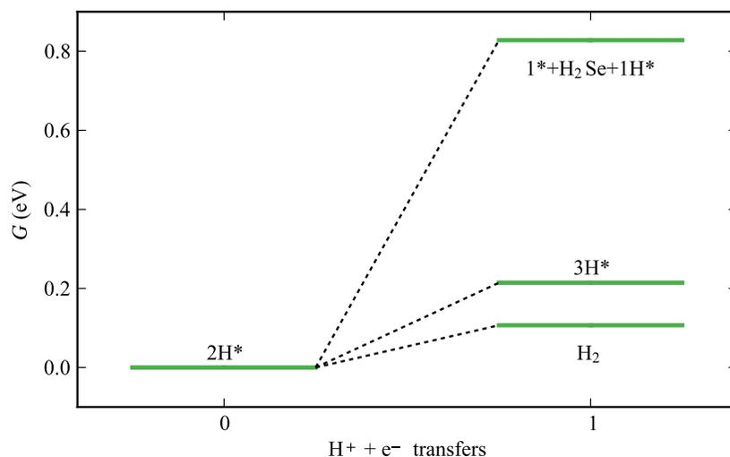
Figure S9: Free energy diagram for  $\text{H}_2$  evolution, H adsorption, and  $\text{H}_2\text{Se}$  evolution on the Se-edge of  $\text{WSe}_2$  with  $\theta_{\text{Se}} = 1.0$  ML and  $\theta_{\text{H}} = 0.50$  ML. Here,  $\text{H}^*$  denotes an adsorbed hydrogen, and  $^*$  denotes a selenide vacancy.
