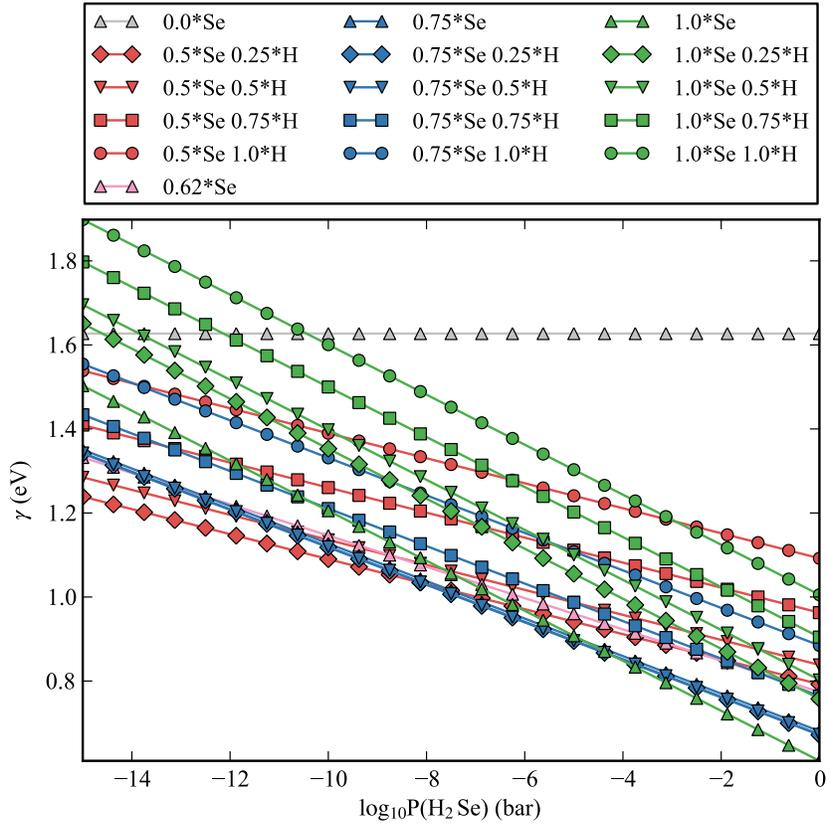
Figure S1: Plot of  $\gamma$  vs.  $\log_{10}P(\text{H}_2\text{Se})$  for the Mo-edge of MoSe<sub>2</sub>.
