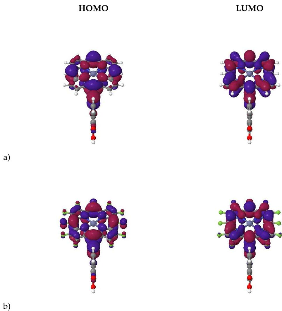
Figure S10: Comparison of the spatial shape of the HOMO and LUMO of dyes using only the H side group and the EthynPhA anchor group together with the ZnP (top) and FZnP (bottom) backbones.
