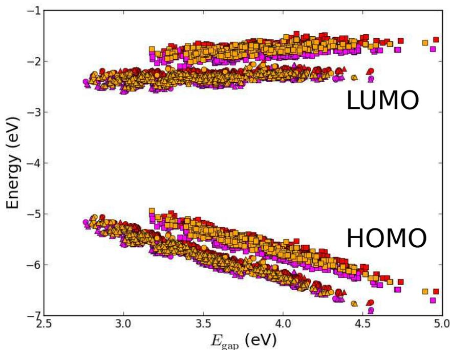
Figure S1: Calculated  $E_{\text{HOMO}}$  and  $E_{\text{LUMO}}$  relative to vacuum ordered by the resulting  $E_{\text{gap}}$  of functionalized porphyrins with the ZnP (red), H<sub>2</sub>P (orange) and TiOP (magenta) backbones and the EthynPhA (square), 2CarboxyPropenA (circle) and 2CyanoPropenA (triangle) anchor groups.
