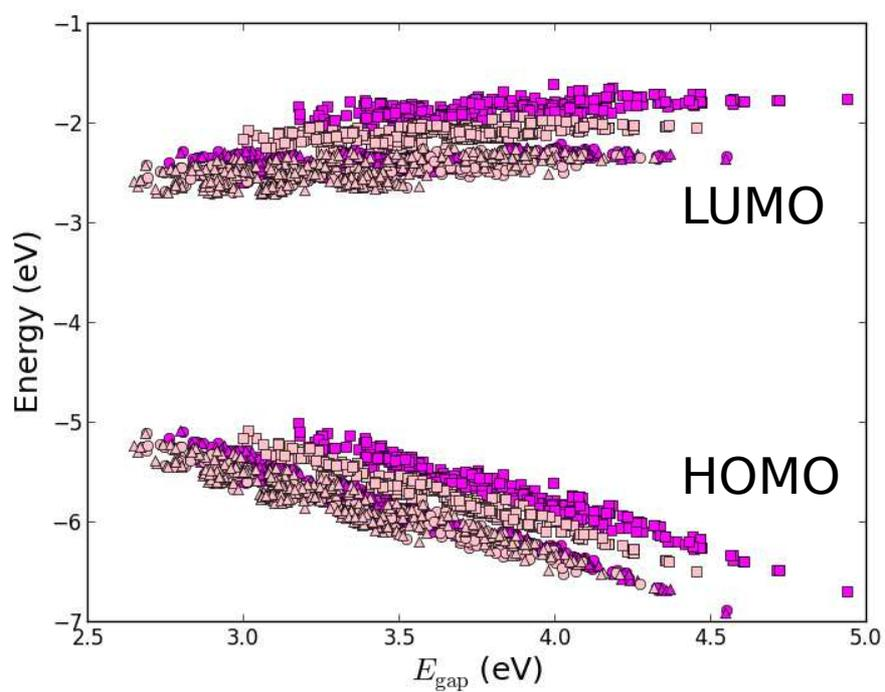
Figure S5: Calculated  $E_{\text{HOMO}}$  and  $E_{\text{LUMO}}$  relative to vacuum ordered by the resulting  $E_{\text{gap}}$  of functionalized porphyrins with the TiOP (magenta) and TiO<sub>2</sub>BAP (pink) backbones and the EthynPhA (square), 2CarboxyPropenA (circle) and 2CyanoPropenA (triangle) anchor groups.
