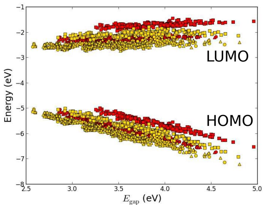
Figure S9: Calculated  $E_{\text{HOMO}}$  and  $E_{\text{LUMO}}$  relative to vacuum ordered by the resulting  $E_{\text{gap}}$  of functionalized porphyrins with the ZnP (red) and FZnP (yellow) backbones and the EthynPhA (square), 2CarboxyPropenA (circle) and 2CyanoPropenA (triangle) anchor groups.
