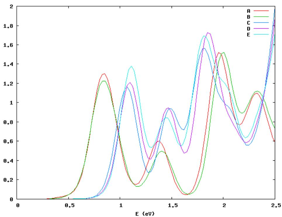
Figure S13: TD-DFT spectra with an added width of 0.1 eV of the top five candidates. With a sufficiently amount of dye layers, all dyes will have a step-function absorption spectrum above the absorption edge since the absorption here is non-zero for all dyes. However, the absorption edge is poorly predicted by TD-DFT due to the charge-transfer character of Donor- $\pi$ -Acceptor porphyrin dyes.
