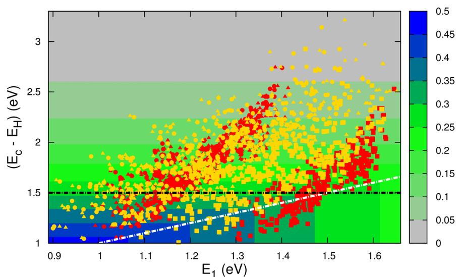
Figure S12: Calculated level alignment quality as function of the optical gap,  $E_1$ , and the energy difference between the conduction band for functionalized porphyrins with the ZnP (red) and FZnP (yellow) backbones and the EthynPhA (square), 2CarboxyPropenA (circle) and 2CyanoPropenA (triangle) anchor groups. The black dotted line indicates the lower limit of  $E_c - E_H$  for dyes to be used with the  $I^-/I_3^-$  electrolyte and the white dotted line indicates where  $E_c - E_H = E_1$ .
