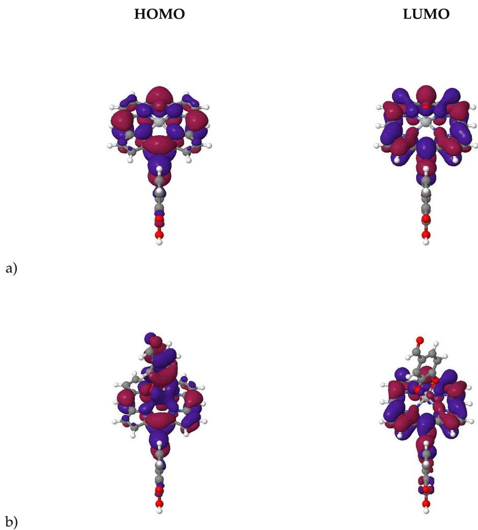
Figure S6: Comparison of the spatial shape of the HOMO and LUMO of dyes using only the H side group and the EthynPhA anchor group together with the TiOP (top) and TiO<sub>2</sub>BAP (bottom) backbones.
