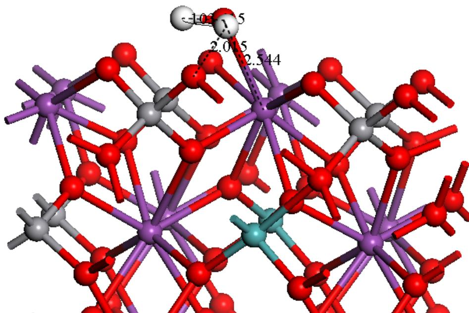
Fig. S6. The geometric structure of H<sub>2</sub>O adsorbed on Mo@Bi<sub>2</sub>S<sub>3</sub> surface.
