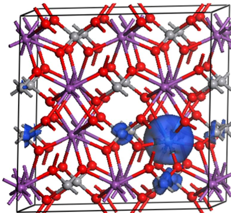
Fig. S4. The geometric structure of H<sub>2</sub>O adsorbed on Mo@V\_top surface.
