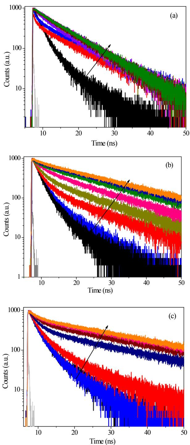
**Figure S5.** Time resolved emission decays of EPT in buffer with increasing concentration of (a) SDS (0 mM to 50 mM) (b) Triton-X (0 mM to 10 mM) and (c) CTAB (0 mM to 10 mM) collected at 530 nm ( $\lambda_{\text{ex}} = 375$  nm).
