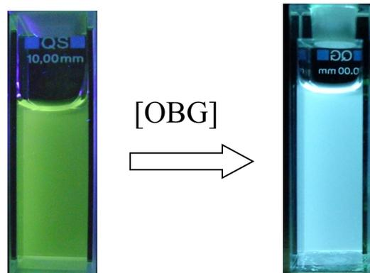
**Figure S1.** Fluorescence switch of EPT in presence of OBG micelles ( $\lambda_{\text{ex}} = 360 \text{ nm}$ ).
