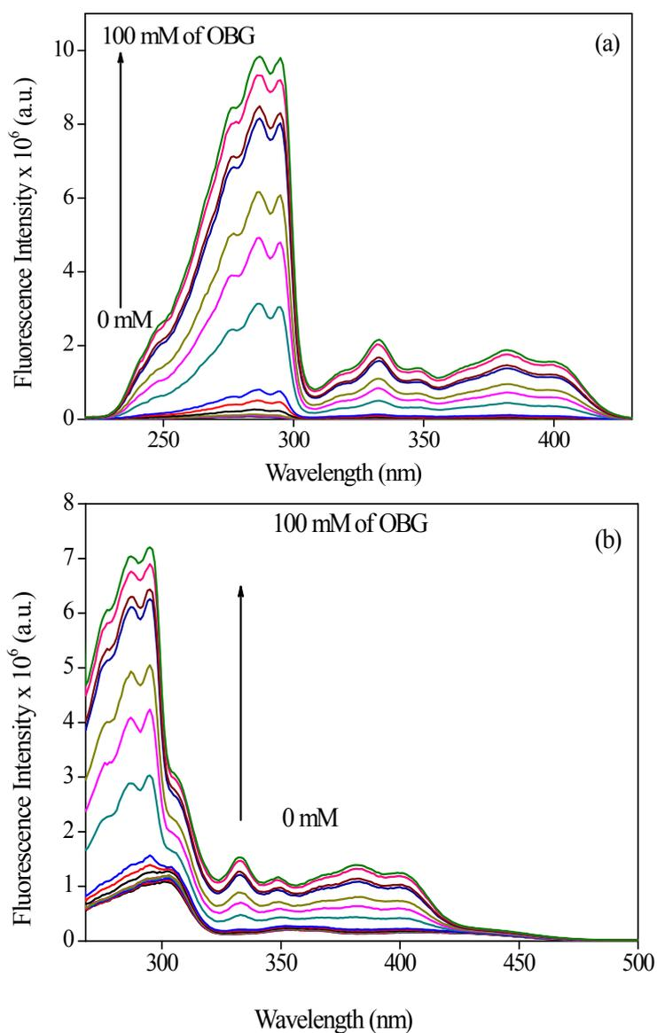
**Figure S2.** Excitation spectra of EPT in buffer with increasing concentration of OBG (0 mM to 100 mM) collected at 440 nm (a) and 530 nm (b).
