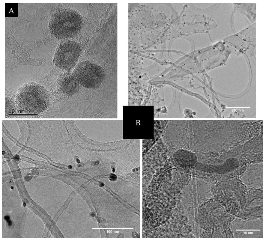
Figure S6. TEM micrographs of  $\text{Fe}_3\text{O}_4/\text{FLG}$  catalyst reduced at  $400^\circ\text{C}$  with spherical shape of particles (A) and CNTs grown on this catalyst during ethane decomposition at  $800^\circ\text{C}$ .
