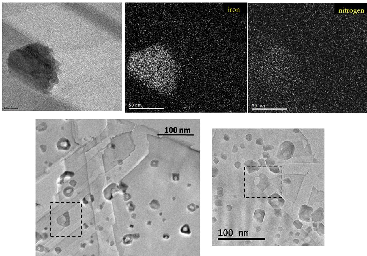
Figure S4. TEM and TEM/EELS analysis micrographs showing a displacement of faceted  $\text{FeN}_x$  core during etching of graphene.
