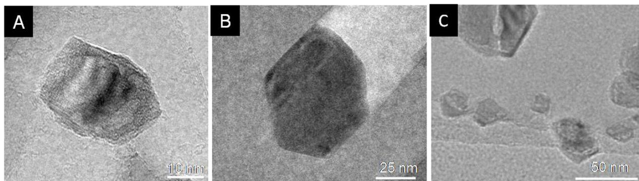
Figure S1. TEM micrographs of faceted nanoparticles obtained after ammonia treatments: A) core-shell, B) homogenous, C) semi-core shell.
