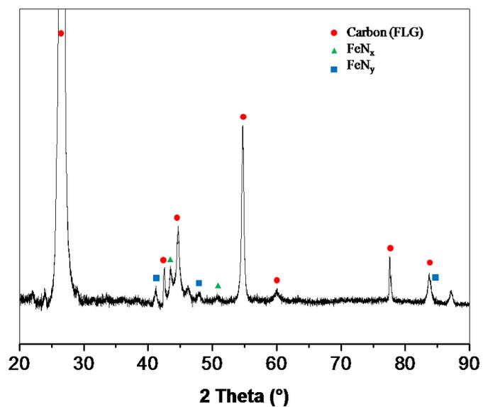
Figure S2. DRX pattern of ammonia treated FLG-supported  $\text{Fe}_3\text{O}_4$  particles.
