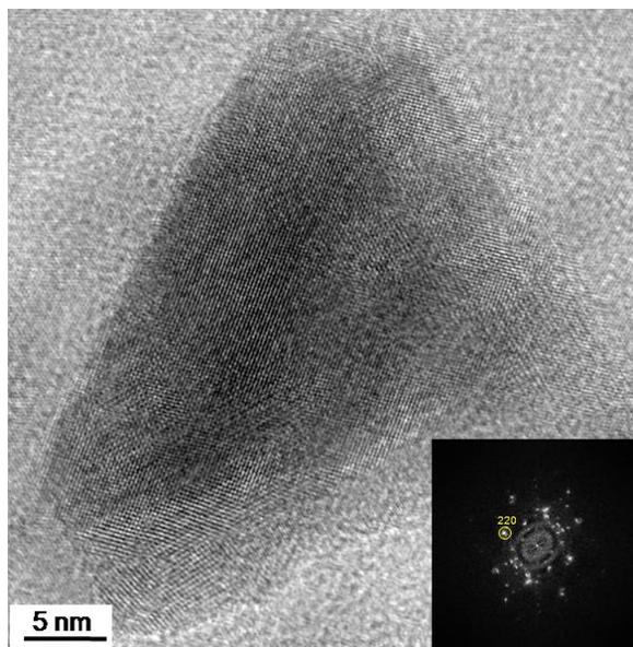
Figure S3. HR-TEM micrograph and electron diffraction of  $\text{Fe}_{16}\text{N}_2$  containing particle ( $d_{220}=0,214$  nm).
