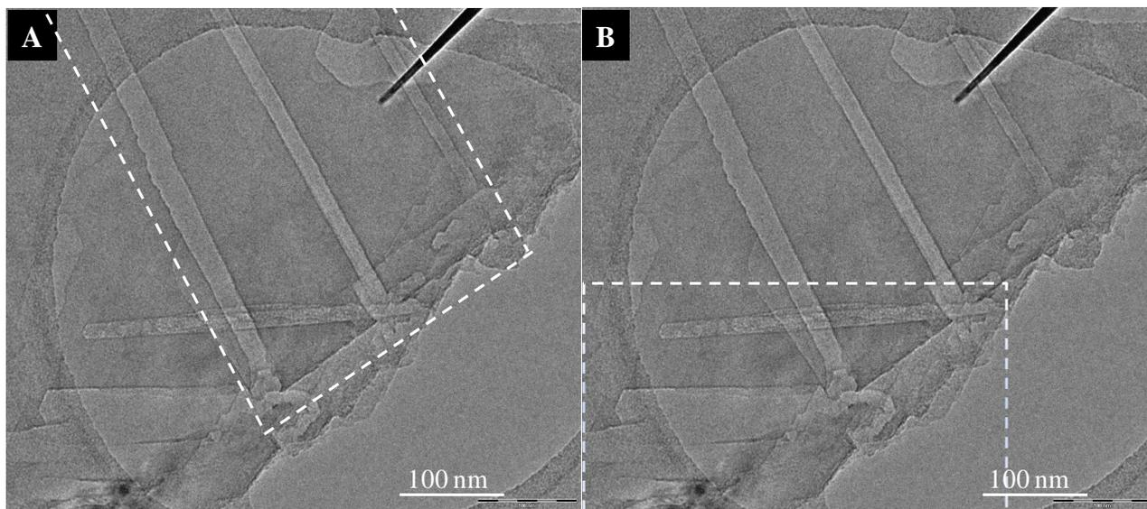
Figure S5. TEM micrograph with two zones (A) and (B) of two catalyst-free FLG assemblies, where graphene etching proceeded with direction perpendicular to the edges in the first zone (A) and at  $60^\circ$  from the edges in the second zone (B).
