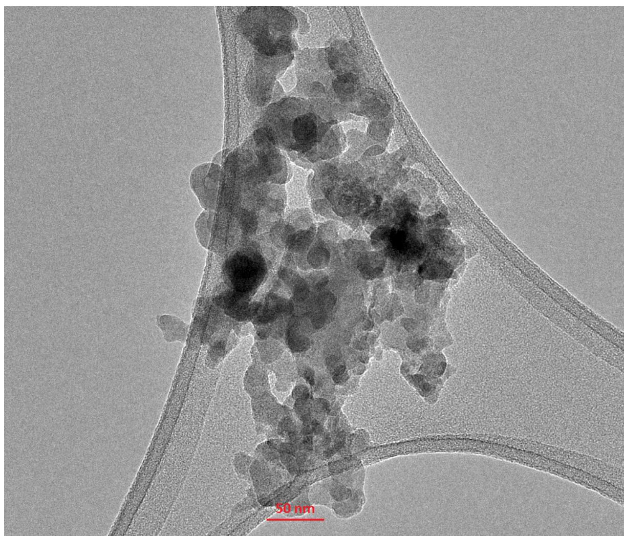
Figure S1. Transmission microscope images of NdP<sub>5</sub>O<sub>14</sub> nanocrystals
