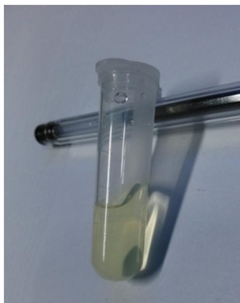
**Figure S4.** Homogeneous solution containing SP3 membrane fragments after immersing in 1.5M  $\text{VO}_2^+$  at 40 °C for 54 h.
