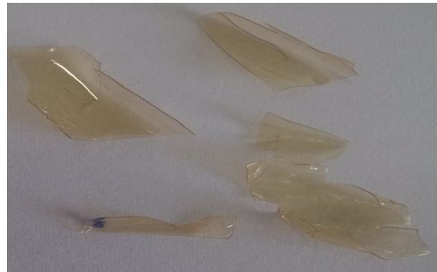
**Figure S3.** SP3 membrane fragments (after soaked in 1.5 M  $\text{VO}_2^+$  at 40 °C for 30 h)
