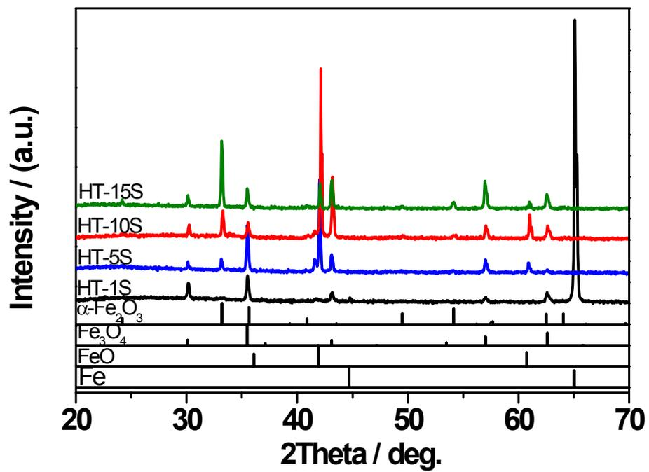
**Fig. S3** XRD patterns of HT-1S, HT-5S, HT-10S and HT-15S electrode.
