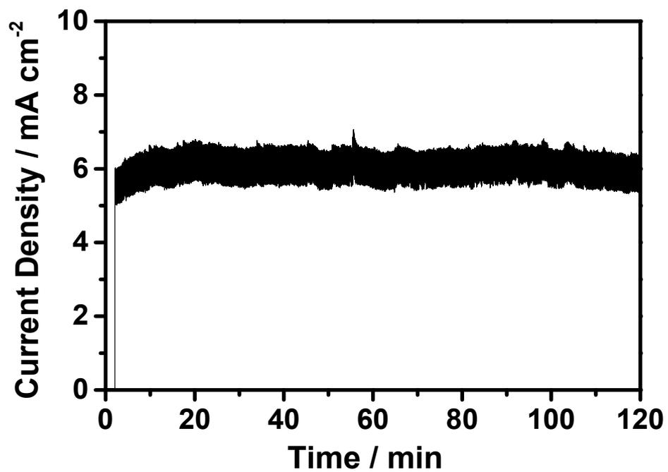
**Fig. S11** Amperometric *i*-*t* curve for HT-10S electrode in 1 M NaOH (pH 13.6) at 1.23 V vs. RHE.
