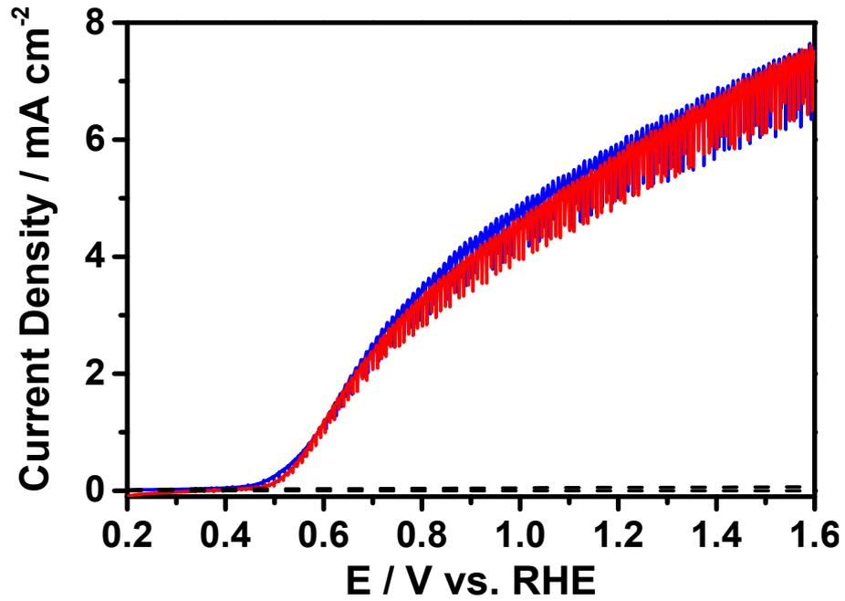
**Fig. S14** LSV curves for HT-10S electrode in 1 M NaOH (pH 13.6) before (blue) and after (red) i-t test. Light source: 300 W Xe lamp. The onset potential obtained with high-intensity Xe lamp was found to be 0.05 V more negative than that obtain using low-intensity AM 1.5 G light source. These results demonstrated the high stability of the present hematite photoelectrode.
