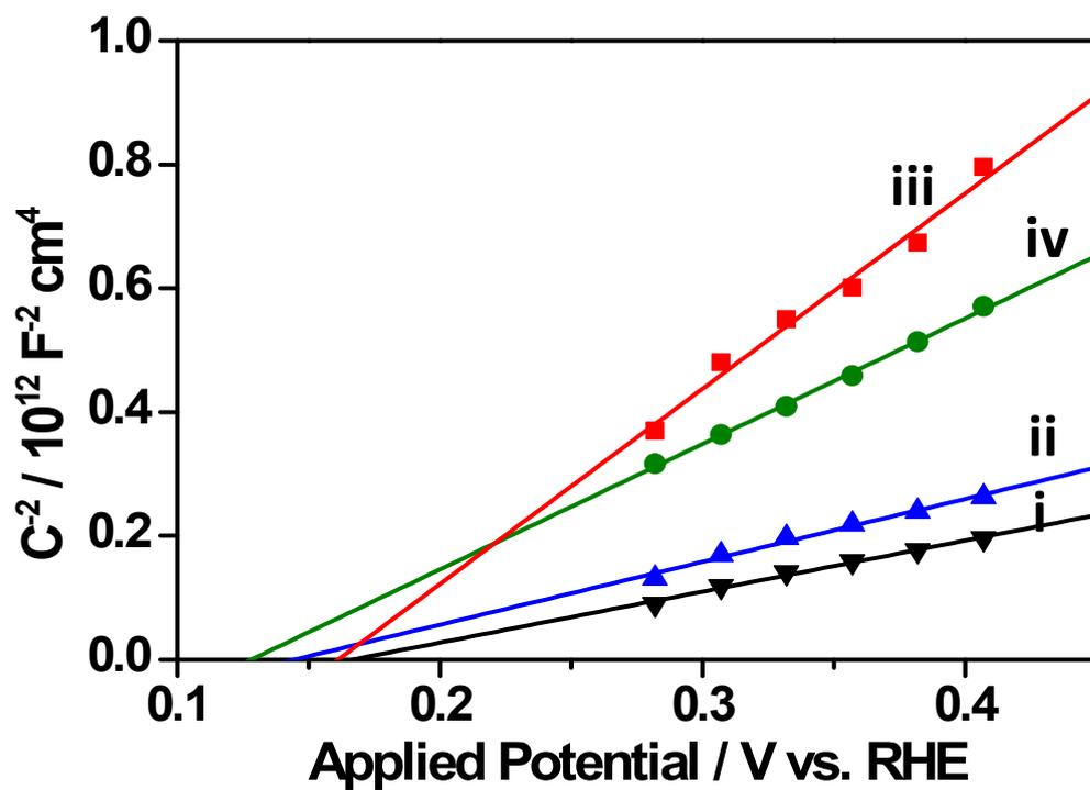
**Fig. S2** Mott-Schottky plots for HT-1S (i), HT-5S (ii), HT-10S (iii) and HT-15S (iv) electrodes measured in 1 M NaOH (pH 13.6) electrolyte. Frequency: 1000 Hz; Amplitude: 25 mV.
