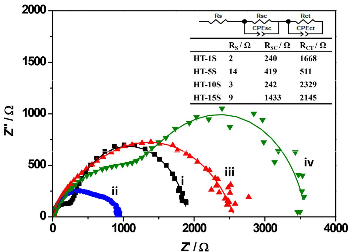
**Fig. S8** Nyquist plots for impedance spectroscopy data measured at pH 13.6 at 1.23 V vs. RHE of HT-1S (i), HT-5S (ii), HT-10S (iii) and HT-15S (iv) electrodes under AM 1.5 G illumination. A simple model with two interfaces is used to simulate the IS of hematite.
