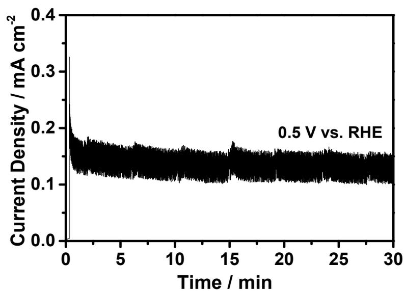
**Fig. S10** Amperometric *i-t* curve for HT-10S electrode in 1 M NaOH (pH 13.6) at 0.5 V vs. RHE. Light source: 300 W Xe lamp. The use of the high intensity Xe lamp instead of low intensity AM 1.5 G light source during the measurement will facilitate the analysis of the experimental results.
