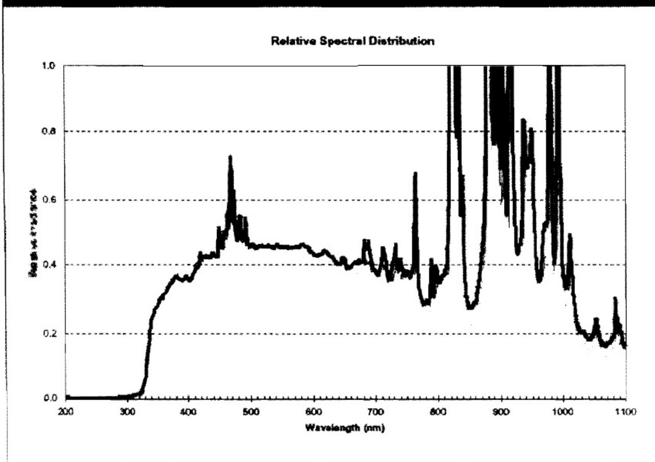
Fig. S12 the relative spectral distribution of the 300 W Xe lamp.
