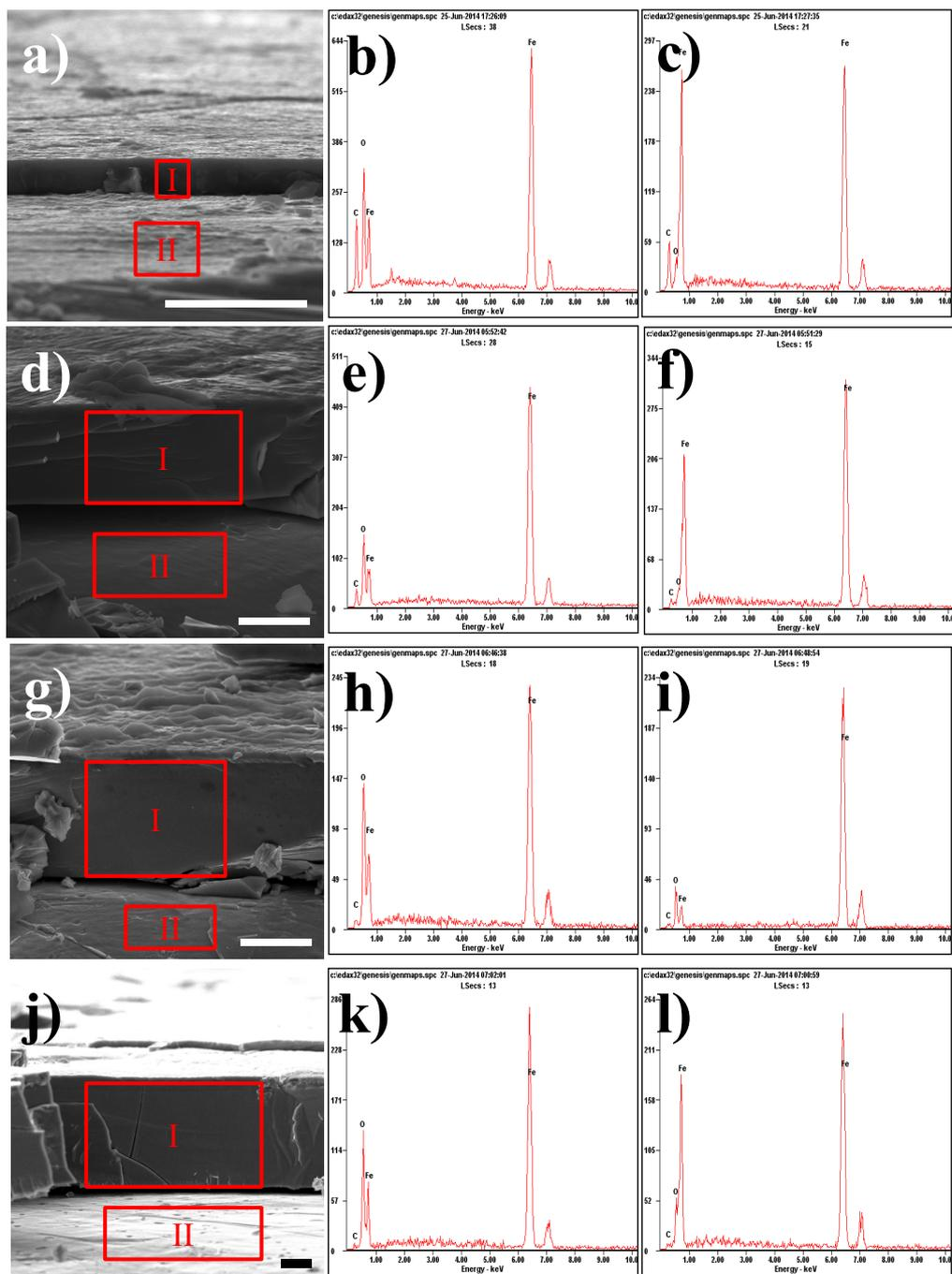
**Fig. S6** a) cross sectional SEM images of HT-1S, b) EDS analysis in area I in a), c) EDS analysis in area II in a), d) SEM side images of HT-5S, e) EDS analysis in area I in d), f) EDS analysis in area II in d), g) SEM side images of HT-10S, h) EDS analysis in area I in g), i) EDS analysis in area II in g), j) SEM side images of HT-15S, k) EDS analysis in area I in j), l) EDS analysis in area II in j), (scale bar stands for 10  $\mu\text{m}$ ).
