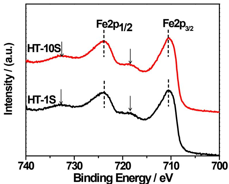
**Fig. S5** XPS spectra of HT-1S and HT-10S (the binding energies are calibrated by the binding energy of C1s 285 eV). The binding energy of Fe2p<sub>3/2</sub> and Fe2p<sub>1/2</sub> are 710.6 eV and 723.9 eV respectively, which is a characteristic position for Fe<sup>3+</sup>. Particularly, the satellite peaks (see arrows) at high binding energy give the existence of Fe<sup>3+</sup> species on the surface.
