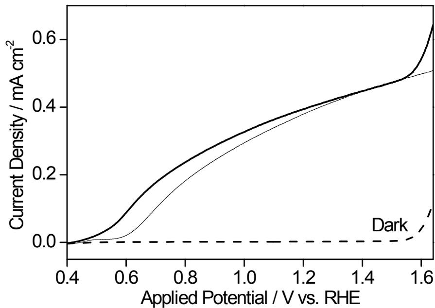
**Fig. S1** LSV curve for Co-Pi/HT-10S electrode under light irradiation and in dark. Electrolyte: 1.0 M NaOH (pH 13.6) aqueous solution; Light source: AM 1.5 G 100 mW cm<sup>-2</sup>; Scan rate: 20 mV s<sup>-1</sup>. The solid and dash lines indicate the scans under light and dark conditions, respectively. The fine line shows the LSV curve of HT-10S.
