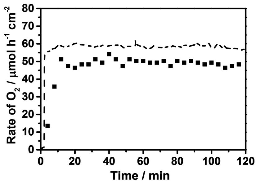
**Fig. S13** The rate of O<sub>2</sub> evolution for HT-10S electrode in 1 M NaOH (pH 13.6) at 1.23 V vs. RHE.
