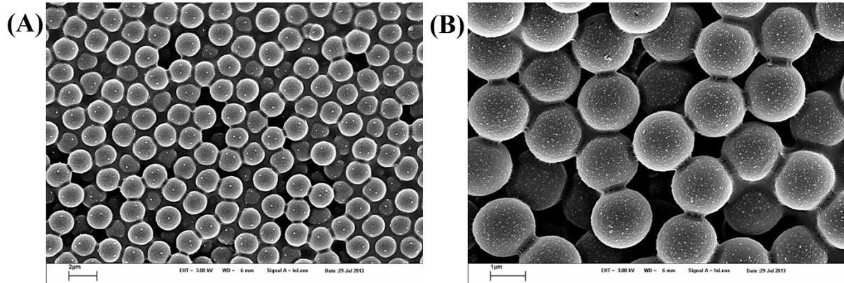
**Figure S.1** SEM images of colloidal silica after adsorption of (A) silver-citrate nanoparticles (scale bar is 2 μm) or (B) silver-PAA nanoparticles (scale bar is 1 μm).
