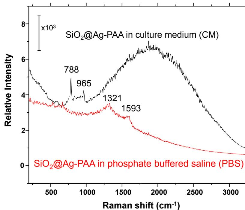
**Figure S.10** SERS spectra of culture medium (CM, black) or phosphate buffered saline (PBS, red) bulk aqueous solutions after incubation with SiO<sub>2</sub>@Ag-PAA particles without fibroblasts. The laser excitation wavelength was 532 nm and the grating was 600 g·mm<sup>-1</sup> (BLZ = 500 nm). The broad peak (black curve) is due to the autofluorescence.
