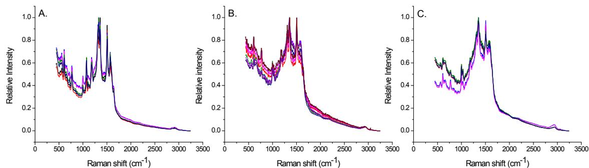
**Figure S.5** SERS spectra of Rh6G ( $10^{-8}$  mol·L $^{-1}$ ) in aqueous solution of SiO $_2$ @Ag-PAA particles as single (A), dimers (B) or closely-packed self-assembly (C). The excitation wavelength was 532 nm with the grating 600 g·mm $^{-1}$  (BLZ = 500 nm) and a spectral resolution of 3 cm $^{-1}$ . The SERS spectra are cumulative and averaged over at least ten particles of each type.
