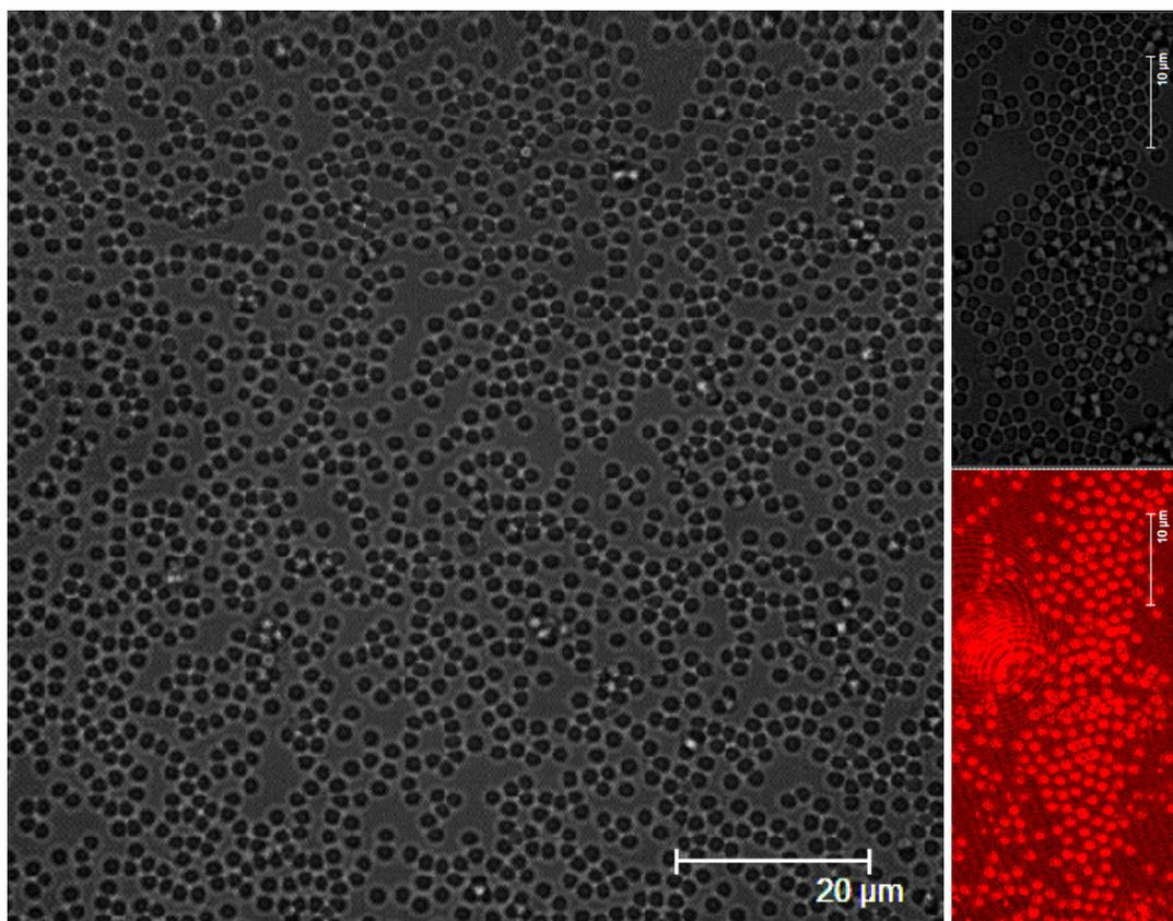
**Figure S.11** CLSM images of SiO<sub>2</sub>@Ag-PAA particles in PBS solution. On the left, CLSM image in transmission mode (scale bar is 20 μm) and on the right, in an excitation mode ( $\lambda_{\text{exc}} = 514 \text{ nm}$ ) after labelling with FITC-PAH (scale bar is 10 μm).
