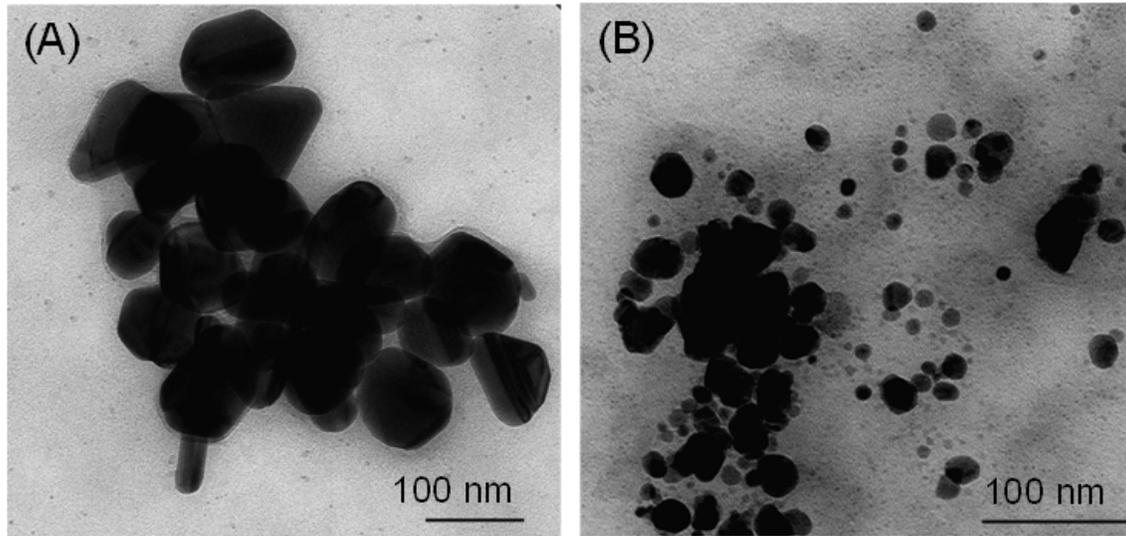
**Figure S.3** TEM images of silver-citrate nanoparticles formed by a Meisel's procedure (A) before and (B) after heating at 37°C (scale bars are 100 nm each).
