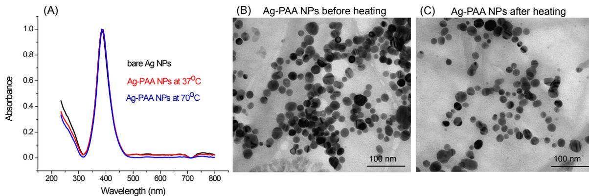
**Figure S.2** A) UV-Vis absorbance spectra of silver-citrate nanoparticles in the matrix of polyacrylic acid (PAA) before and after heating at 37°C in water. B) and C) TEM images of Ag-PAA NPs before and after heating at 37°C (scale bar is 100 nm).
