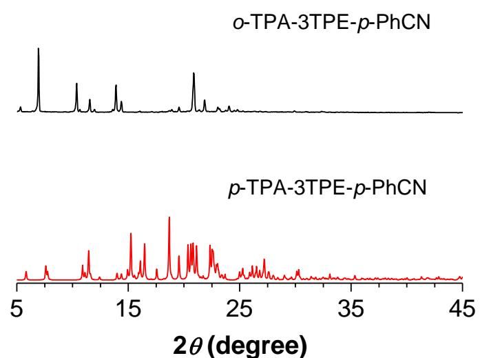
**Fig. S12** Powder XRD patterns for microcrystals of *o*-TPA-3TPE-*p*-PhCN and *p*-TPA-3TPE-*p*-PhCN at room temperature, respectively.
