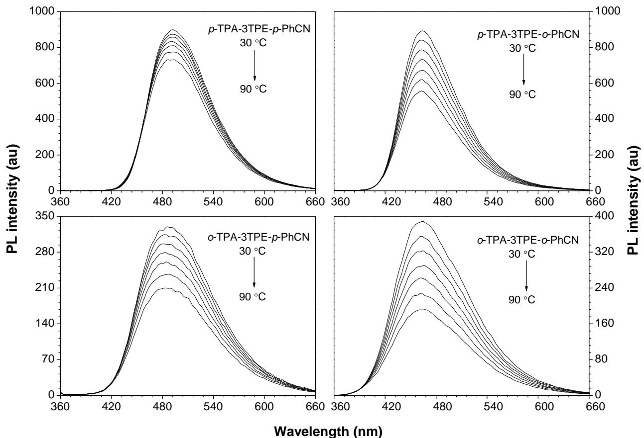
**Fig. S13** Emission spectra of D-3TPE-A molecules in the thin film at different temperatures.
