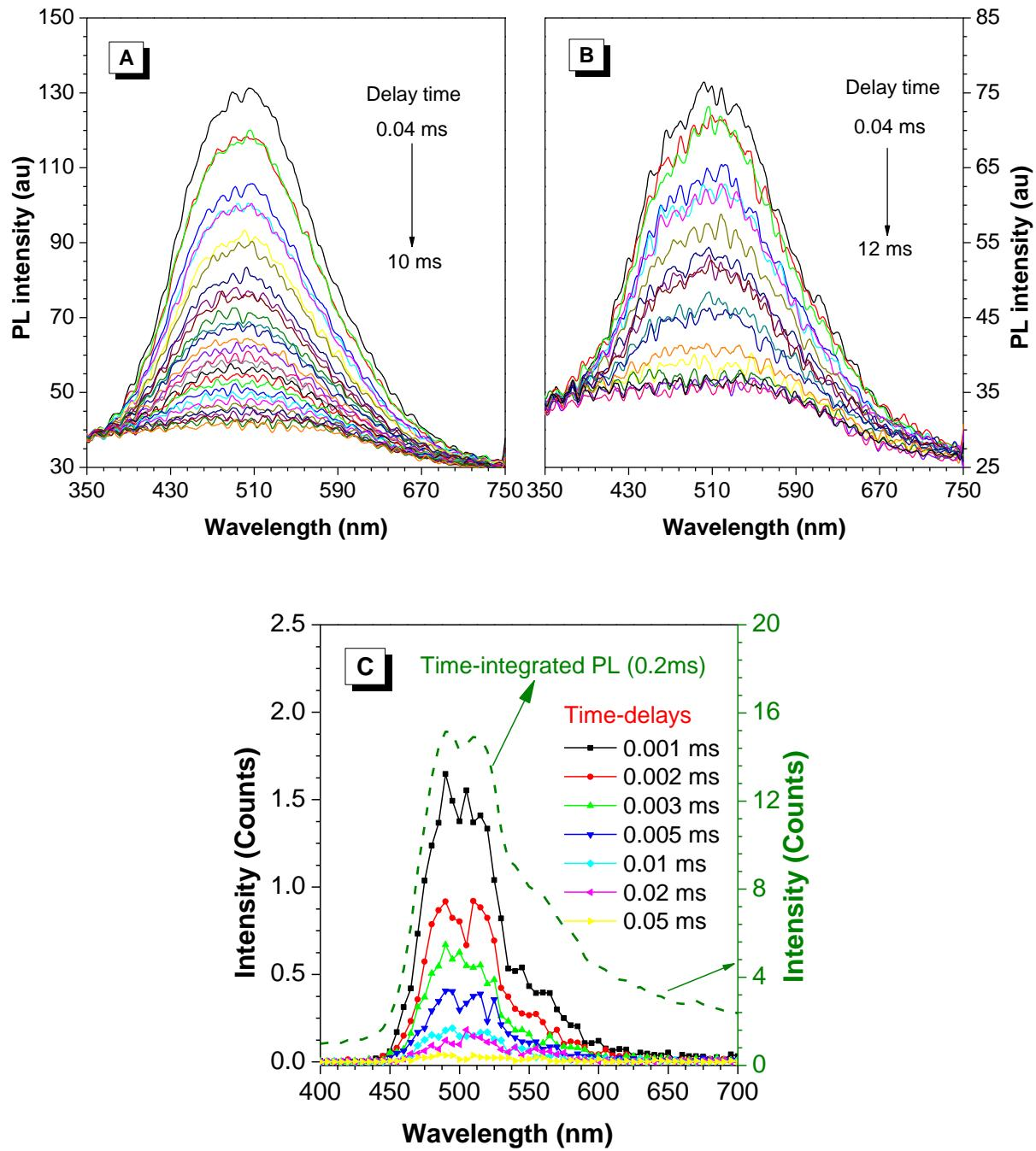
**Fig. S10** Emission spectra with different delay times of crystals of (A) *o*-TPA-3TPE-*o*-PhCN, (B) *o*-TPA-3TPE-*p*-PhCN and (C) *p*-TPA-3TPE-*p*-PhCN at room temperature. (A) and (B) were obtained by time window method using a Perkin-Elmer LS 55 spectrofluorometer, (C) was measured via a time-resolved fluorescence spectrometer with the time resolution of 1  $\mu$ s.
