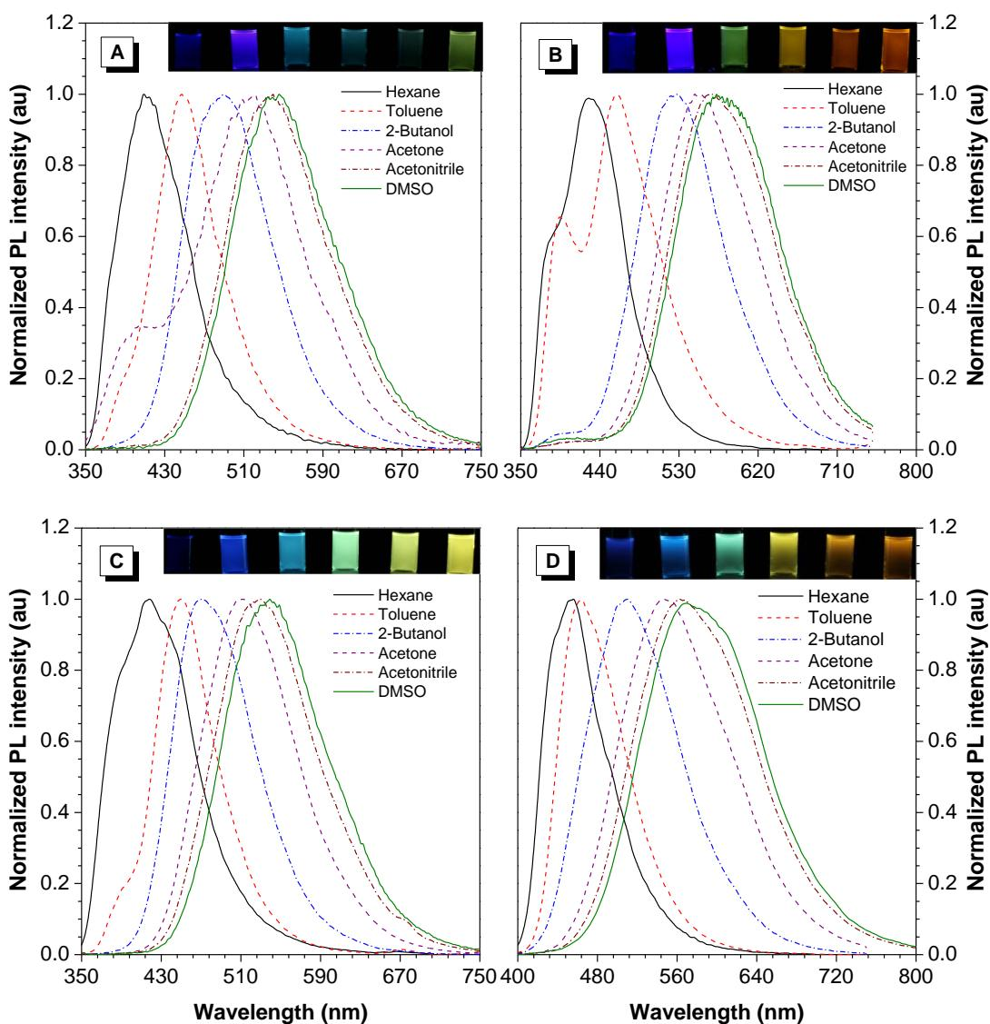
**Fig. S9** Normalized PL spectra of (A) *o*-TPA-3TPE-*o*-PhCN, (B) *o*-TPA-3TPE-*p*-PhCN, (C) *p*-TPA-3TPE-*o*-PhCN and (D) *p*-TPA-3TPE-*p*-PhCN in different solvents. Concentration: 10  $\mu$ M.
