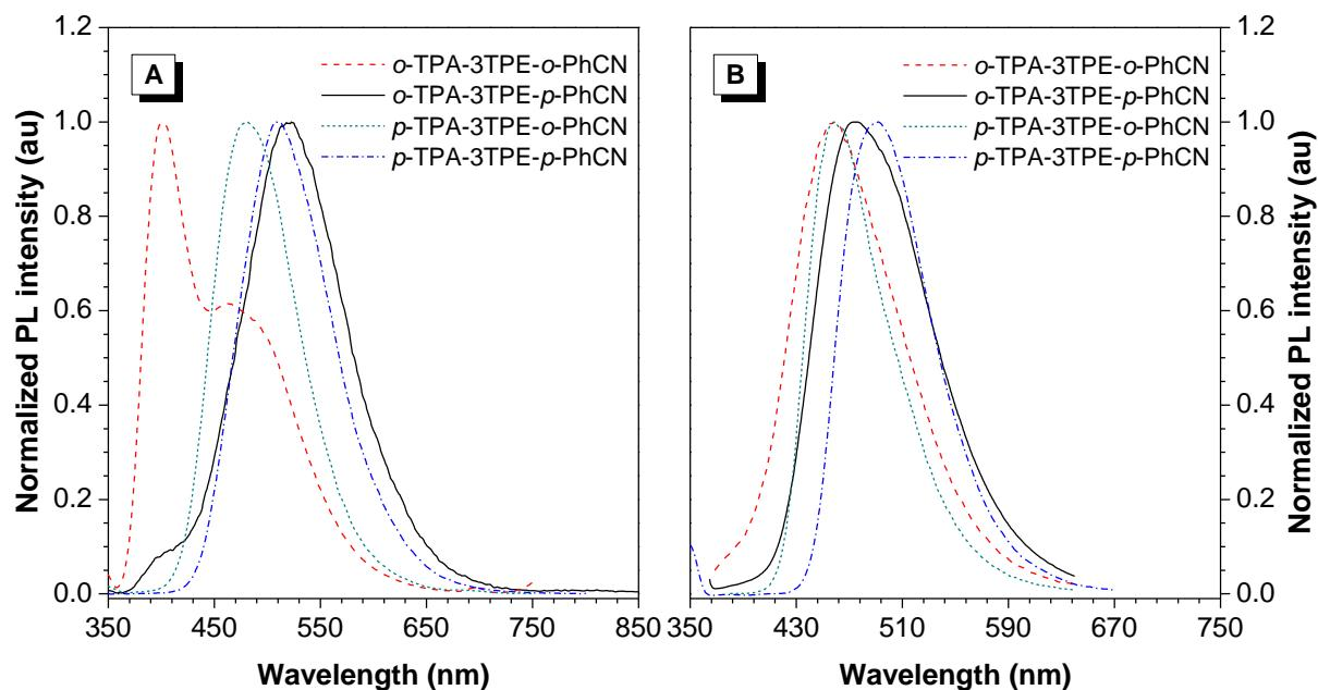
**Fig. S6** Normalized PL spectra of D-3TPE-A molecules in (A) THF solution and (B) film state.
