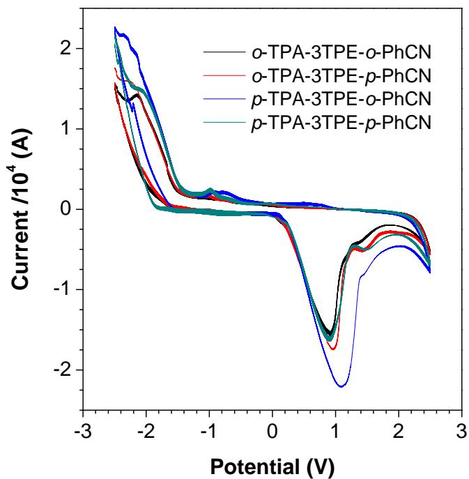
**Fig. S7** Cyclic voltammogram of D-3TPE-A molecules measured in dichloromethane containing 0.1 M tetra-n-butylammonium hexafluorophosphate. Scan rate: 100 mV/s.
