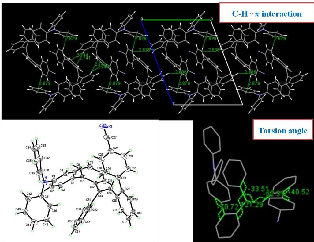
**Fig. S11.** Single crystal structure of *o*-TPA-3TPE-*o*-PhCN.
