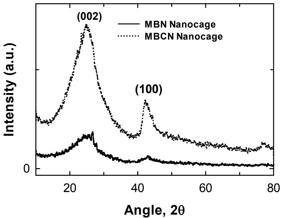
**Fig. 1** High angle X-ray diffraction pattern of MBN and MBCN nanocages
