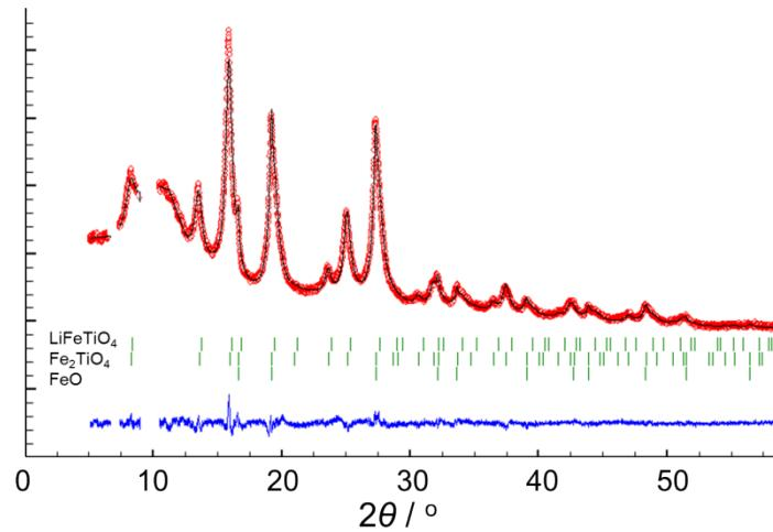
**Fig. S4** Rietveld refinement of 100<sup>th</sup> discharged LiFeTiO<sub>4</sub>. Space group: *Fd-3m*, *R*-factors:  $R_p = 8.51$ ,  $R_{wp} = 8.44$ ,  $R_e = 6.30$ . Fe<sup>3+</sup> cations were distributed as: (Fe<sub>0.11</sub>)<sub>8a</sub>[Fe<sub>0.17</sub>]<sub>16c</sub>[Fe<sub>0.08</sub>]<sub>16d</sub> derived from the Rietveld refinement. Note that the Fe and Ti have very close X-ray scattering factors. The 2θ region at about 10° was excluded for refinement.
