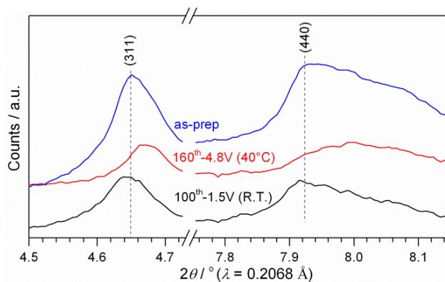
**Fig. S3** *Ex situ* synchrotron XRD patterns of (311) and (440) Bragg peaks of as-prepared and cycled LiFeTiO<sub>4</sub>.
