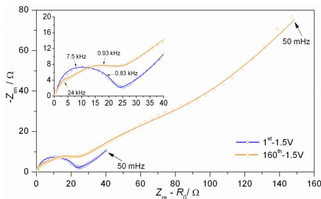
**Fig. S5** Complex impedance plots of LiFeTiO<sub>4</sub> at fully discharged states (1.5 V) from the first and extended cycles tested at 40°C. Inset shows the enlarged plots at high frequent regions.
