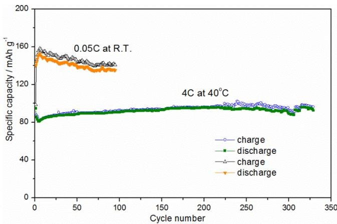
**Fig. S1** Charge/discharge capacities of LiFeTiO<sub>4</sub> measured at a 0.05C rate at room temperature and at a 4C rate at 40 °C in the voltage range of 1.5–4.8 V vs. Li<sup>+</sup>/Li.
