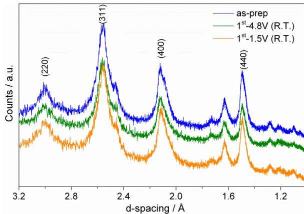
**Fig. S2** *d*-spacing of as-prepared LiFeTiO<sub>4</sub> and samples collected from the first charge-discharge cycle at room temperature.
