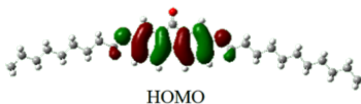
Fig. S1 Semiempirically calculated charge density contours of the HOMO for F-OC 9 .
