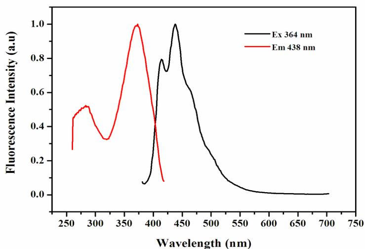
**Fig. S6** Normalized fluorescence excitation and emission spectra of CPPBI in chloroform at a concentration of  $1.0 \times 10^{-9}$  mol/L.
