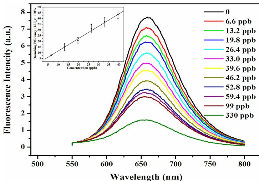
**Fig. S18** Fluorescence emission spectra of the CPPBI functionalized film recorded at different vapor pressures of aniline ( $\lambda_{\text{ex}} = 364$  nm). Inset is the plot of quenching efficiency against analyte concentration, of which the results utilized are from three parallel measurements.
