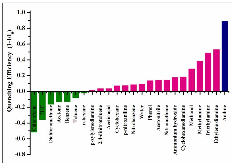
**Fig. S17** Fluorescence response of the film to various reagents with injection of 5 mL saturated vapor of various reagents into the quartz cell (~4.5 mL).
