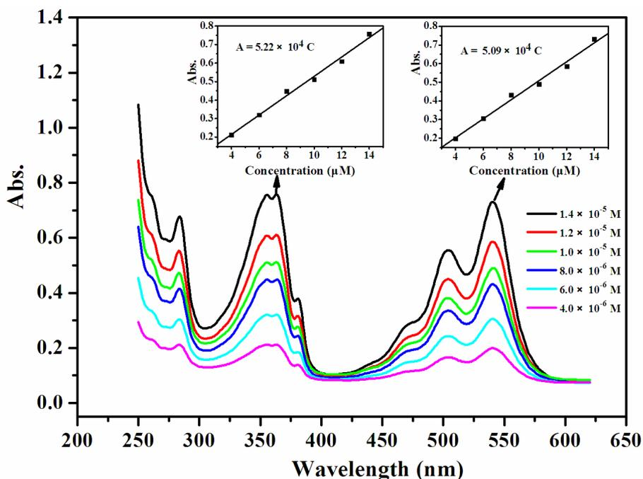
**Fig. S1** UV-Vis absorption spectra of CPPBI in chloroform at room temperature for concentrations from  $1.4 \times 10^{-5}$  mol/L to  $4.0 \times 10^{-6}$  mol/L. Insets are the change of the absorbance with increasing in the concentration, recorded at 364 and 541 nm, respectively. In the equation, “A” represents for the absorbance and “C” is the concentration of the samples under study.
