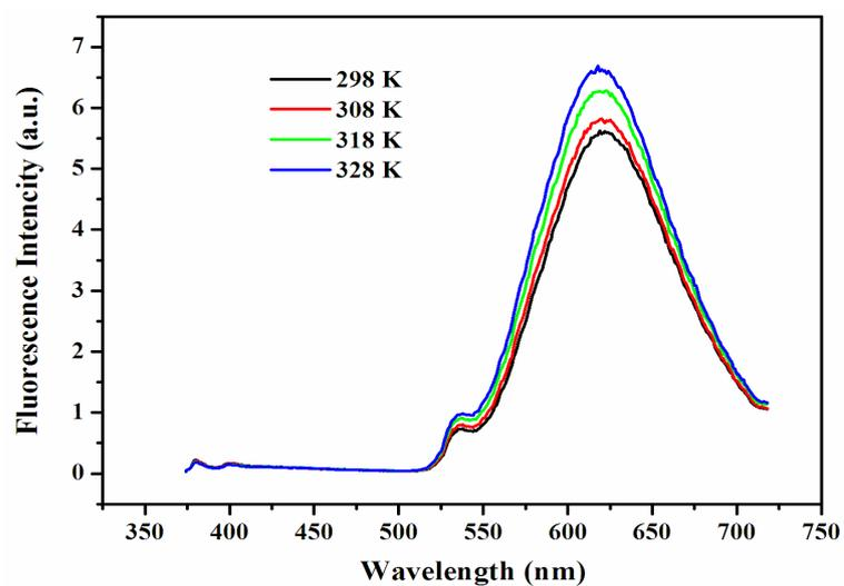
**Fig. S7** Temperature-dependent fluorescence emission spectra of CPPBI in chloroform at a concentration of  $5.0 \times 10^{-6}$  mol/L from 298 K to 328 K excited at 364 nm.
