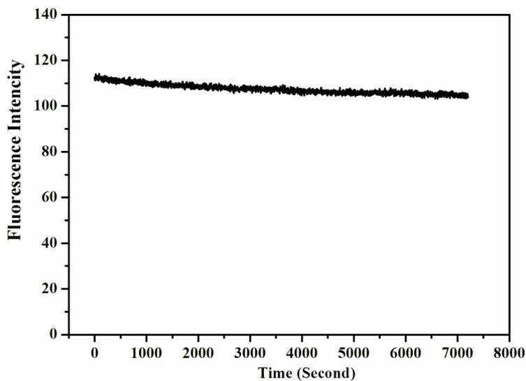
**Fig. S16** Fluorescence emission intensities recorded of CPPBI in film state excited at 364 nm, the monitored wavelength was 658 nm.
