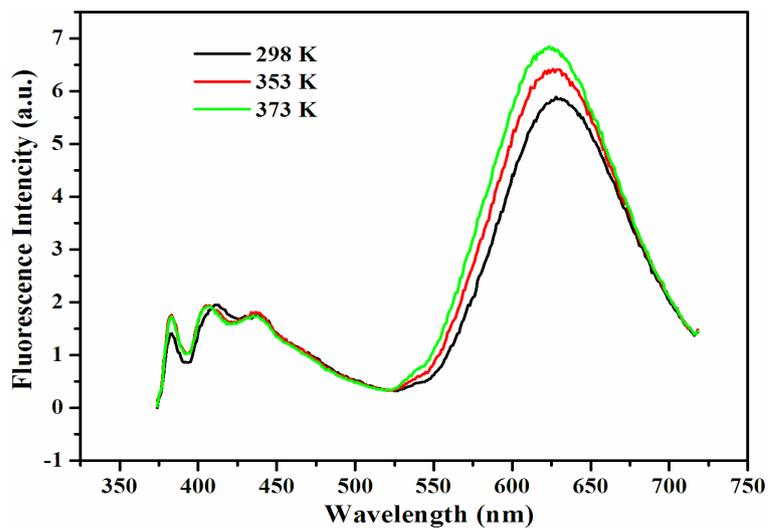
**Fig. S8** Temperature-dependent fluorescence emission spectra of CPPBI in tetrachloroethane at a concentration of  $5.0 \times 10^{-6}$  mol/L from 298 K to 373 K excited at 364 nm.
