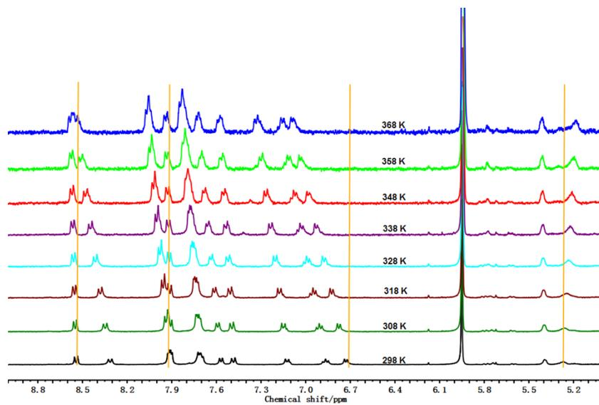
**Fig. S13** Temperature-dependent  $^1\text{H}$  NMR spectra of CPPBI in deuterated tetrachloroethane.
