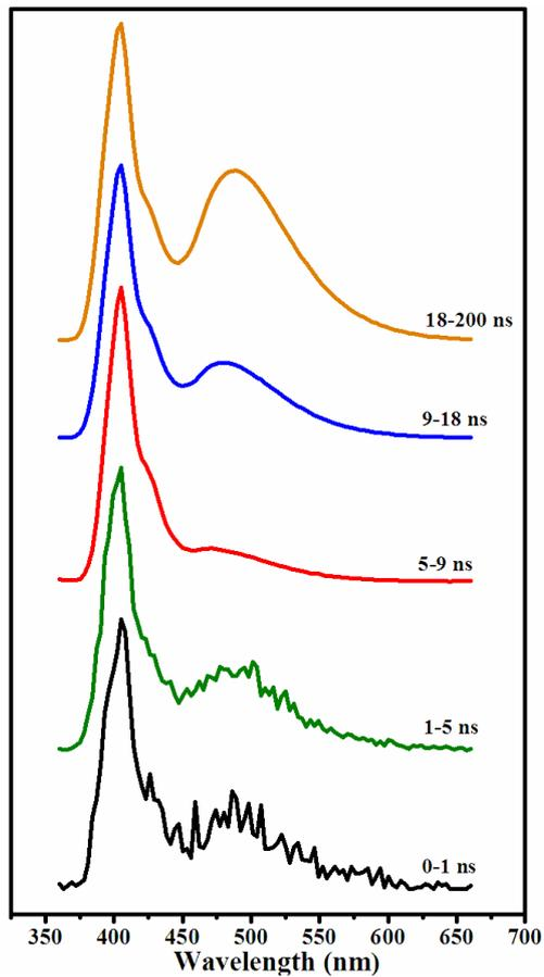
**Fig. S14** Time-resolved emission spectra of CPEC in chloroform at a concentration of  $1.0 \times 10^{-3} \text{ mol} \cdot \text{L}^{-1}$  using pico-second pulsed diode laser (EPL-340) as an excitation source.
