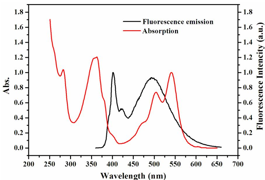
**Fig. S3** Normalized absorption (red) of CPPBI in chloroform ( $5.0 \times 10^{-6}$  mol/L) and emission spectra (black) of CPEC excited at 340 nm in chloroform ( $2.5 \times 10^{-3}$  mol/L).
