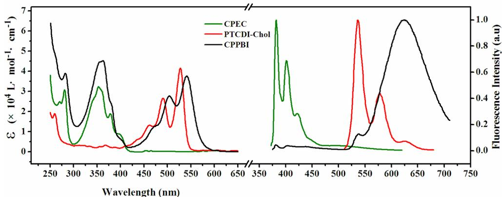
**Fig. S2** Normalized fluorescence emission (right) and absorption spectra (left) of CPPBI, CPEC, PTCDI-Chol in chloroform at a concentration of  $5.0 \times 10^{-6}$  mol/L, the excitation wavelengths of CPPBI, PTCDI-Chol and CPEC are 364 nm, 490 nm and 350 nm, respectively.
