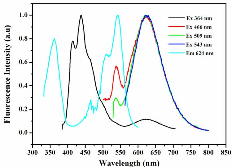
**Fig. S5** Normalized fluorescence excitation and emission spectra of CPPBI in chloroform at a concentration of  $1.0 \times 10^{-8}$  mol/L. The detected wavelength was set at 624 nm, the excited wavelength was 364, 466, 509, and 543 nm, respectively.
