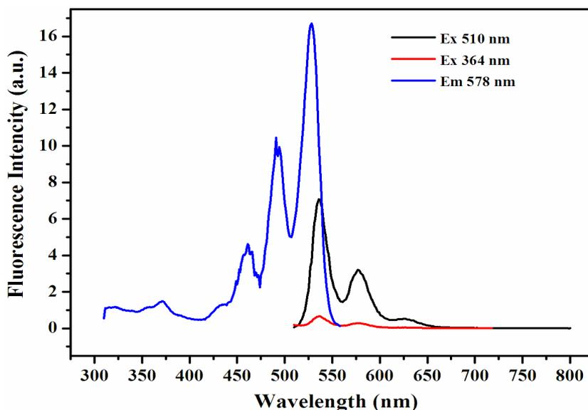
**Fig. S4** Fluorescence excitation and emission spectra of PTCDI-Chol in chloroform at a concentration of  $5.0 \times 10^{-6}$  mol·L<sup>-1</sup>. The detected wavelength was set at 578 nm, the excited wavelength was 364, 509, respectively.
