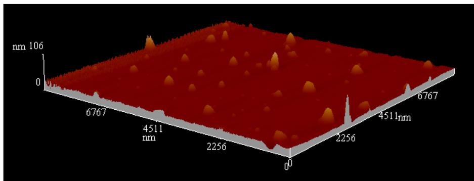
Fig. S11 The three dimensional AFM image of the aggregated CPPBI from its chloroform solution at a concentration of  $1.0 \times 10^{-6}$  mol/L.
