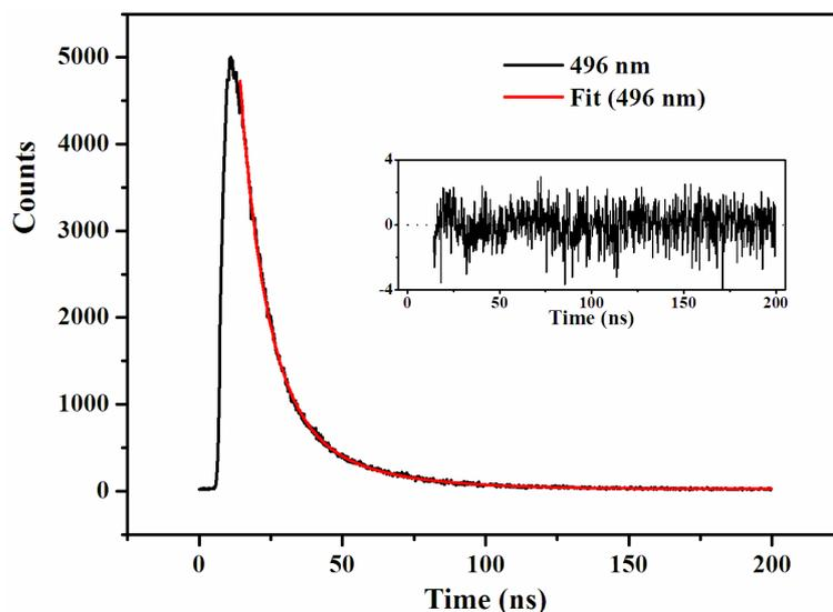
**Fig. S9** Lifetime at 496 nm of CPEC in chloroform at a concentration of  $1.0 \times 10^{-3}$  mol/L using pico-second pulsed diode laser (EPLD-340) as an excitation source,  $\tau_1 = 9.3$  ns (52.5%),  $\tau_2 = 27.6$  ns (47.5%),  $\tau_D = \tau_1 \times 52.5\% + \tau_2 \times 47.5\% = 18.0$  ns. Inset is the corresponding residual-distributions, the  $\chi^2$  value is 1.16.
