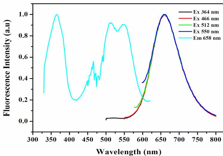
**Fig. S15** Normalized fluorescence excitation and emission spectra of the sensing film prepared by dip-coating CPPBI on a glass plate surface.
