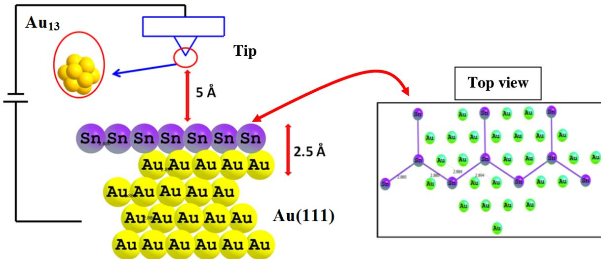
**Figure S5.** (Color online) (left) A schematic illustration of the STM-like setup for the electron. Transport calculations: Sn monolayer deposited on Au. (right) top view of the monolayer lattice commensurate with that of Au (111) surface.
