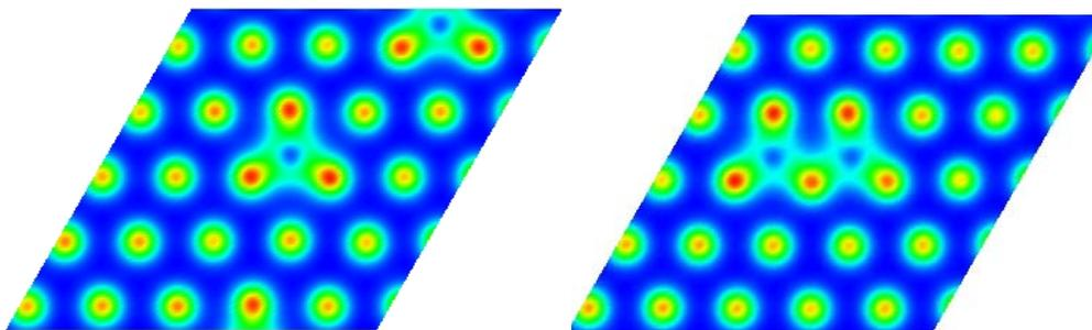
Figure -S2: The iso-surface density of  $\text{Sn}_2@Au_{111}$  in (a) far apart (b) bonded case. In both case charge has been transferred to nearby gold atoms.
