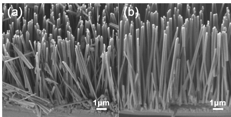
**Figure S1.** Side view SEM images of (a) annealed ZnO NRs and (b) annealed ZnO/Al<sub>2</sub>O<sub>3</sub> NRs.
