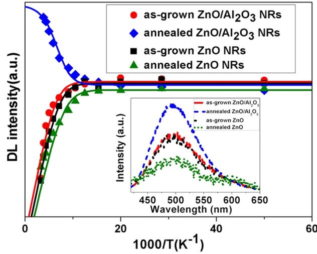
**Figure S4.** The temperature dependence of integrated DL intensity for the as grown ZnO/Al<sub>2</sub>O<sub>3</sub> NRs, annealed ZnO/Al<sub>2</sub>O<sub>3</sub> NRs, as grown ZnO NRs and annealed ZnO NRs, respectively. The solid lines are the fitting curves using Eq. (1). Inset shows the PL spectra of these samples at 260K.
