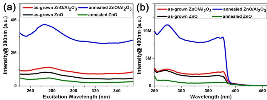
**Figure S5.** Photoluminescence excitation spectra of different samples collected at the wavelength of (a) 380nm and (b) 490nm. The collection bandwidth is 5nm.
