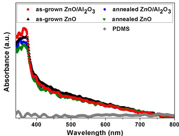
**Figure S3.** Absorption spectra for the as-grown ZnO/Al<sub>2</sub>O<sub>3</sub> NRs, annealed ZnO/Al<sub>2</sub>O<sub>3</sub> NRs, as-grown ZnO NRs, and annealed ZnO NRs, respectively. The absorption property of the transparent PDMS substrate is also plotted.
