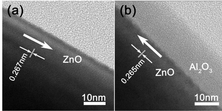
**Figure S2.** HRTEM images of an (a) as-grown ZnO NR and (b) as-grown ZnO/Al<sub>2</sub>O<sub>3</sub> NR.
