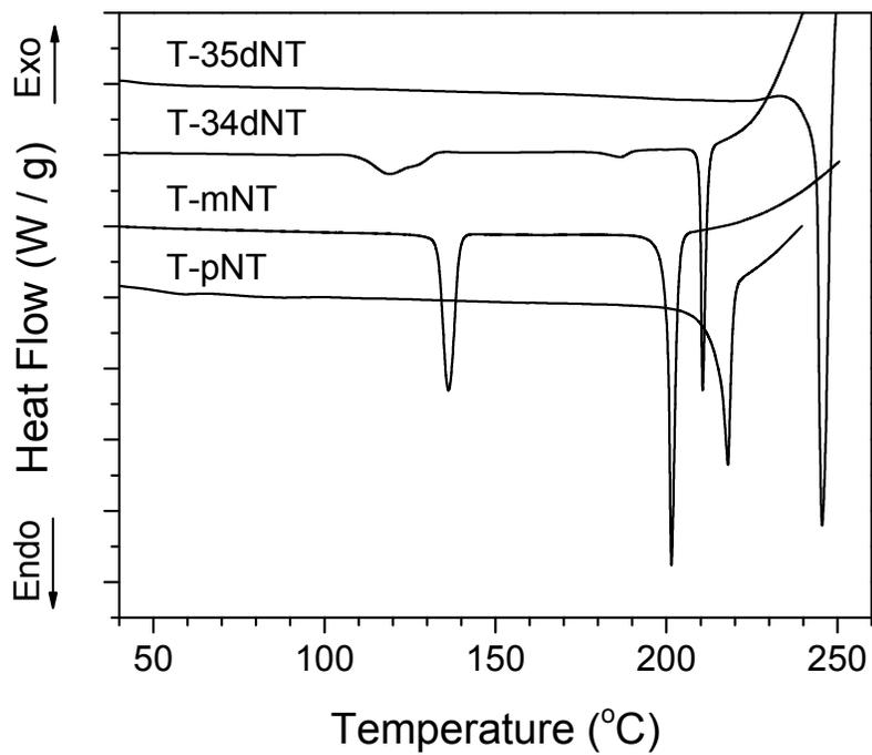
Figure S5. DSC thermograms of T-phenazine compounds.
