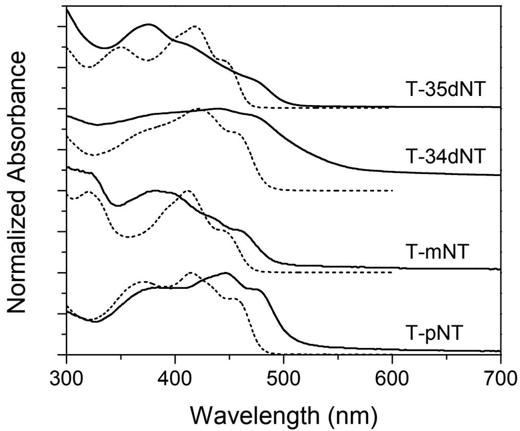
Figure S6. UV-vis spectra of T-phenazine compounds in solution (dashed line) and as films (solid line).
