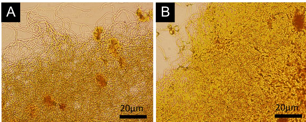
Figure S11. POM images of xerogel of **T-34dNT** from AN gel: (A) pristine and (B) dried for 1 week at ambient condition.
