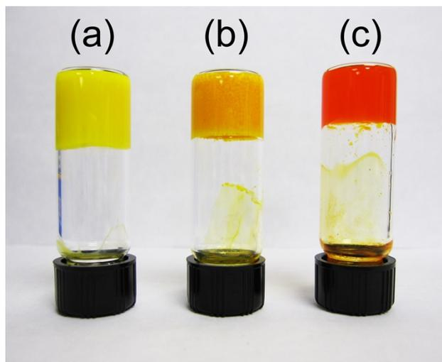
Figure S9. Pictures of **T-34dNT** gels: (a) in AN (7 mM), (b) in EA (10 mM), and (c) in cyclohexane (7 mM).
