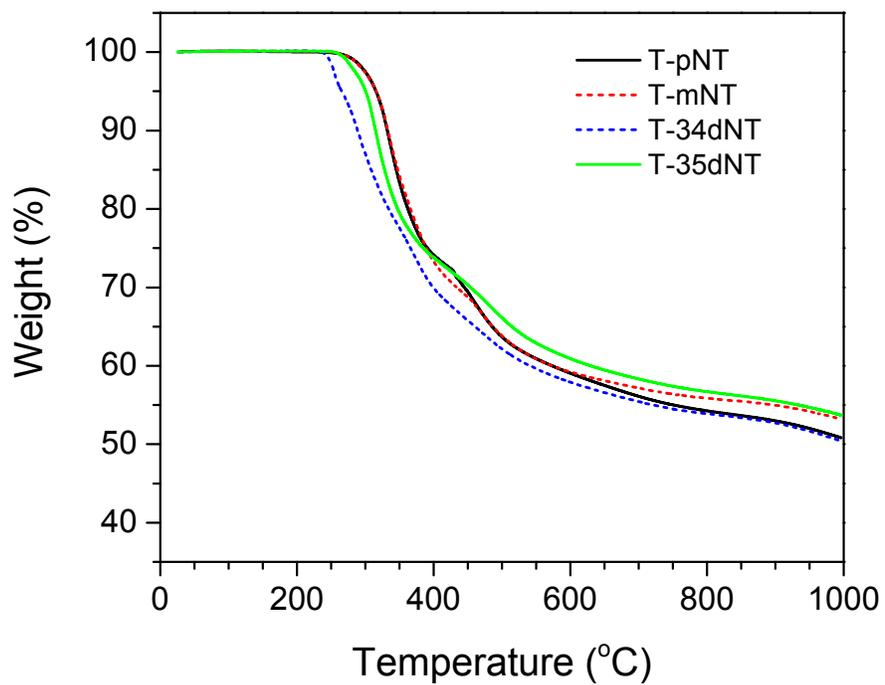
Figure S4. TGA thermograms of T-phenazine compounds.
