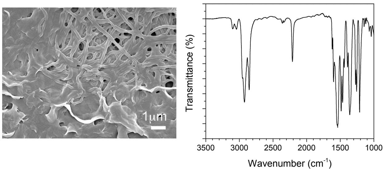
Figure S10. SEM image of xerogel of **T-34dNT** from AN gel dried for 1 week at ambient condition (left) and FT-IR spectrum of the corresponding sample (right).
