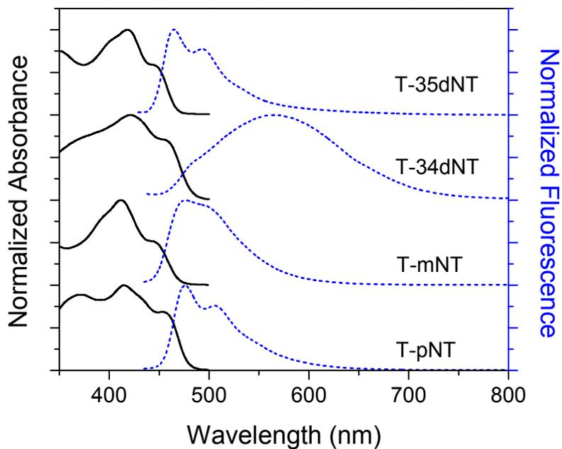
Figure S1. UV-vis absorption (solid line) and fluorescence (dashed line) spectra of T-phenazines in DCM. Excitation wavelength: 412 nm for **T-pNT** and **T-mNT**, and 422 nm for **T-34dNT** and **T-35dNT**.
