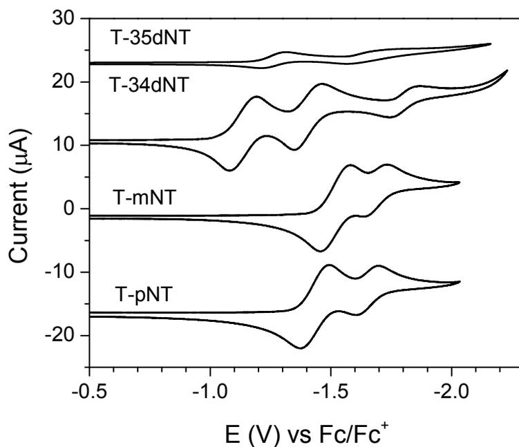
Figure S2. Cyclic voltammograms of NO<sub>2</sub> substituted T-phenazine molecules.
