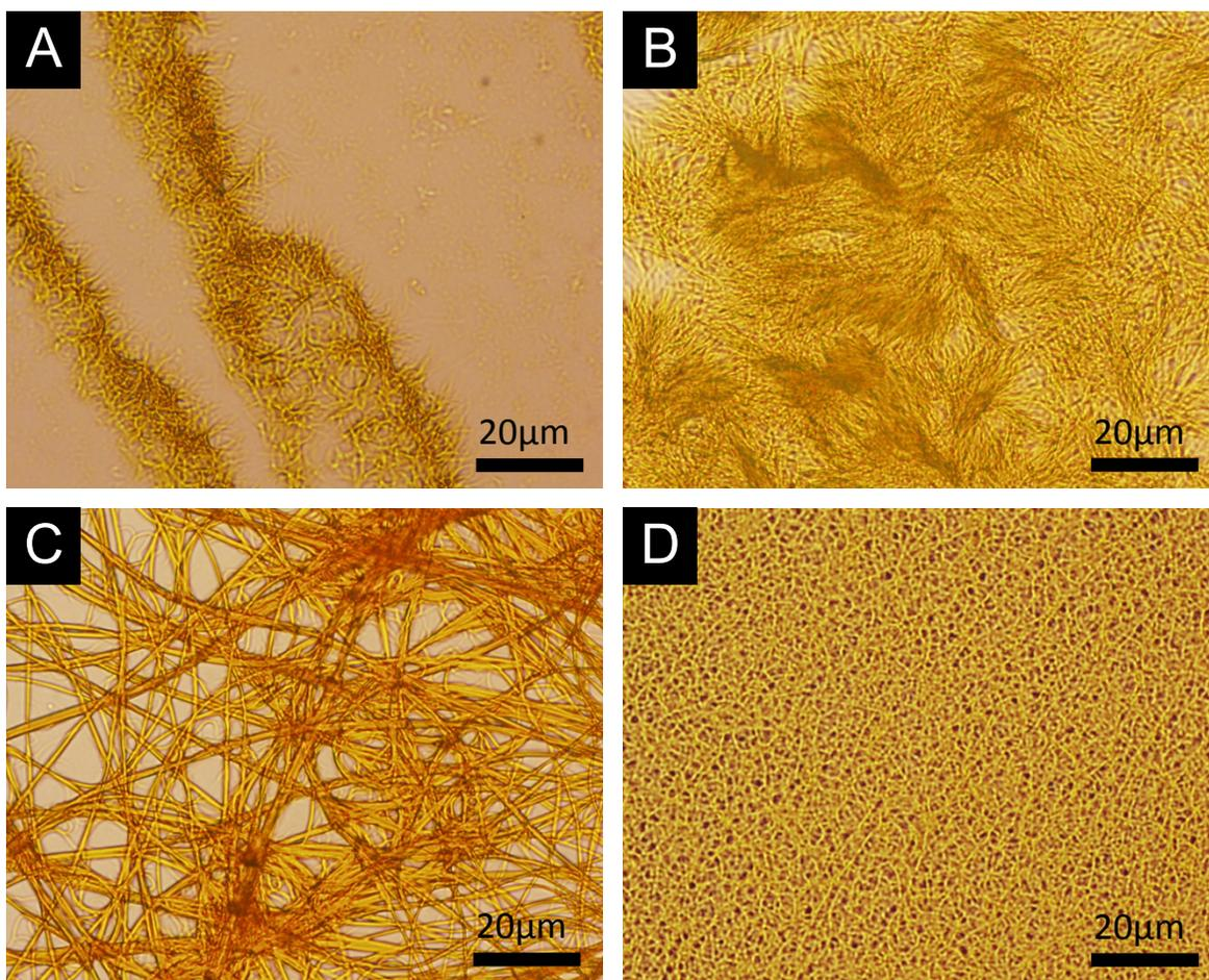
Figure S7. POM images of cast films from DCM solutions: (A) T-pNT, (B) T-mNT, (C) T-34DNT, and (D) T-35DNT.
