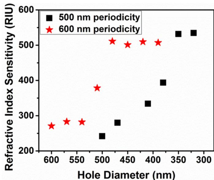
**Figure S8 Refractive index sensitivity for 500 nm and 600 nm periodicity templates with varying hole size.** The range over which the nanohole array is optimized for a refractive index sensor differs from a SERS sensor, as even though both effects originate in the local field, the SPP have a larger field decay length and more restrictive excitation condition, making it more sensitive than the LSPR to changes in the refractive index.
