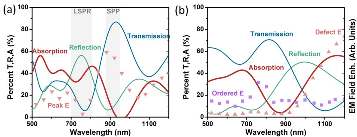
**Figure S5 Comparison of optical modes and resulting EM field enhancement for 600 nm periodicity.** The transmission (T), reflection (R), and absorption ( $A=1-T-R$ ) is compared to the peak EM field enhancement for an (a) ordered and (b) 'gap' defective pattern for a 600 nm template with 420 nm, 540 nm hole size, and 50 nm gap defects, respectively.
