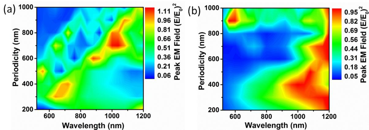
**Figure S9 Additional SERS tuning curves.** (a) The EM field corresponding to the optimal absorption condition. The EM field is slightly redshifted from the absorption peak. The EM field magnitude is normalized by the highest value for each periodicity (b) The ‘gap’ defect EM field, normalized for each periodicity individually to accentuate how the EM field changes as the template is varied.
