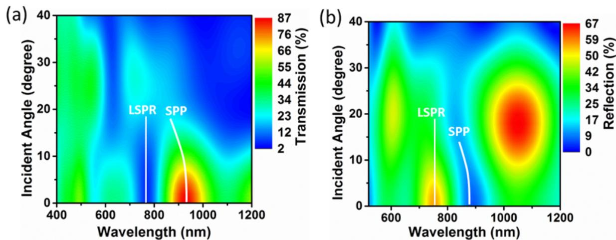
**Figure S4 Change in LSPR and SPP with incident angle.** (a) The transmission and (b) reflection show that the LSPR is relatively unaffected by the input angle while the SPP shifts due to the momentum matching condition changing.
