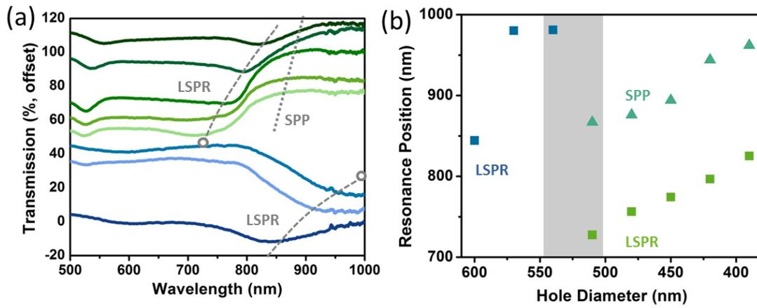
**Figure S3 Change in optical modes at transition zone for 600 nm periodicity.** (a) The transmission is shown for a set of hole sizes covering 600 nm to 390 nm in 30 nm intervals. (b) The estimated peak position of the LSPR and SPP peaks for each hole diameter with a fixed periodicity of 600 nm.
