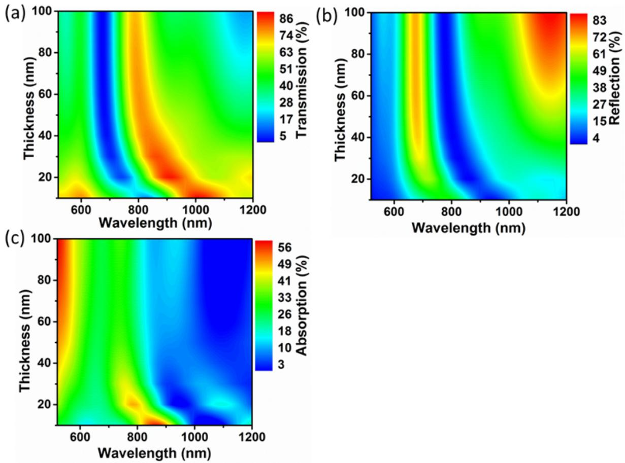
**Figure S10** Effect of metal thickness on optical properties. The transmission (T), reflection (R), and absorption ( $A=1-T-R$ ) is compared as the metal film thickness is changed for a 500 nm periodicity template with a hole size of 350 nm.
