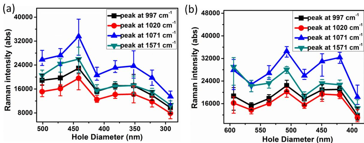
**Figure S7 Measured Raman Signal** The measured Raman intensity for 785 nm excitation at several nanohole sizes for (a) a 500 nm periodicity template and (b) a 600 nm periodicity template. Error bars represent the average of three measurements, each line corresponds to a different Raman transition.
