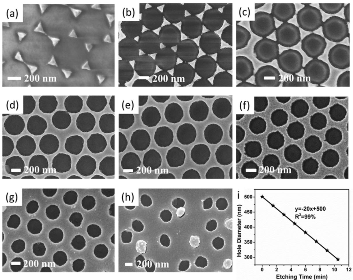
**Figure S1 SEM images for 500 nm periodicity template.** (a-h) Gold nanoarrays with a periodicity of 500 nm and hole diameters of 500 nm, 470 nm, 440 nm, 410 nm, 380 nm, 350 nm, 320 nm, 290 nm, and a film thickness of 50 nm; (i) linear relationship between the hole diameter and the etching time. For reference, the percentage of defects for the 440 nm hole size was ~50% from the SEM images.
