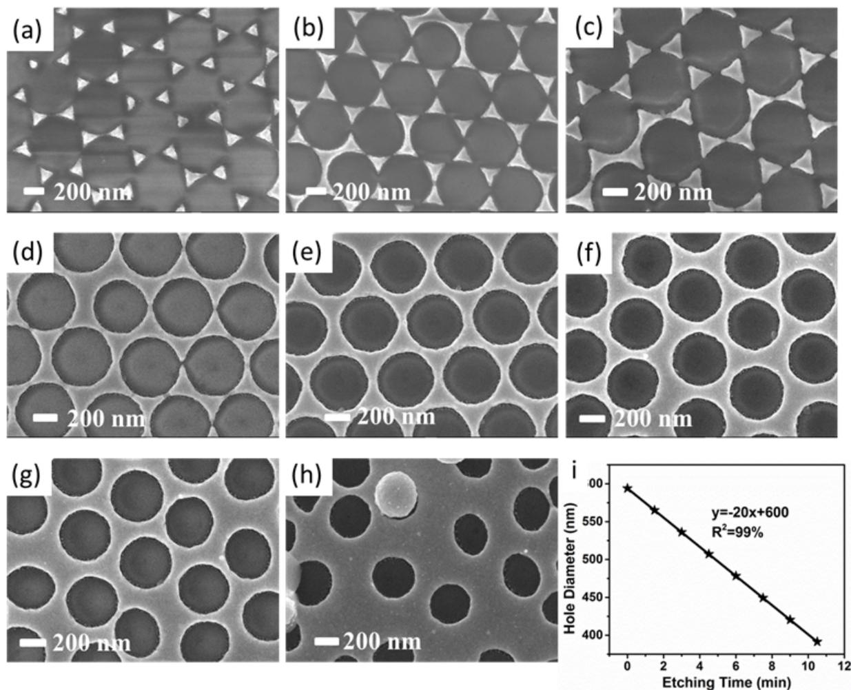
**Figure S2 SEM images for 600 nm periodicity template.** (a-h) Gold nanoarrays with a periodicity of 600 nm and hole diameters of 600 nm, 570 nm, 540 nm, 510 nm, 480 nm, 450 nm, 420 nm, 390 nm, and a film thickness of 50 nm; (i) linear relationship between the hole diameter and the etching time. For reference, the percentage of defects for the 540 nm hole size was ~85% from the SEM images.
