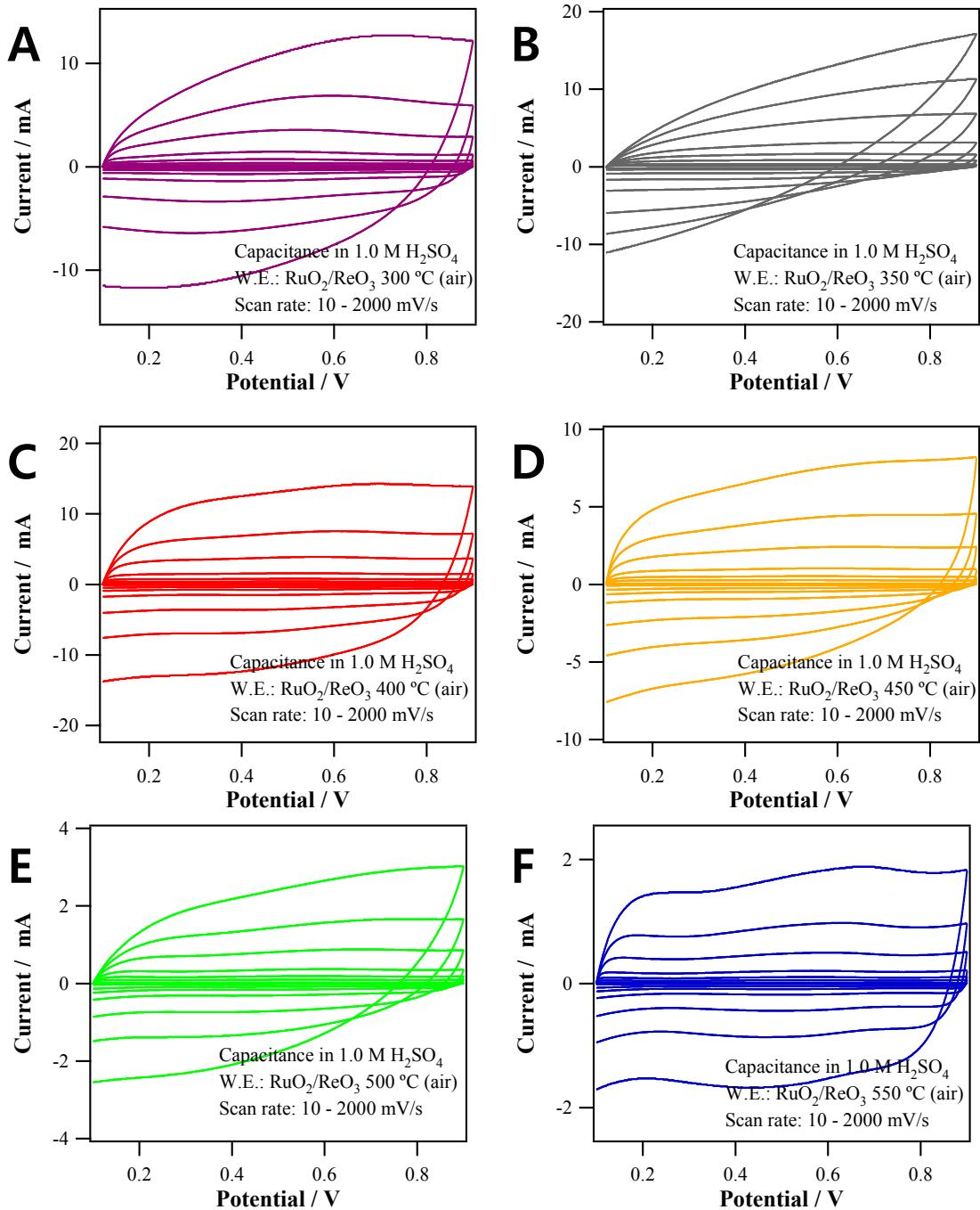
**Fig. S7.** Capacitance measurements of  $\text{RuO}_2\text{-ReO}_3(0.11)/\text{GC}$  in 1.0 M  $\text{H}_2\text{SO}_4$  solution with  $v$  of 100, 500, 1000, and 2000  $\text{mV s}^{-1}$  at various annealing temperatures.
