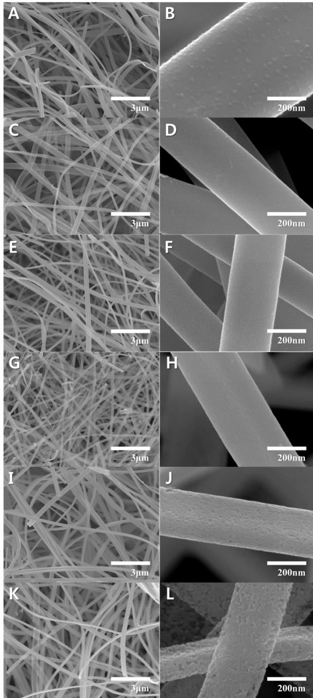
**Fig 3S.** SEM images of  $\text{RuO}_2\text{-ReO}_3(\text{n})$  composite nanofibers after thermal annealing process: at  $300^\circ\text{C}$  (A, B),  $350^\circ\text{C}$  (C, D),  $400^\circ\text{C}$  (E, F),  $450^\circ\text{C}$  (G, H),  $500^\circ\text{C}$  (I, J), and  $550^\circ\text{C}$  (K, L).
