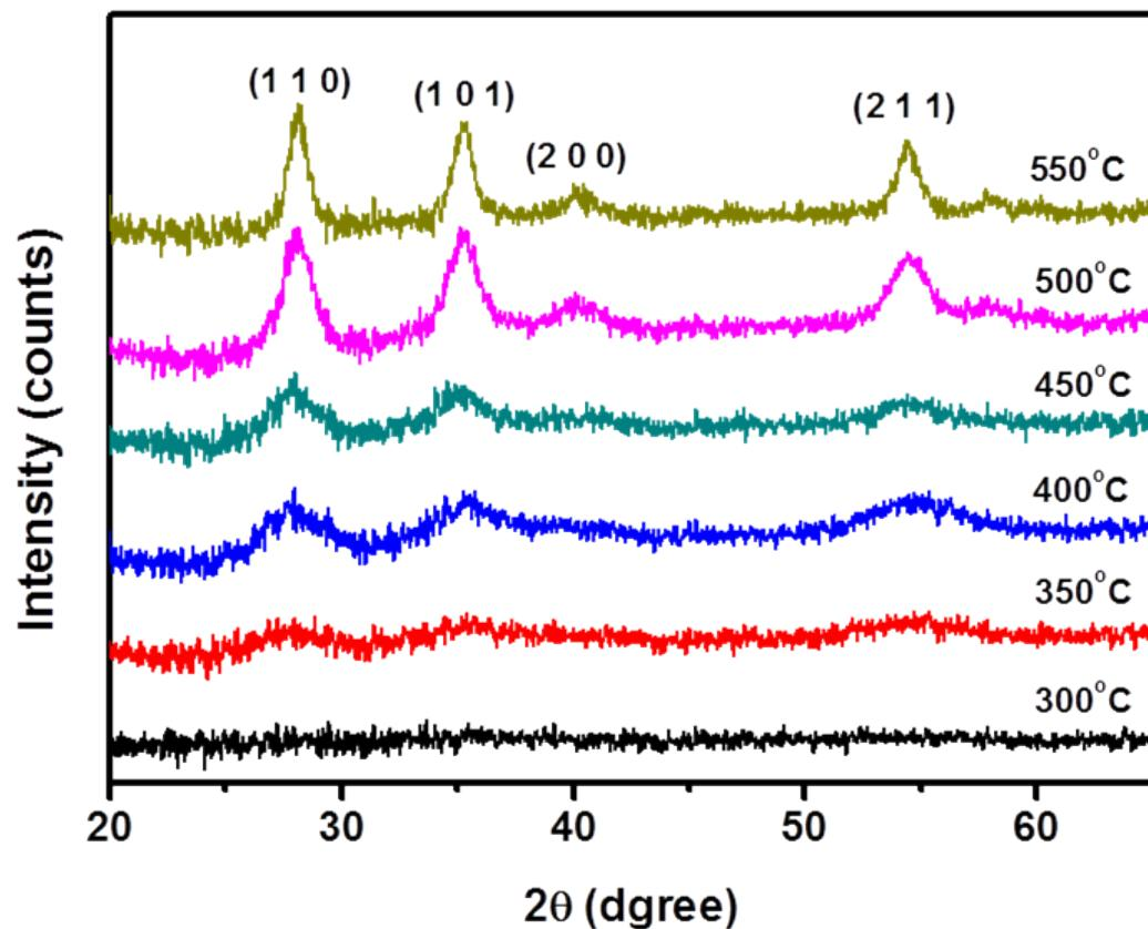
**Fig. S2** XRD patterns of the  $\text{RuO}_2\text{-ReO}_3$  composite nanofibers as a function of annealing temperature in air for electrospun  $\text{RuO}_2\text{-ReO}_3$  (precursor solution ratio,  $\text{Ru:Re}=2:1$ ) nanofibers at room temperature.
