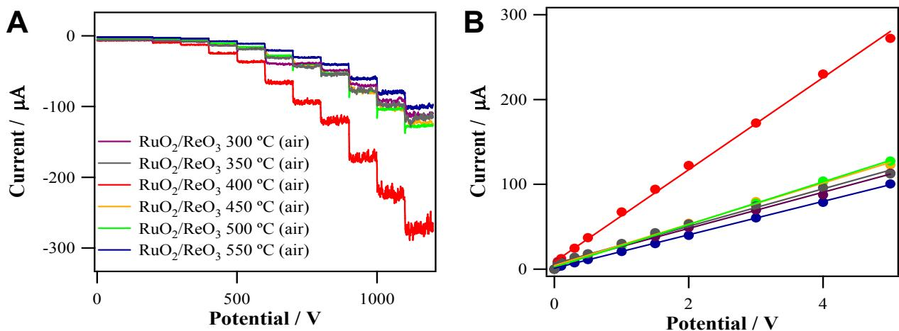
**Fig. S9.** (A) Dynamic current responses of various electrodes to the addition of H<sub>2</sub>O<sub>2</sub> in 0.10 M PBS at E<sub>app</sub> = - 0.2 V vs. SCE. (B) Corresponding calibration plots of (A) at various annealing temperatures.; at 300°C (purple), 350°C (black), 400°C (Red), 450°C (yellow), 500°C (green), and 550°C (blue).
