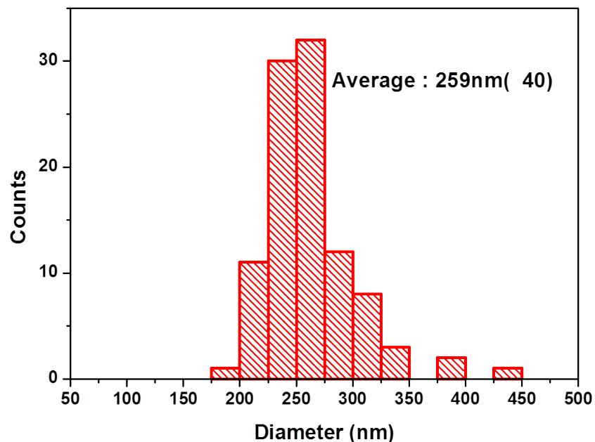
**Fig. S1** Histogram of the size distribution of the RuO<sub>2</sub>-ReO<sub>3</sub>(0.11) composite nanofibers after thermal annealing at 400°C in air.
