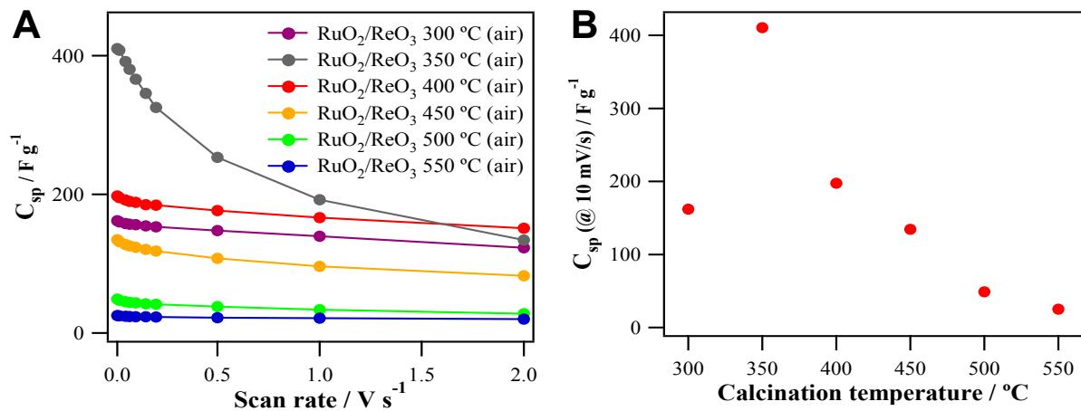
**Fig. S8.** (A) Variation of specific capacitance of RuO<sub>2</sub>-ReO<sub>3</sub>(n)/GC electrodes obtained by applying a potential from 0.1 to 0.9 V (vs. SCE) in 1.0 M H<sub>2</sub>SO<sub>4</sub> solution with  $v$  from 10 to 2000 mV s<sup>-1</sup> at various annealing temperatures. (B) The specific capacitance of RuO<sub>2</sub>-ReO<sub>3</sub>(n)/GC electrodes with 10 mV s<sup>-1</sup> at various annealing temperatures.
