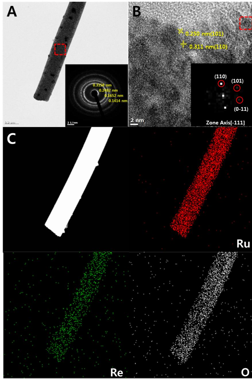
**Fig. S4.** Detailed crystal structures of  $\text{RuO}_2\text{-ReO}_3$  composite nanofibers by TEM; HRTEM image of  $\text{RuO}_2\text{-ReO}_3$  nanofibers and the fast Fourier transform (FFT) of the lattice-resolved image
