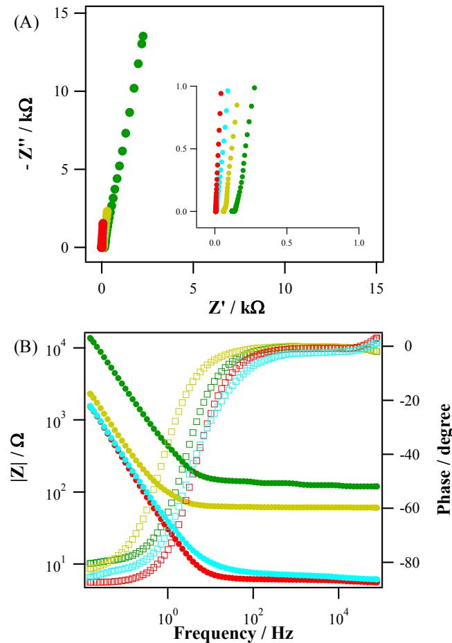
**Fig. S5.** (A) Nyquist plots and (B) Bode plots of various composite RuO<sub>2</sub>-ReO<sub>3</sub>(0.00, 0.07, 0.11, and 0.13)/GC electrodes in 1.0 M H<sub>2</sub>SO<sub>4</sub> solution ( $E_{\text{app}} = 0.50$  V, frequency range: from 10 mHz to 500 kHz); GC (black), RuO<sub>2</sub>/GC (green), RuO<sub>2</sub>-ReO<sub>3</sub>(0.07)/GC (yellow), RuO<sub>2</sub>-ReO<sub>3</sub>(0.11)/GC (red), and RuO<sub>2</sub>-ReO<sub>3</sub>(0.13)/GC (cyan).
