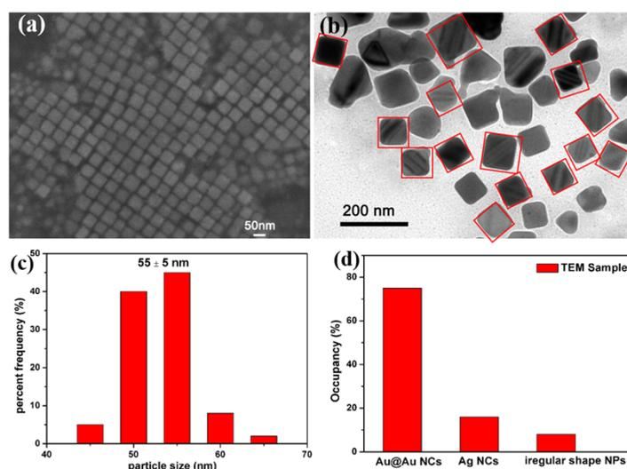
**Fig. S1** SEM image (a), TEM image (b), the size distribution histograms (c) and the occupancy (d) of the Au@Ag core-shell NCs
