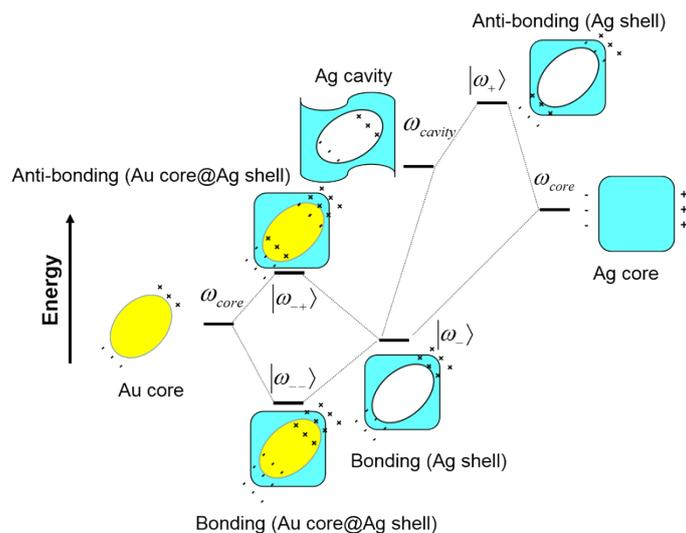
**Fig. S5** Plasmon hybridization diagram of Au@Ag core-shell NC structure
