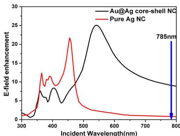
Fig. S4 The wavelength-dependent electric field enhancements of Au@Ag core-shell NC and pure Ag NC
