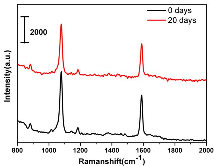
**Fig. S6** Raman spectra of 4-MBA labeled Au@Ag core-shell NCs solution at different days
