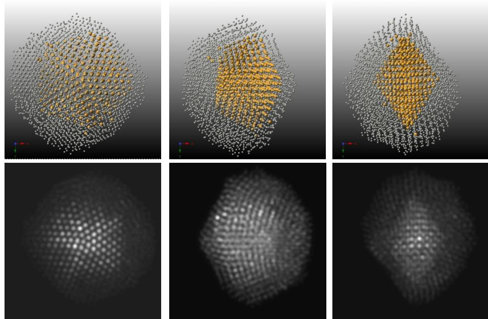
**Figure S7:** Simulated HAADF-STEM images of Dh Au(core)-Pd(shell) bimetallic nanoparticles at different orientations (left:0°, middle, 45° and right: 90°). Upper panel: configurations taken from gcMC, lower panel: HAADF-STEM simulations.
