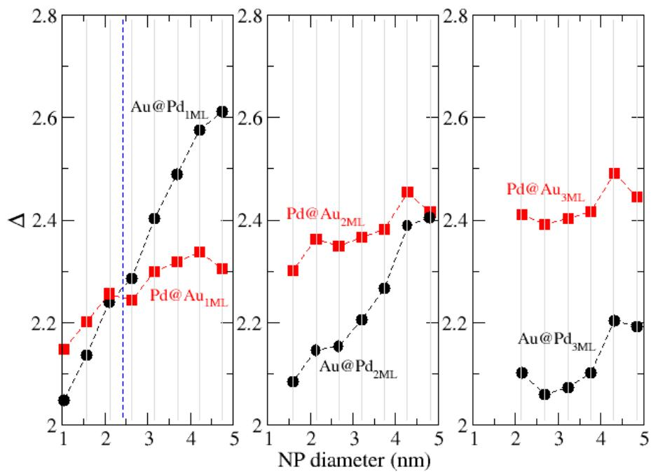
**Figure S4:** Excess energy as a function of NP size for core-shell with different shell-thickness (1 ML, 2 ML and 3 ML) for the case of Ih geometry
