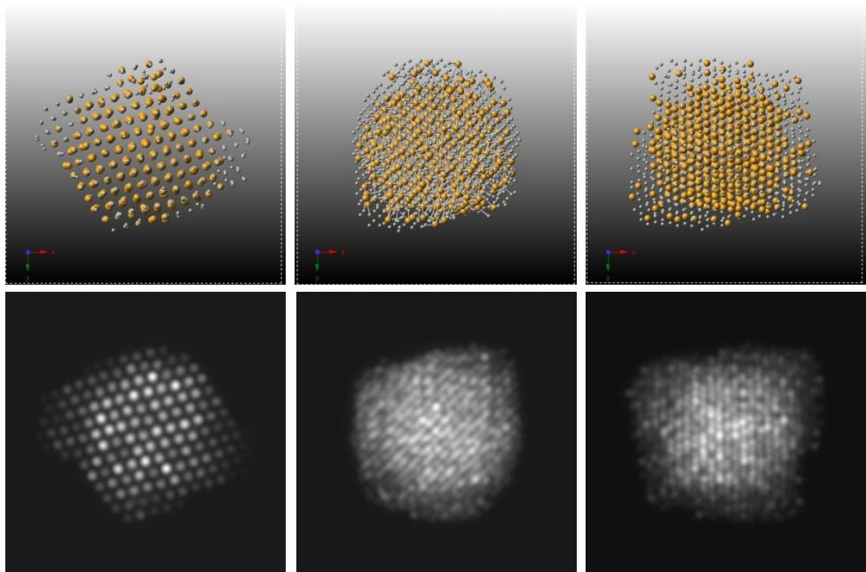
**Figure S8:** Simulated HAADF-STEM images of TOAu(core)-Pd(shell) bimetallic nanoparticles at different orientations (left:  $0^\circ$ , middle,  $45^\circ$  and right:  $90^\circ$ ). Upper panel: configurations taken from gCLD, lower panel: HAADF-STEM simulations.
