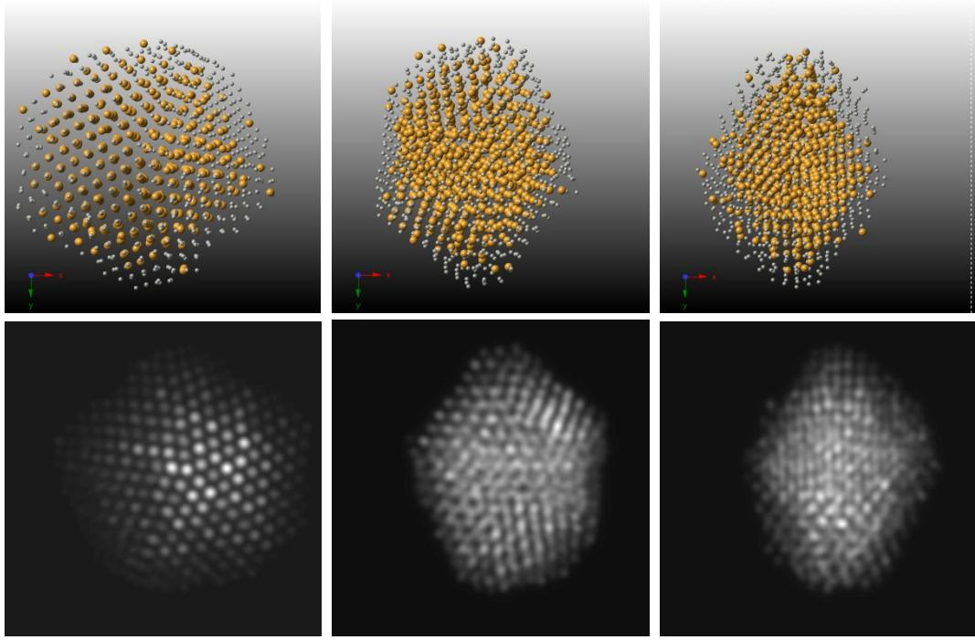
**Figure S6:** Simulated HAADF-STEM images of Dh Au(core)-Pd(shell) bimetallic nanoparticles at different orientations (left:0°, middle, 45° and right: 90°). Upper panel: configurations taken from gcLD, lower panel: HAADF-STEM simulations.
