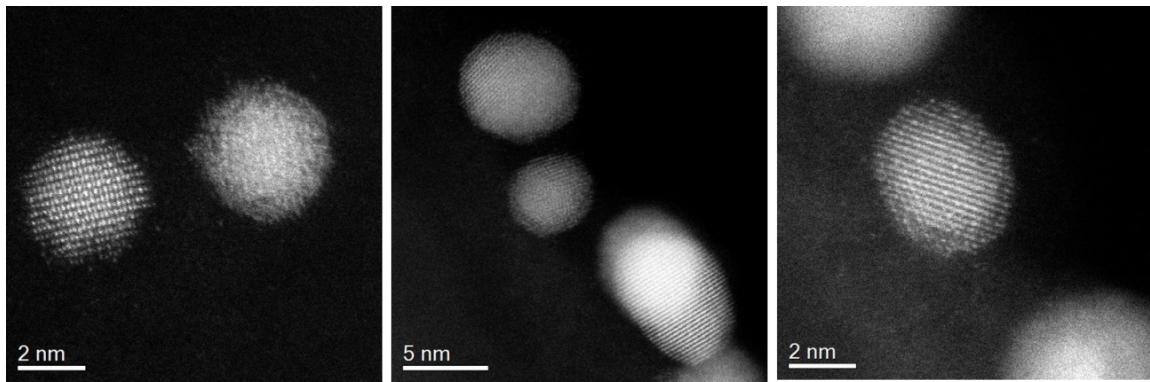
**Figure S2:** Diverse sub-5nm size core-shell NPs observed by Cs-STEM, in some of them, certain degree of mixing between Pd and Au is evident.
