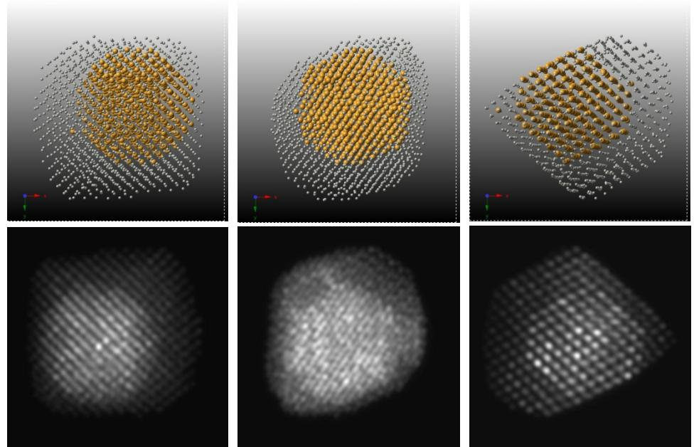
**Figure S9:** Simulated HAADF-STEM images of TO Au(core)-Pd(shell) bimetallic nanoparticles at different orientations (left:  $0^\circ$ , middle,  $45^\circ$  and right:  $90^\circ$ ). Upper panel: configurations taken from gcMC, lower panel: HAADF-STEM simulations
