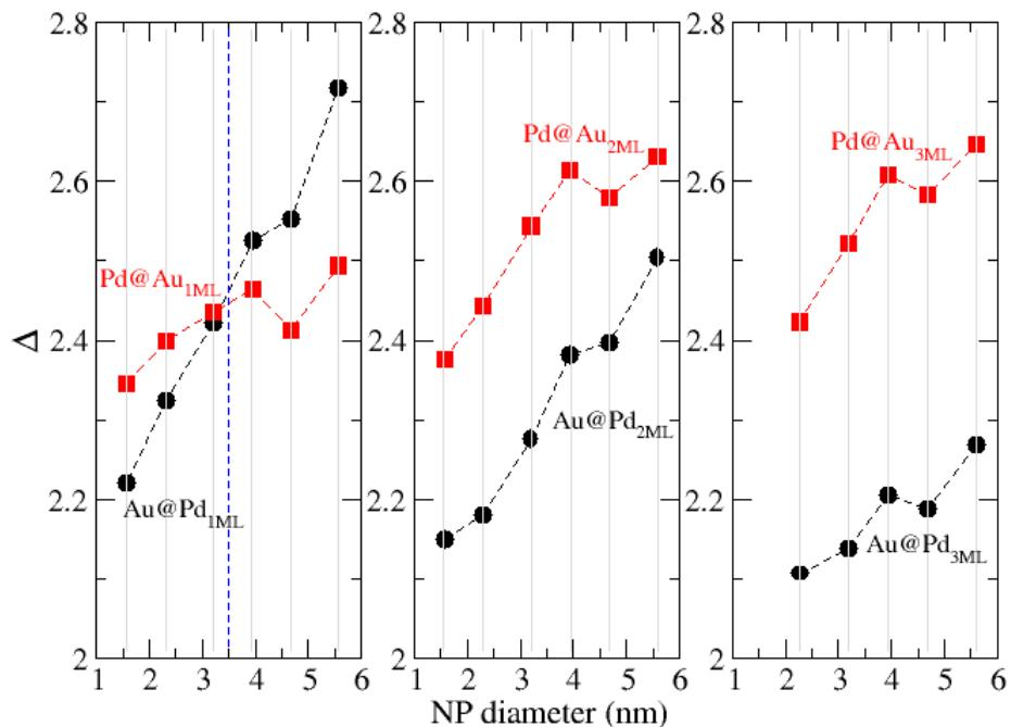
**Figure S3:** Excess energy as a function of NP size for core-shell with different shell-thickness (1 ML, 2 ML and 3 ML) for the case of Dh geometry.
