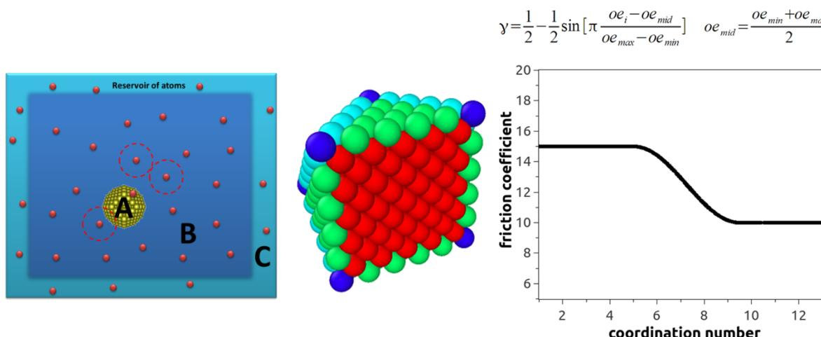
**Figure S1:** Left) GCLD model system: (A) cluster seed, (B) solution region and (C) reservoir of atoms. Right) cross-section of a typical nanoparticle where the atoms were colored according to its coordination number and dependence of the friction coefficient of each atom according to its coordination number.
