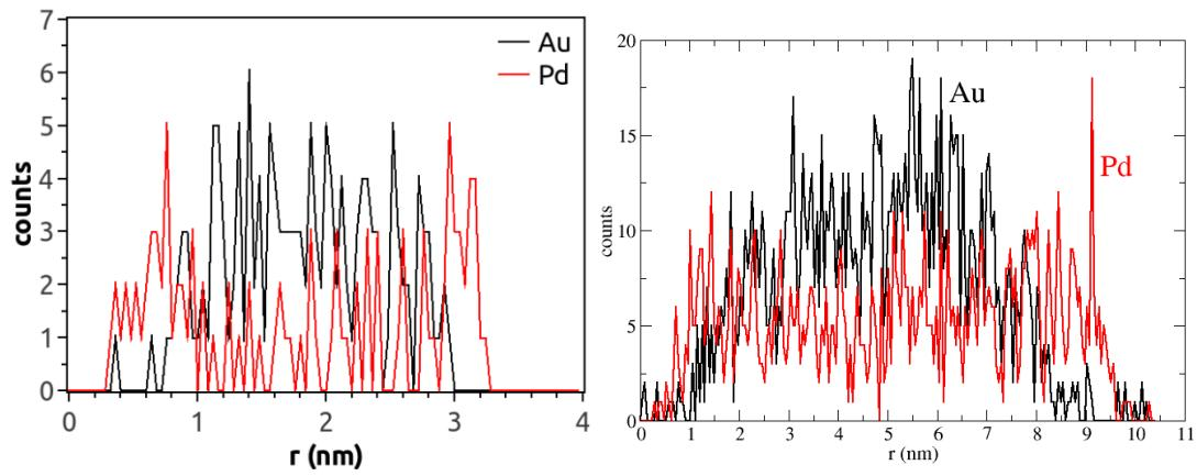
**Figure S10:** Left) Simulated EDS profile line of the resulting Dh Au(core)-Pd(shell) nanoparticles. Right) Experimental EDS profile line of a selected nanoparticle.
