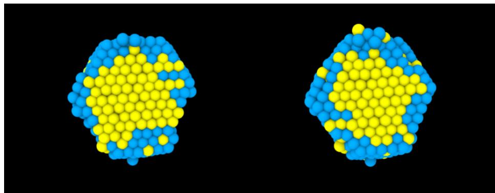
**Figure S5:** Cross-section images of figure 6f. Note the degree of mixing between Au and Pd in the interface region. Images produced with OVITO<sup>1</sup> software.
