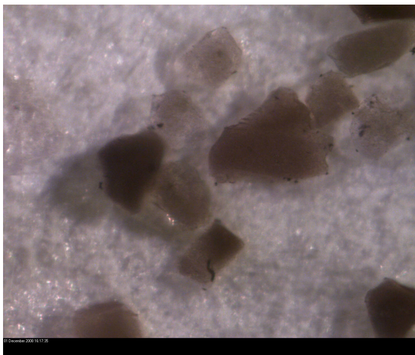
Fig. S2c. Visible microscope image of reduced 1:1 CuAu/SiO 2 .
