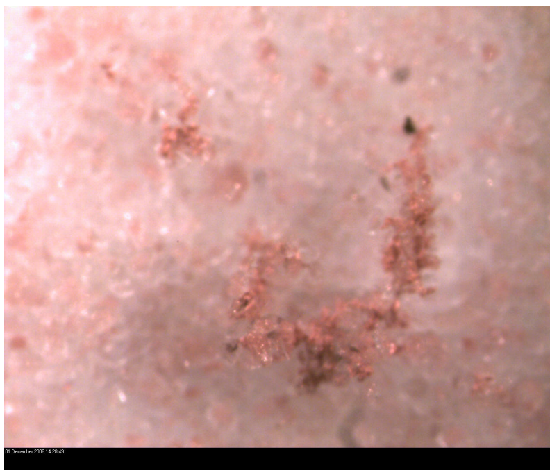
Fig. S2a Visible Microscope Image of 1:1 CuAu/SiO 2 catalyst direct calcination showing a large gold-rich cluster and pink copper-rich silica particles behind.
