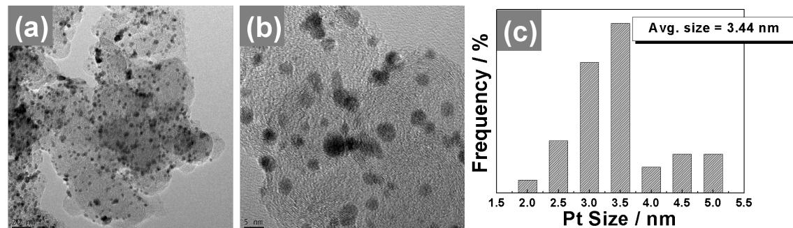
**Fig. S1** (a) TEM, (b) HR-TEM images, and (c) the size distribution of Pt/C before stability test.
