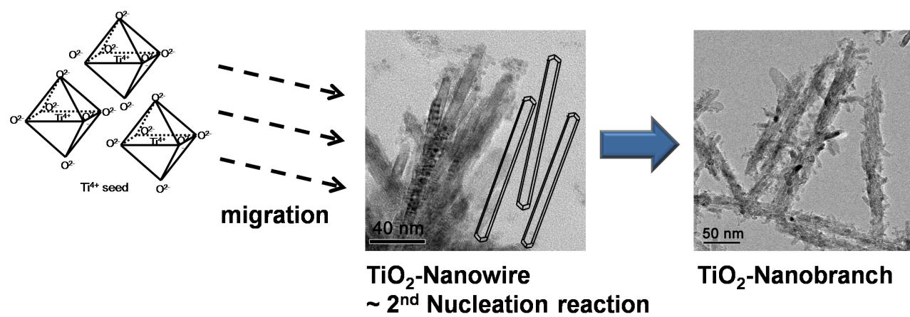
**Scheme S1** Formation mechanism of  $\text{TiO}_2$ -nanobranch supports using a seeding method with  $\text{TiO}_2$ -nanowires as seeds.
