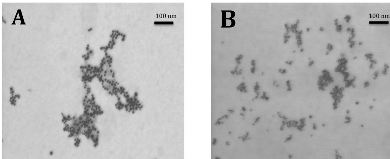
Figure S1. SEM pictures of AuNP before (A) and after (B) laser drop irradiation (1 s/d).
