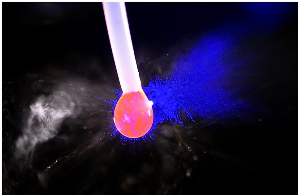
Figure S2. Picture of a drop of solution in the early stages of its explosion after one shot with the laser beam concentrated and focused in the drop.
