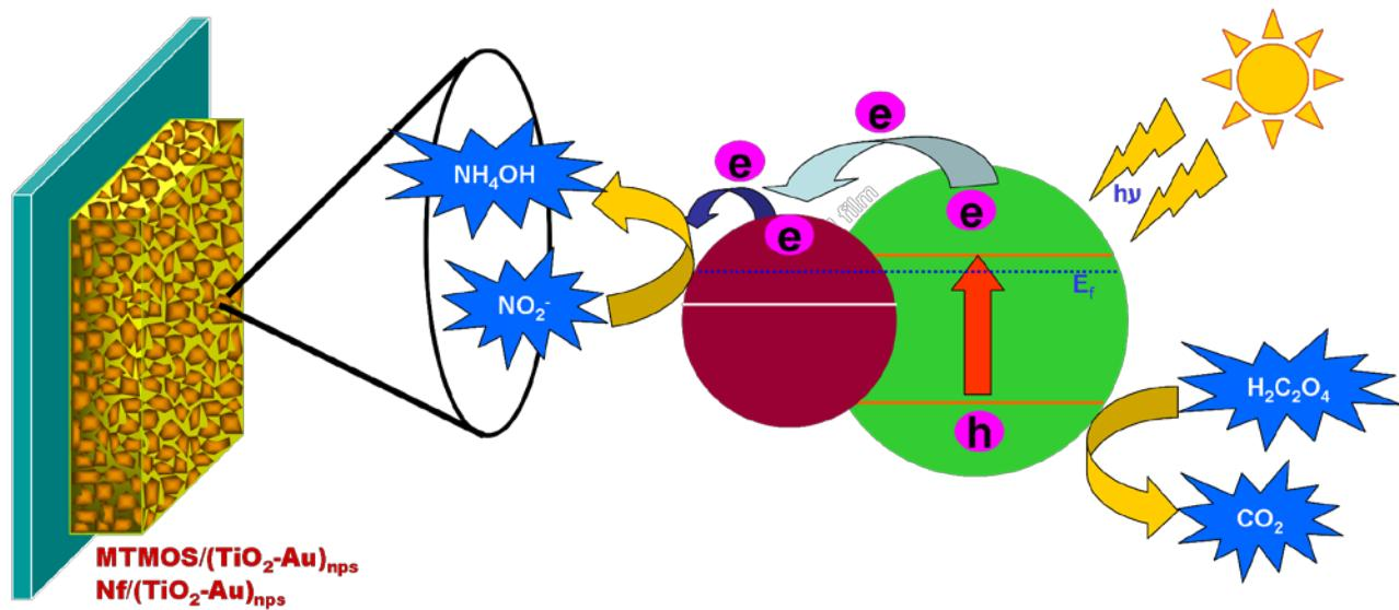
**Fig. S3.** Schematic representation for photocatalytic reduction of nitrite by  $(\text{TiO}_2-\text{Au})_{\text{nps}}$ .
