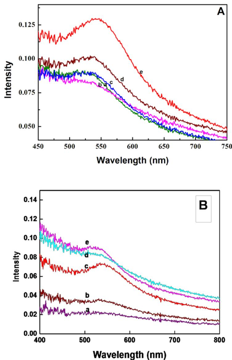
**Fig. S1.** Diffuse reflectance spectra of MTMOS/(TiO<sub>2</sub>-Au)<sub>nps</sub> (A) and Nf/(TiO<sub>2</sub>-Au)<sub>nps</sub> (B) film coated on glass plate. The molar ratios of TiO<sub>2</sub>:Au are: 100:1 (a), 100:2 (b), 100:3 (c), 100:4 (d) and 100:5 (e).
