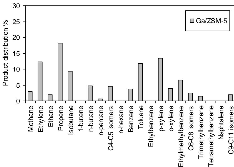
**Figure S2:** Product distribution for 1% wt Ga/ZSM-5 catalyst in the MTA reaction. (C<sub>9</sub>-C<sub>11</sub> isomers: aromatic products).
