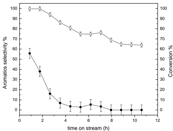
**Figure S7:** (●) conversion and (○) selectivity to aromatics in the reaction of methanol in a fully reduced 1% wt Ag/ZSM-5 catalyst pre-treated with H<sub>2</sub> for 4h at 550 °C.
