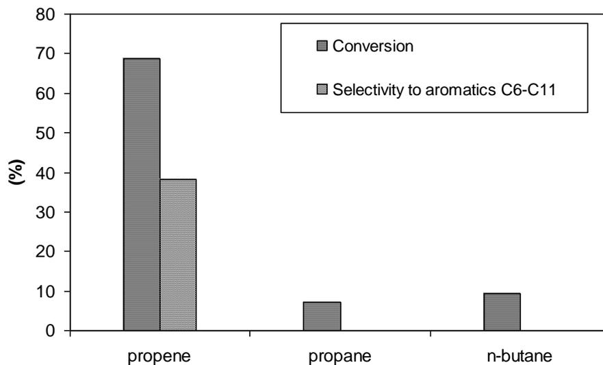
**Figure S8:** Conversion and selectivity to aromatics obtained feeding of ZSM-5 with propene, propane and *n*-butane.
