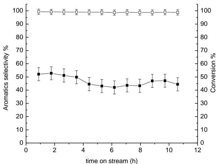
**Figure S1:** (■) conversion and (□) selectivity to aromatics in the reaction of methanol over 1% wt Ga/ZSM-5 catalyst.
