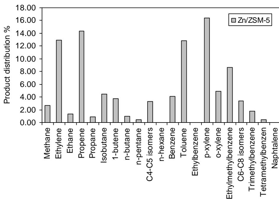
**Figure S4:** Product distribution for 1% wt Zn/ZSM-5 catalyst in the MTA reaction. (C<sub>9</sub>-C<sub>11</sub> isomers: aromatic products).
