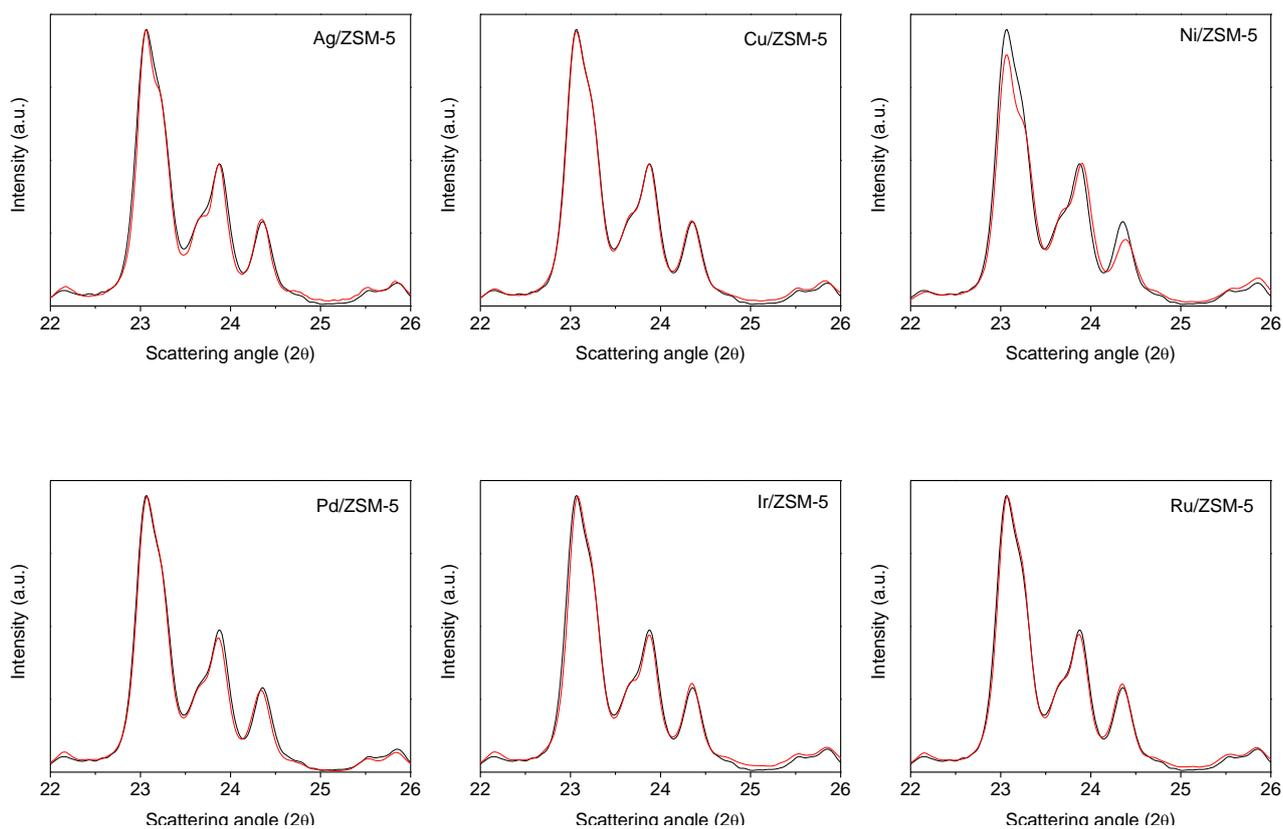
**Figure S5:** Enlarged  $2\theta$  region from 22 to  $26^\circ$  for the aluminium framework of Ag/ZSM-5, Cu/ZSM-5 and Ni/ZSM-5 (red line, top XRPD patterns) and Pd/ZSM-5, Ir/ZSM-5 and Ru/ZSM-5 (red line, bottom XRPD patterns). ZSM-5 (black line) is reported in all patterns for comparison.
