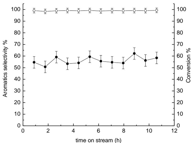
**Figure S3:** (●) conversion and (○) selectivity to aromatics in the reaction of methanol over 1% wt Zn/ZSM-5 catalyst.
