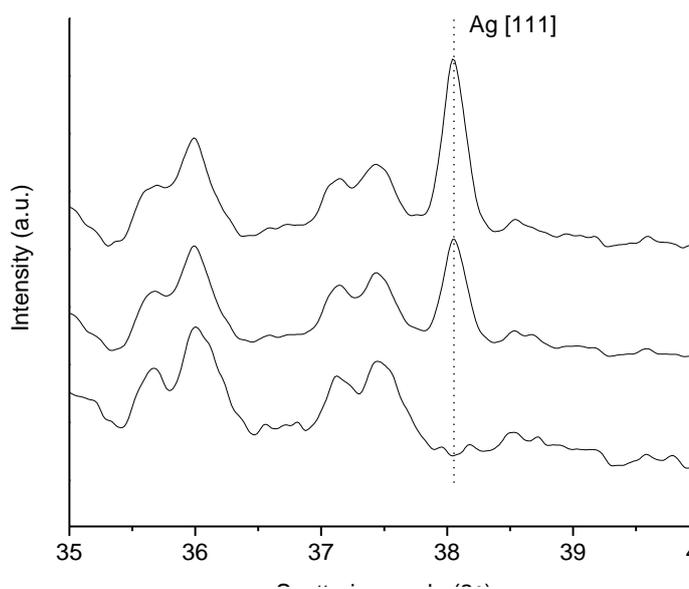
**Figure S6:** Reduction and formation of Ag metal in the MTA reaction (highlighted by the Ag[111] reflection) from a 1% wt Ag/ZSM-5 for: (a) fresh catalyst, (b) catalyst after 5.5 h time on stream and (c) catalyst after 11 h time on stream.
