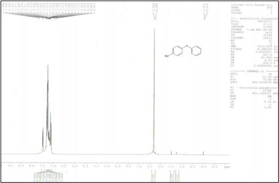
Figure 44. 1 H-NMR spectrum of 4-tolylphenyl sulfide (Table 2, Entry 3).
