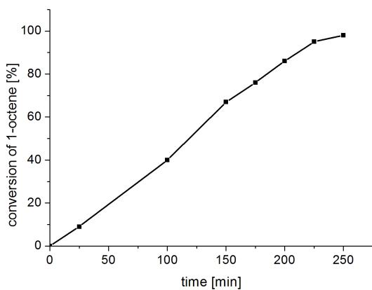
**Figure S3.** Hydrosilylation of 1-octene with 1,1,1,3,5,5-heptamethyltrisiloxane using Pt nanoparticle-loaded on a ROMP-derived monoliths.
