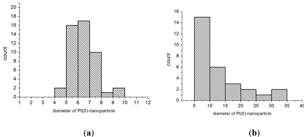
**Figure S6.** Histogram of Pt-nanoparticles immobilized on GMA-based monoliths **(a)** before catalysis; the mean particle diameter of the Pt nanoparticles was 6.4 nm. **(b)** After catalysis; the mean particle diameter of Pt nanoparticles was 12.6 nm.
