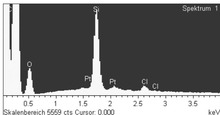
**Figure S2.** EDX spectrum of Pt-nanoparticles formed within the pores of a ROMP-derived monolith.
