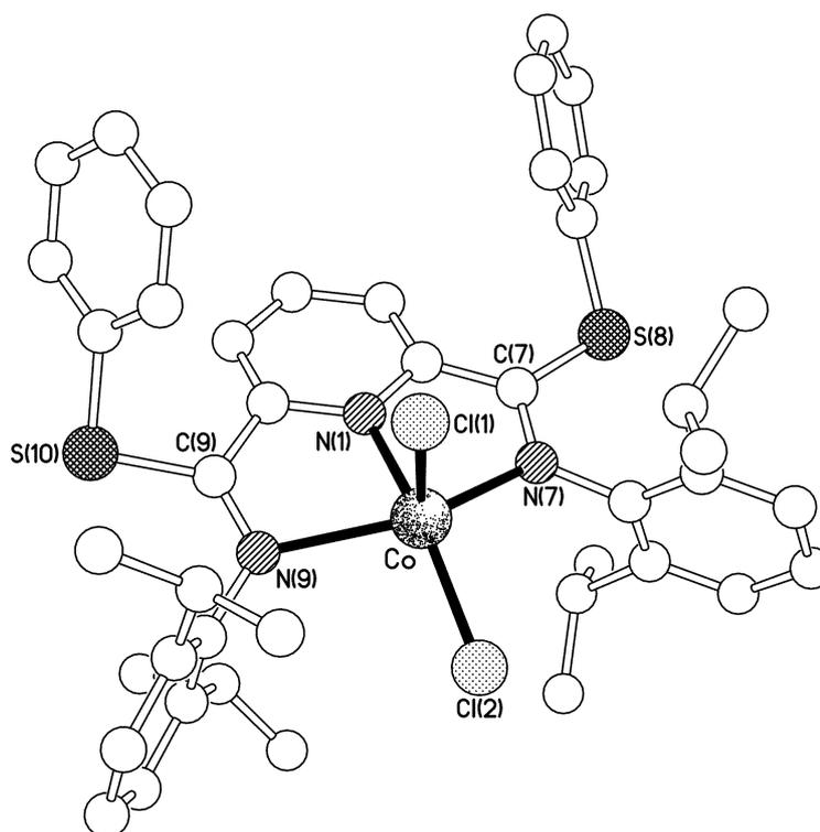
**Fig. S18** The molecular structure of [Co(6)Cl<sub>2</sub>].
