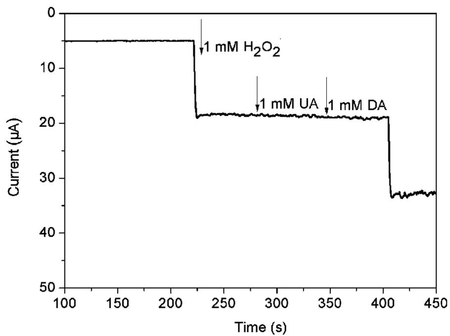
**Fig. S8** The current responses of AgNPs/PANINs/GCE to the sequential additions of 1.0 mM H<sub>2</sub>O<sub>2</sub>, 1.0 mM UA and 1.0 mM DA.
