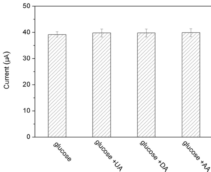
**Fig. S9** Comparison of the responses of GOD/AgNPs/PANINFs/GCE to the addition of 2 mM glucose, 2 mM glucose with 0.1 mM ascorbic acid (UA), 2 mM glucose with 0.1 mM uric acid (DA), and 2 mM glucose with 0.1 mM dopamine (UA) in O<sub>2</sub>-saturated 0.2 M PBS (pH 7.4) at -0.58 V.
