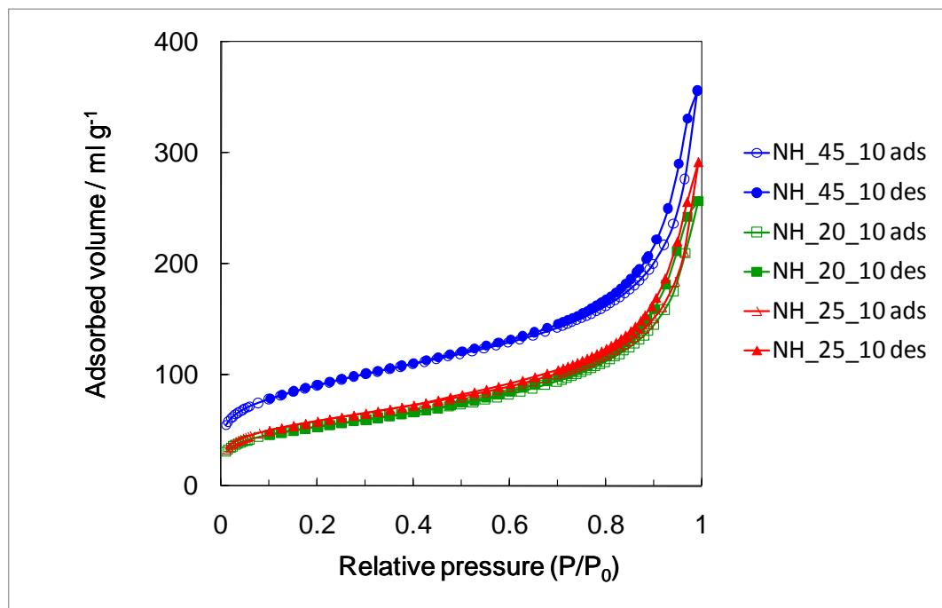
**Figure S3.** N<sub>2</sub> adsorption and desorption isotherms for NH\_Y\_10 catalysts that are not sketched in Fig. 1. When the alumina content is between 15 and 45 wt. %, the texture is very similar.
