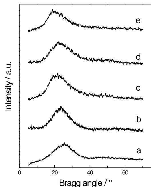
**Figure S4.** XRD diffractograms of (a) NH\_0\_10, (b) NH\_5\_10a, (c) NH\_10\_10, (d) NH\_15\_10 and (e) NH\_20\_10. The other samples present similar patterns (see also Debecker et al. Chem Mater 2009).
