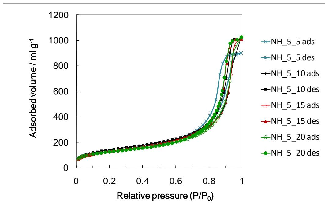
**Figure S2.** N<sub>2</sub> adsorption and desorption isotherms for catalysts with different MoO<sub>3</sub> content. The MoO<sub>3</sub> loading (between 5 and 20 wt. %) does not affect significantly the texture.
