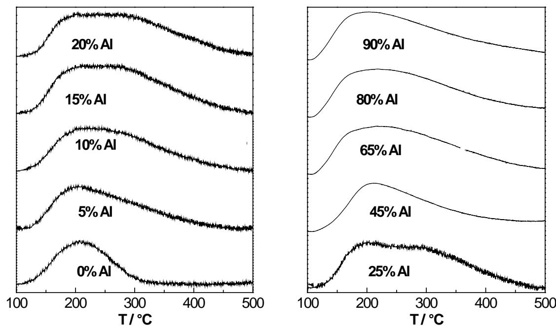
**Figure S5.** NH<sub>3</sub>-TPD thermograms obtained from the different catalysts with different Al content.
