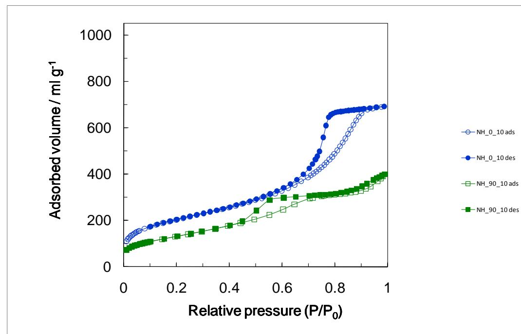
**Figure S1.** N<sub>2</sub> adsorption and desorption isotherms for binary catalysts (NH\_0\_10 and NH\_90\_10). Both samples are mesoporous.
