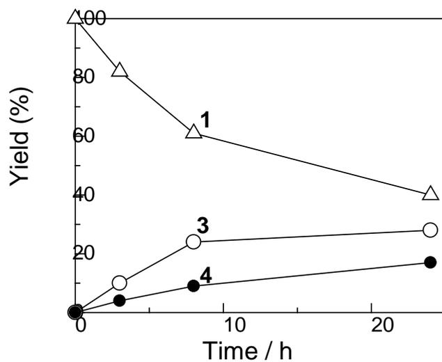
**Fig. S3.** Yields of (△) unreacted aniline **1**, (○) *N*-isopropylaniline **3** and (●) isopropylidene-phenylamine **4** for the reaction of aniline with *i*Pr<sub>2</sub>NH by Pt/CeO<sub>2</sub>-1.8 vs. reaction time. Reaction conditions are shown in Table 3.
