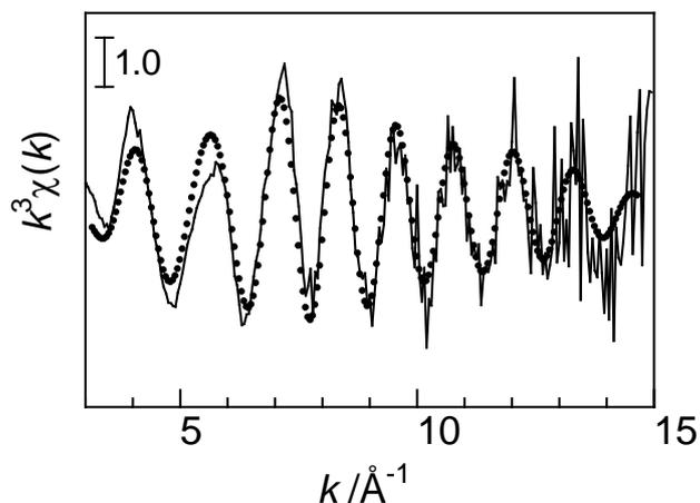
**Fig. S2.** The inverse Fourier transform of  $k^3$ -weighted Pt L3-edge EXAFS spectrum of (solid line) Pt/Al<sub>2</sub>O<sub>3</sub>-0.8 and (●) its best fit derived from curve-fitting analysis.
