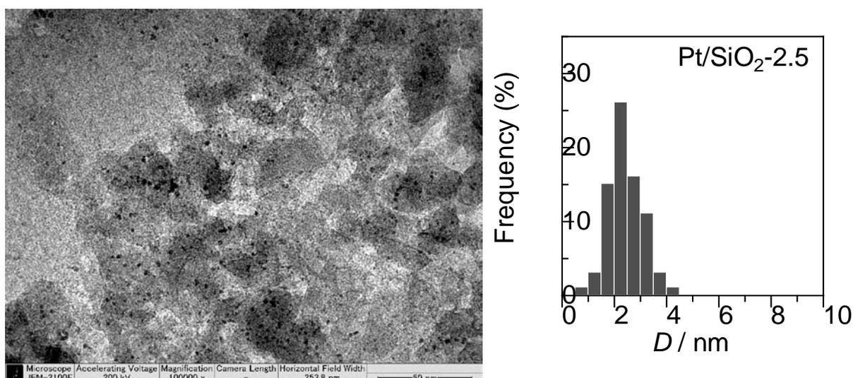
Fig. S1. TEM image and particle size distribution of Pt/SiO<sub>2</sub>-2.5.
