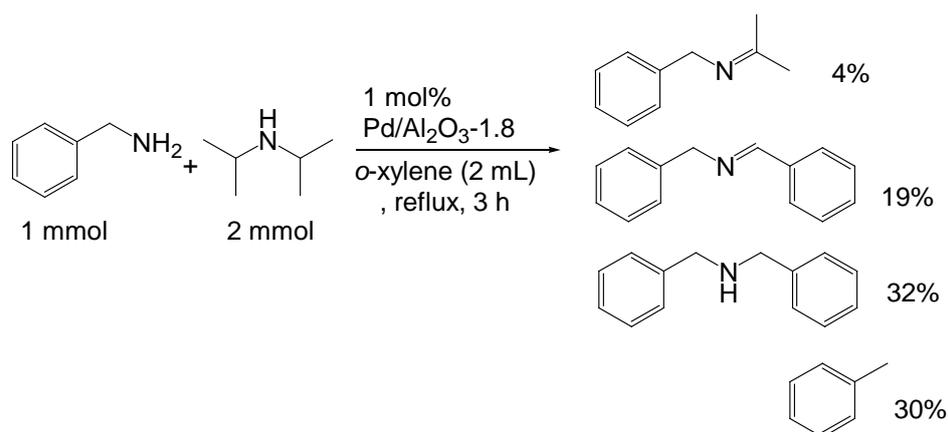
**Scheme S2.** N-alkylation of benzylamine with *i*Pr<sub>2</sub>NH by Pd/Al<sub>2</sub>O<sub>3</sub>-1.8.
