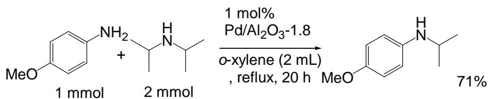
**Scheme S1.** N-alkylation of *p*-methoxyaniline with *i*Pr<sub>2</sub>NH by Pd/Al<sub>2</sub>O<sub>3</sub>-1.8.
