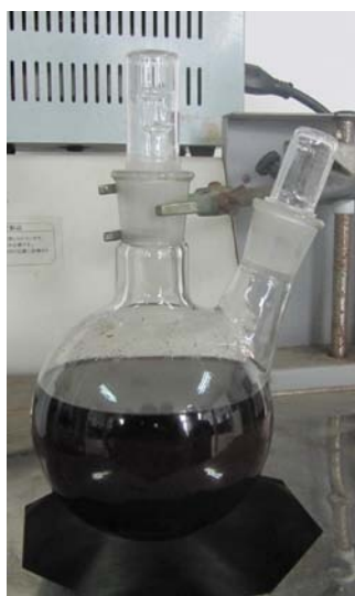
Fig. S5 Large-scale asymmetric epoxidation reaction of \alpha -methylstyrene (100 times as much as the experimental scale)
