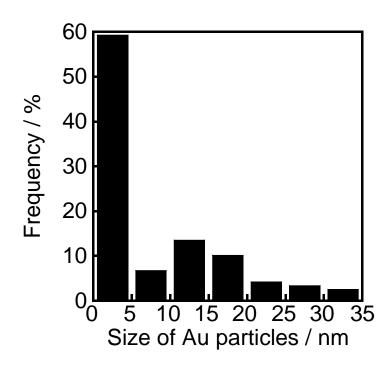
Figure S1 Particle size distribution of MS-(1.00)Au/TiO<sub>2</sub>.
